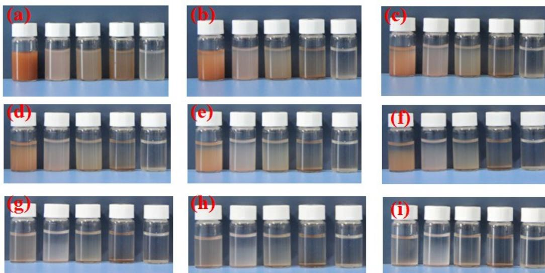
**Fig. S2** The detailed photographs for the dispersion stability of polymers in water ( $1.0 \text{ mg mL}^{-1}$ ) at  $25 \text{ }^\circ\text{C}$  after their ultrasonically dispersed solutions being settled down for 0 (a), 0.5 (b), 1.0 (c), 1.5 (d), 2.0 (e), 3.0 (f), 4.0 (g), 5.0 (h), and 6 h (i), respectively. The samples located from left to right in each photograph are MMIPs-2, MMIPs-5, MMIPs-8, MMIPs-11, and MMIPs-14.
