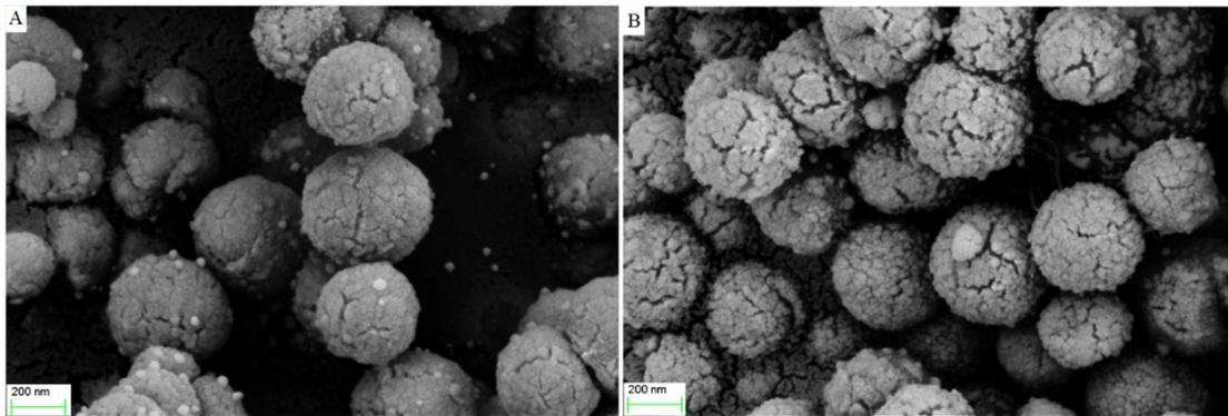
**Fig. S4.** SEM images of MMIPs-2 (A) and MMIPs-2 damaged at 100 °C for 12 h (B).
