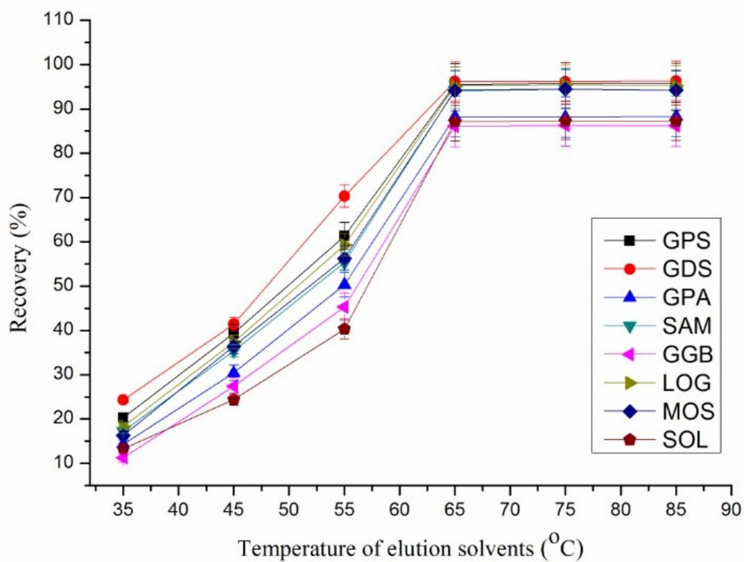
**Fig. S9** Effect of different elution solvents on IGs recoveries for MMIPs-2. Error bars represent one standard deviation for three measurements.
