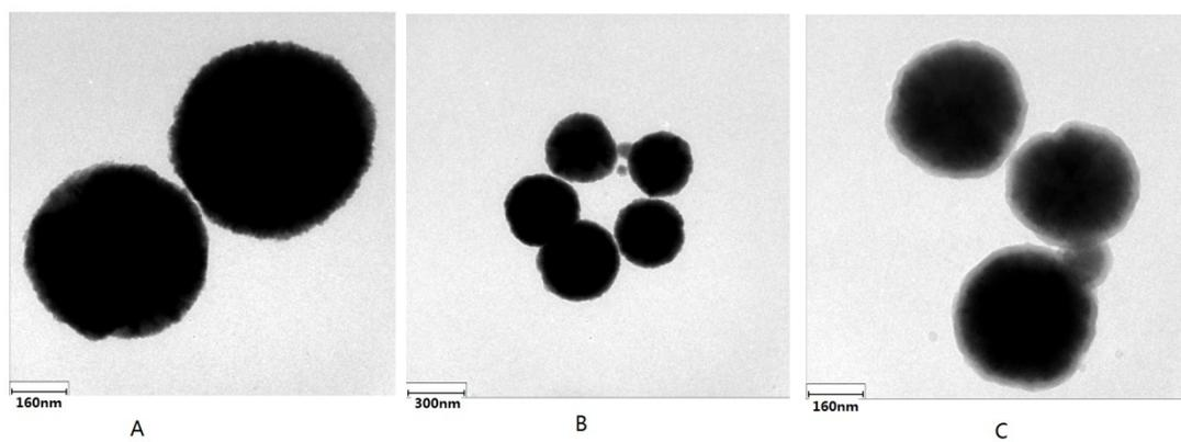
Fig. S1 The effect of the polymerization time on the shell thickness. (A) 3 h, (B) 6 h and (C) 9 h.
