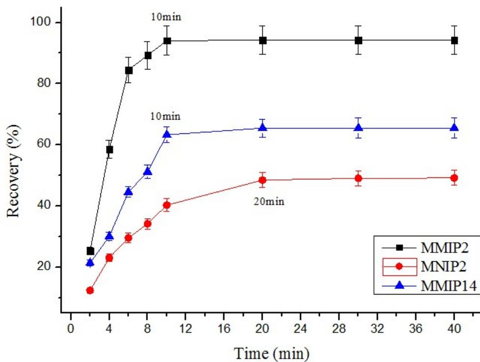
**Fig. S8** Extraction time on MMIPs-2, MNIPs-2, and MMIPs-14. Error bars represent one standard deviation for three measurements.
