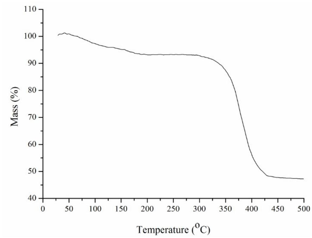
Fig. S5 The thermogravimetric analysis of MMIPs layer.
