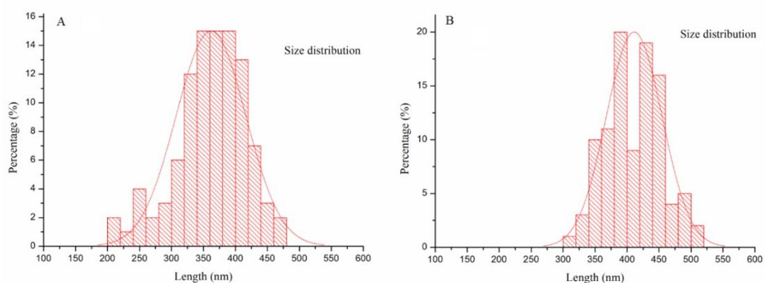
**Fig. S3.** Size distribution of Fe<sub>3</sub>O<sub>4</sub> (A) and MMIPs-2 (B). The particle diameter dispersity of polymers was calculated from the SEM data measuring the size of, at least, 100 particles.
