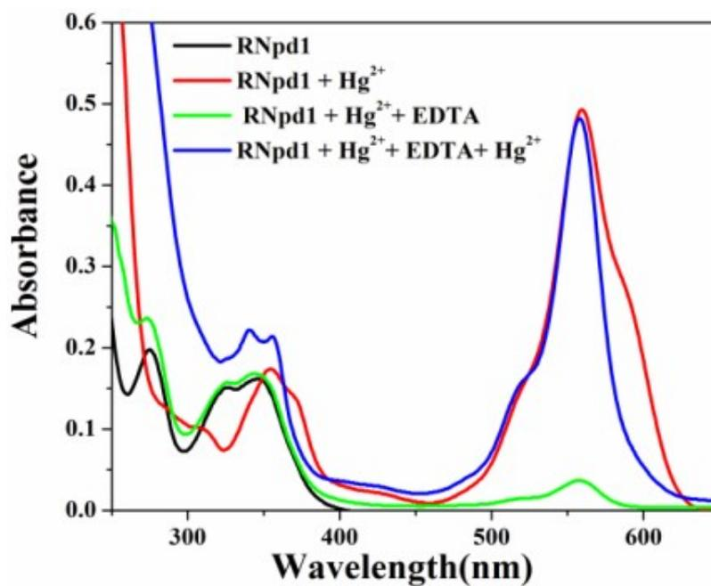
**Fig. S16** Reversibility of **RNpd1:Hg<sup>2+</sup>** complex with EDTA in pH 7.0 phosphate buffer/CH<sub>3</sub>OH (1:2, v/v).
