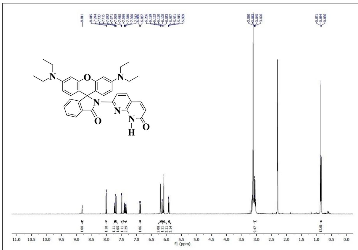
**<sup>1</sup>H-NMR spectrum of RNpd1:Hg<sup>2+</sup> in CDCl<sub>3</sub>**
