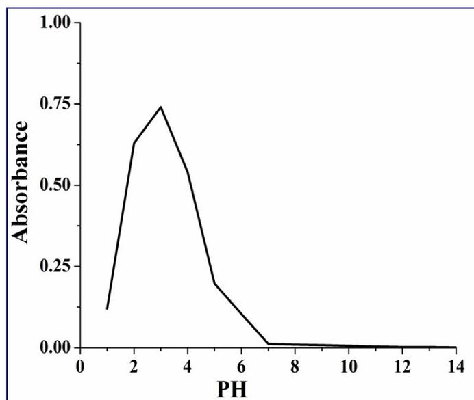
**Fig. S15** Influence of pH in absorbance of **RNpd1** (558 nm) in pH 7.0 phosphate buffer/CH<sub>3</sub>OH (1:2, v/v).
