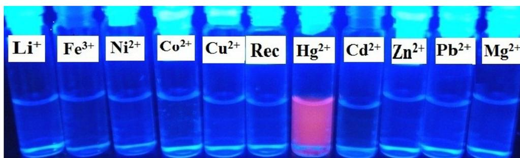
**Fig. S3** Visual fluorescence change under long wavelength UV light of **RNpd1** (10  $\mu$ M) with different metal ions ( $\text{Li}^+$ ,  $\text{Fe}^{3+}$ ,  $\text{Ni}^{2+}$ ,  $\text{Co}^{2+}$ ,  $\text{Cu}^{2+}$ ,  $\text{Rec}$ ,  $\text{Hg}^{2+}$ ,  $\text{Cd}^{2+}$ ,  $\text{Zn}^{2+}$ ,  $\text{Pb}^{2+}$ ,  $\text{Mg}^{2+}$ ) in pH 7.0 phosphate buffer/ $\text{CH}_3\text{OH}$  (1:2, v/v).
