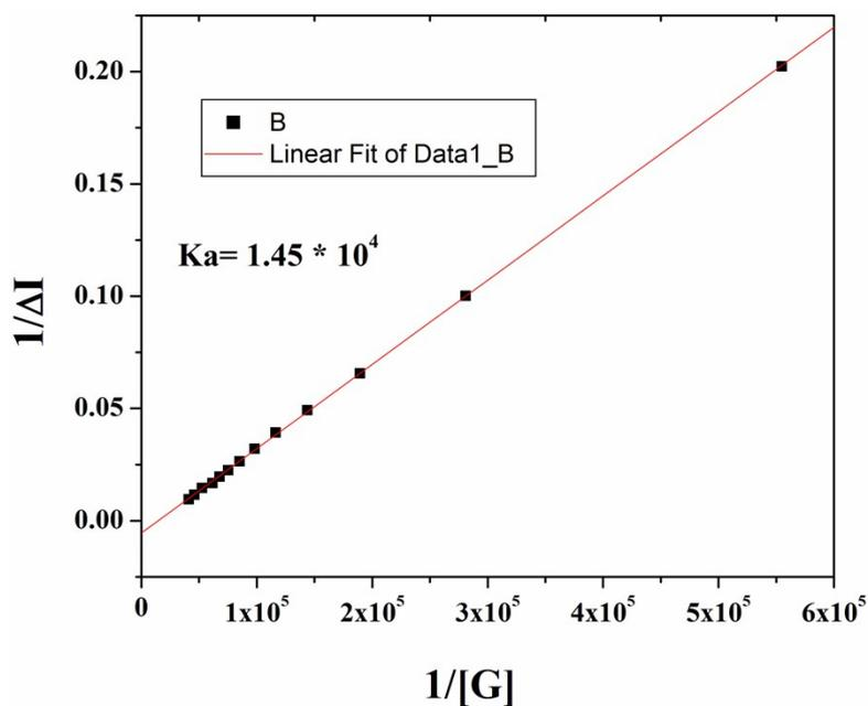
**Fig. S9** Binding constant calculation graph of **RNpd1** with **UA** using fluorescence titration.
