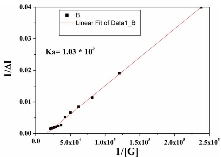
**Fig. S11** Binding constant calculation graph of RNpd1 with guanine using fluorescence titration.
