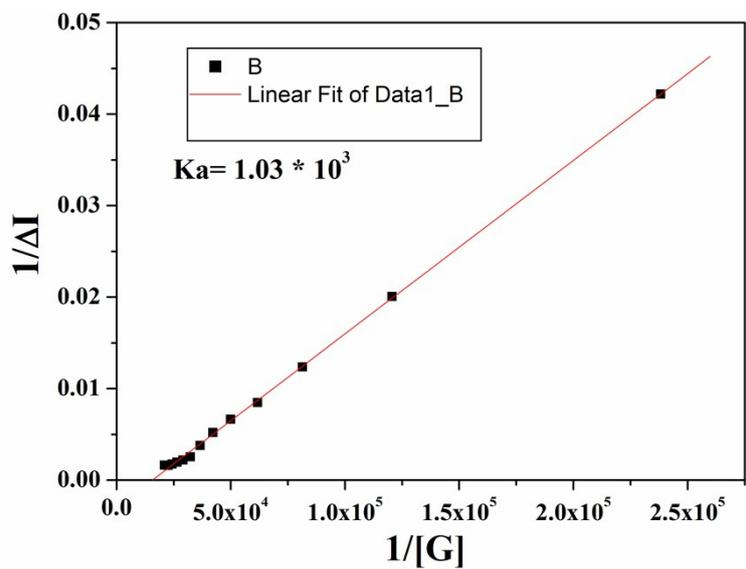
**Fig. S10** Binding constant calculation graph of RNpd1 with adenine using fluorescence titration.
