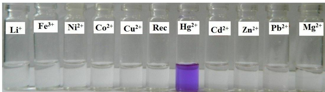
**Fig. S2** Visual colour change of **RNpd1** (10  $\mu$ M) with different metal ions ( $\text{Li}^+$ ,  $\text{Fe}^{3+}$ ,  $\text{Ni}^{2+}$ ,  $\text{Co}^{2+}$ ,  $\text{Cu}^{2+}$ ,  $\text{Hg}^{2+}$ ,  $\text{Cd}^{2+}$ ,  $\text{Zn}^{2+}$ ,  $\text{Pb}^{2+}$ ,  $\text{Mg}^{2+}$ ) in pH 7.0 phosphate buffer/ $\text{CH}_3\text{OH}$  (1:2, v/v).
