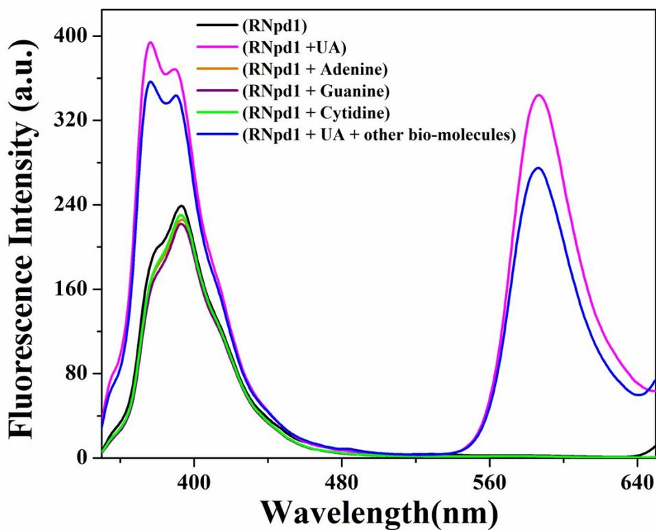
**Fig. S13** Competitive Fluorescence spectra of RNpd1 with UA and other biomolecules in pH 7.0 phosphate buffer/CH<sub>3</sub>OH (1:2, v/v).
