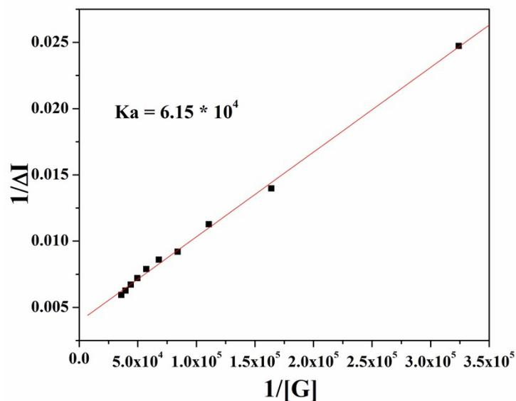
**Fig. S8** Binding constant calculation graph of **RNpd1** with **Hg<sup>2+</sup>** using fluorescence titration.
