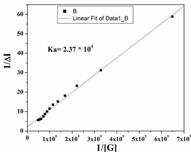
**Fig. S4** Binding constant calculation graph of **RNpd1** with **Hg<sup>2+</sup>** using UV-vis titration.
