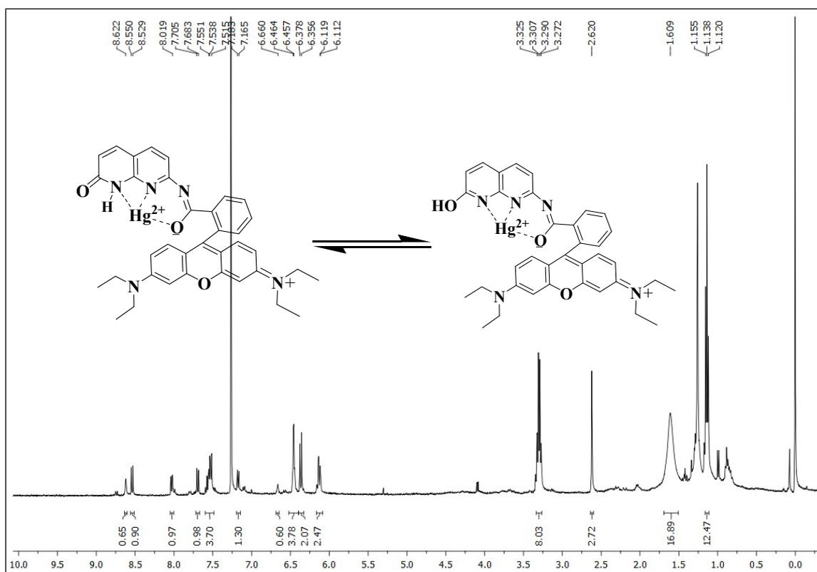
**$^1\text{H-NMR}$  spectrum of  $\text{RNpd1:Hg}^{2+}$  in  $\text{CDCl}_3$  (Expansion) (Keto-enol tautomerism)**
