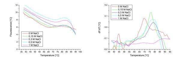
S2. Experiments researching stability of BSA in solution with different concentrations of NaCl conducted on the Roche Light Cycler, capillary based. The left graph shows the captured fluorescence as a function of temperature, while the right displays the first derivative of fluorescence with respect to temperature. For excitation the Light Cycler uses an LED with a peak emission wavelength of 470nm, an emission filter with a bandpass of 710nm was used for capturing fluorescence. As
