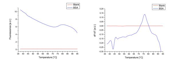
S1. Measurement of background fluorescence of hydrophobic dye bye done with light cycler (left) and first derivative of signal with respect to temperature (right). The sample containing only the dye and buffer, volumes were adjusted to 20µL using water (red). In the same run a sample containing BSA was tested (blue) as a comparison of typical signal intensities.
