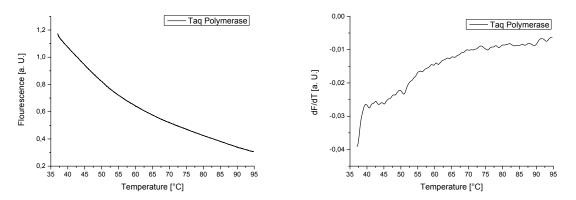
S3. Denaturation of Taq polymerase as recorded by the LightCycler. The signal is very low compared to measurements conducted with BSA. Furthermore the optical filters of the commercial device are not optimal for the dye used in the experiments. A decrease in fluorescence with increasing temperature can be observed as seen on chip. However, due to the low signal no denaturation of domains can be observed.
