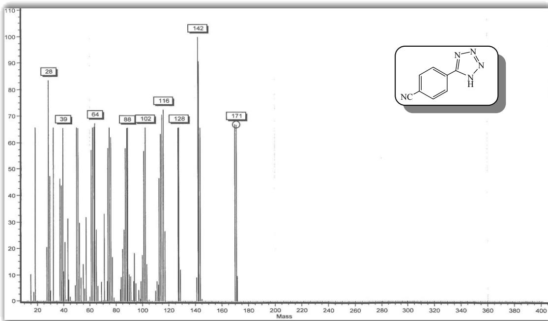
**Figure 18:** Mass spectrum of 4-(1*H*-tetrazol-5-yl)benzonitrile.
