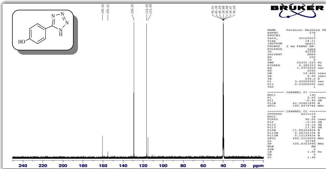
**Figure 33:**  $^{13}\text{C}$  NMR (100 MHz,  $\text{DMSO}-d_6$ ) of 4-(1*H*-tetrazol-5-yl) phenol.
