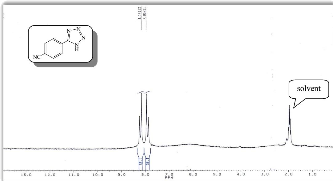
**Figure 15:** <sup>1</sup>H NMR (100 MHz, CD<sub>3</sub>CN) of 4-(1*H*-tetrazol-5-yl)benzonitrile.
