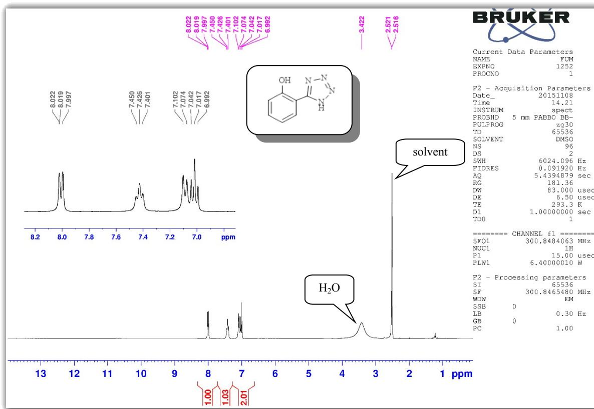
**Figure 35:** <sup>1</sup>H NMR (300 MHz, DMSO-*d*<sub>6</sub>) of 2-(1*H*-tetrazol-5-yl)phenol.
