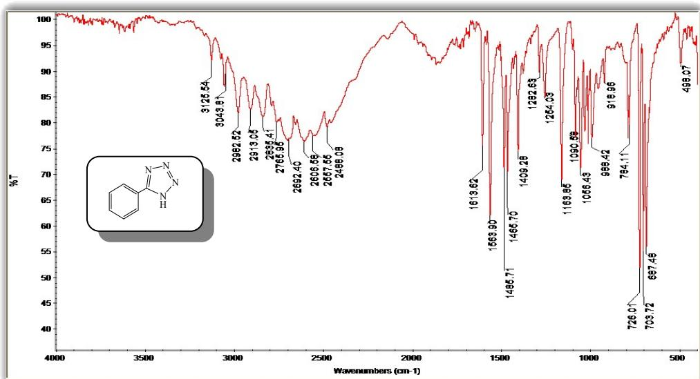
**Figure 1:** FT-IR (KBr) of 5-Phenyl-1*H*-tetrazole.
