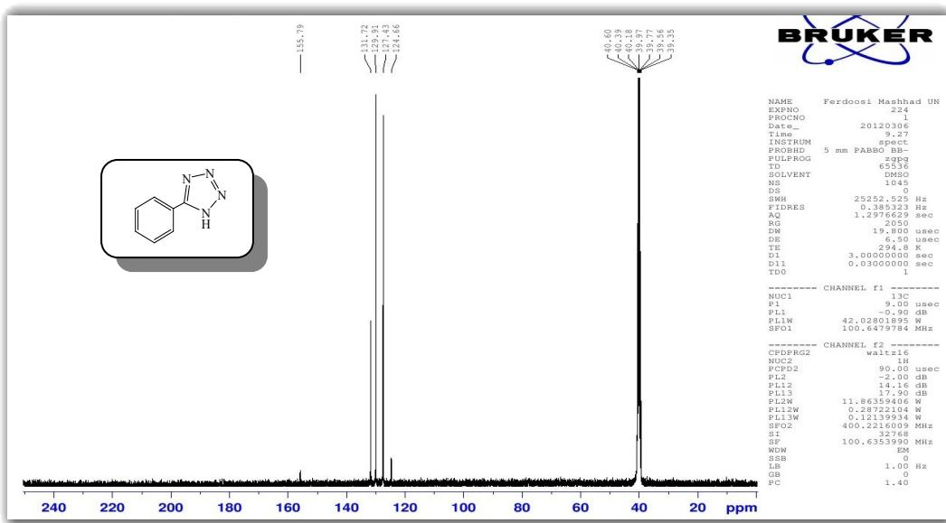
**Figure 3:**  $^{13}\text{C}$  NMR (100 MHz, DMSO- $d_6$ ) of 5-Phenyl-1*H*-tetrazole.
