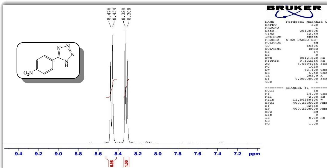
**Figure 12:**  $^1\text{H}$  NMR (400 MHz,  $\text{DMSO}-d_6$ ) of 5-(4-Nitrophenyl)-1*H*-tetrazole expanded.
