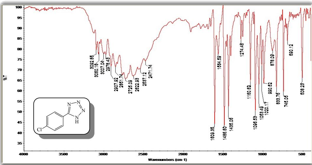
**Figure 10:** FT-IR (KBr) of 5-(4-Chlorophenyl)-1*H*-tetrazole.
