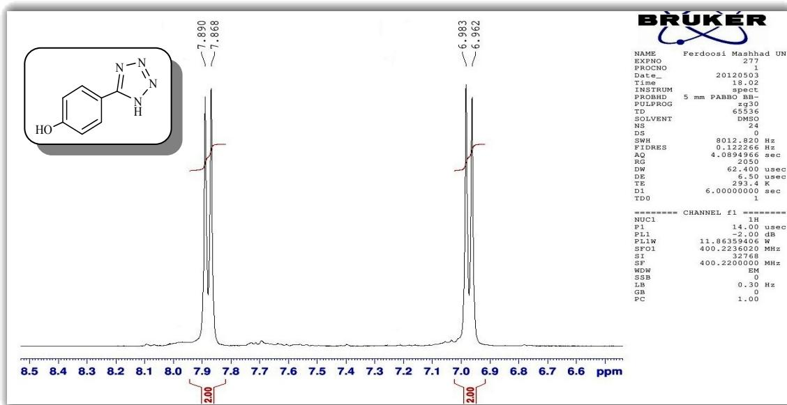
**Figure 32:**  $^1\text{H}$  NMR (400 MHz,  $\text{DMSO}-d_6$ ) of 4-(1*H*-tetrazol-5-yl)phenol expanded.
