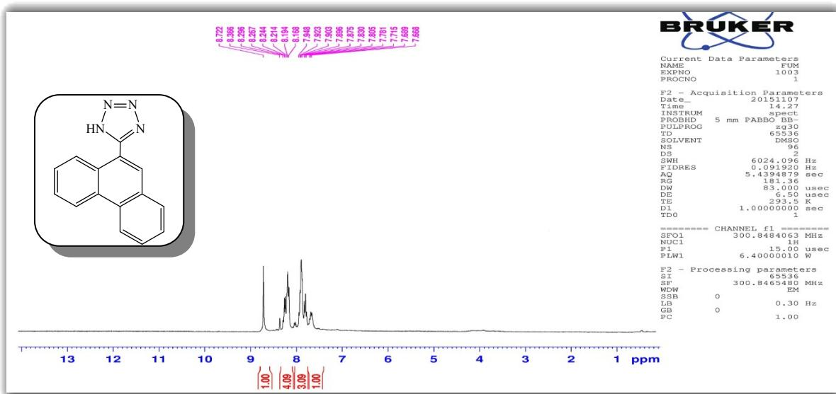
**Figure 43:**  $^1\text{H}$  NMR (300 MHz,  $\text{DMSO}-d_6$ ) of 5-(Phenanthren-9-yl)-1*H*-tetrazole.
