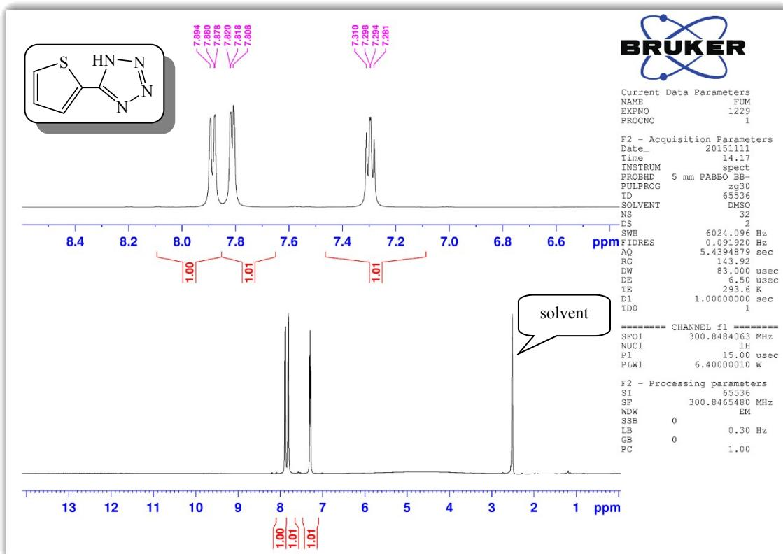
**Figure 53:** <sup>1</sup>H NMR (300 MHz, DMSO-*d*<sub>6</sub>) of 5-(Thiophen-2-yl)-1*H*-tetrazole (3p).
