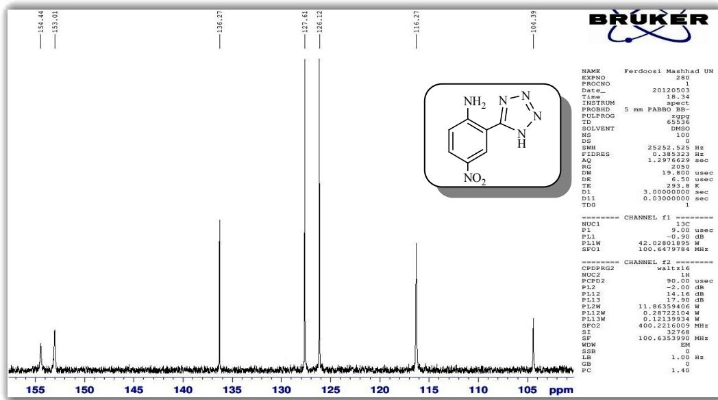
**Figure 22:**  $^{13}\text{C}$  NMR (100 MHz,  $\text{DMSO}-d_6$ ) of 4-Nitro-2-(1*H*-tetrazol-5-yl)benzenamine expanded.
