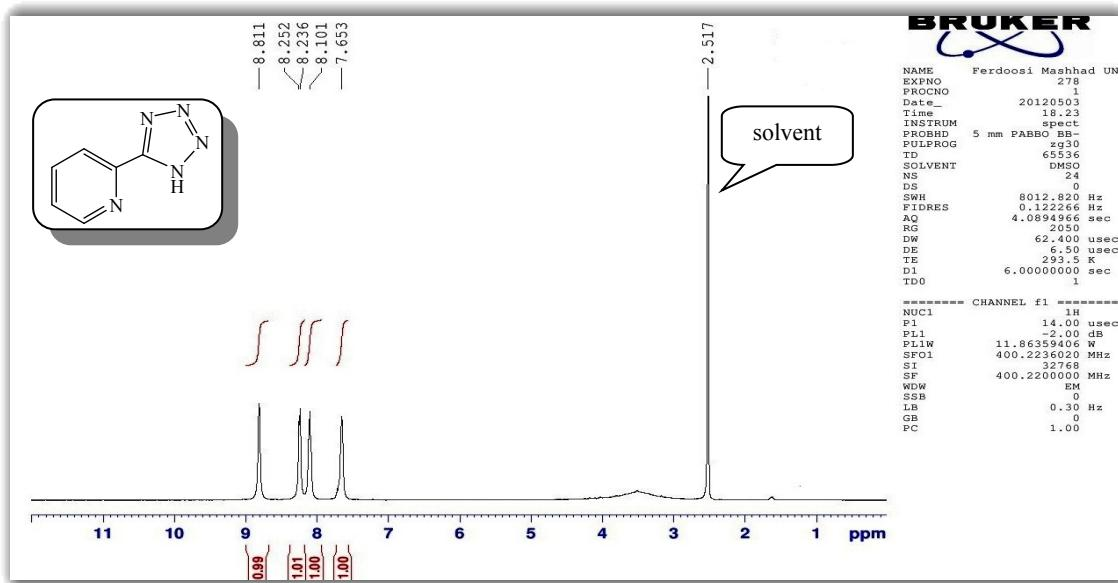
**Figure 50:** <sup>1</sup>H NMR (400 MHz, DMSO-*d*<sub>6</sub>) of 2-(1*H*-tetrazol-5-yl)pyridine.
