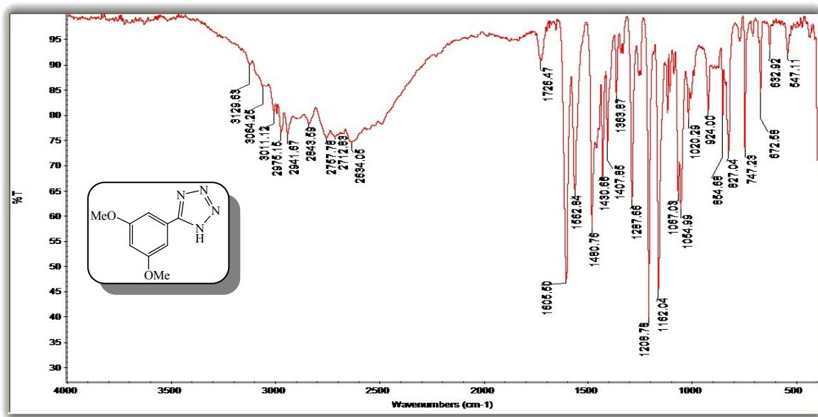
**Figure 26:** FT-IR (KBr) of 5-(3,5-Dimethoxyphenyl)-1*H*-tetrazole.
