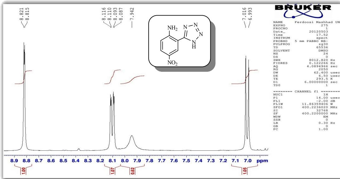
**Figure 20:**  $^1\text{H}$  NMR (400 MHz,  $\text{DMSO}-d_6$ ) of 4-Nitro-2-(1*H*-tetrazol-5-yl)benzenamine expanded.
