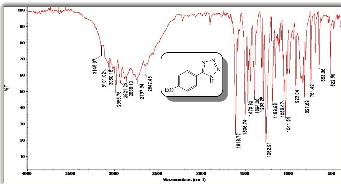
**Figure 42:** FT-IR (KBr) of 5-(4-Ethoxyphenyl)-1*H*-tetrazole.
