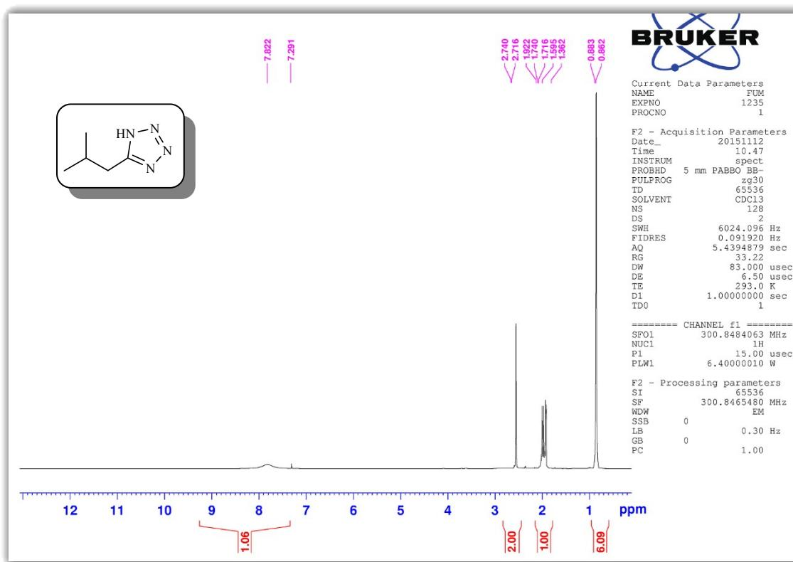
**Figure 61:**  $^1\text{H}$  NMR (300 MHz,  $\text{CDCl}_3$ ) of 5-Isobutyl-1*H*-tetrazole.
