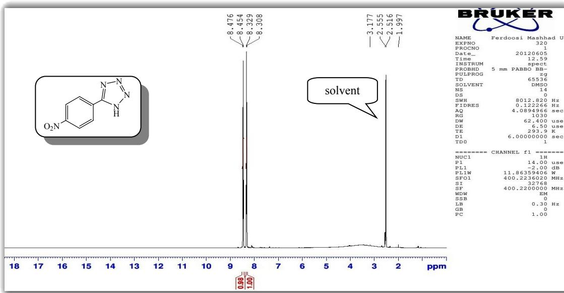
Figure 11: <sup>1</sup>H NMR (400 MHz, DMSO-*d*<sub>6</sub>) of 5-(4-Nitrophenyl)-1*H*-tetrazole.
