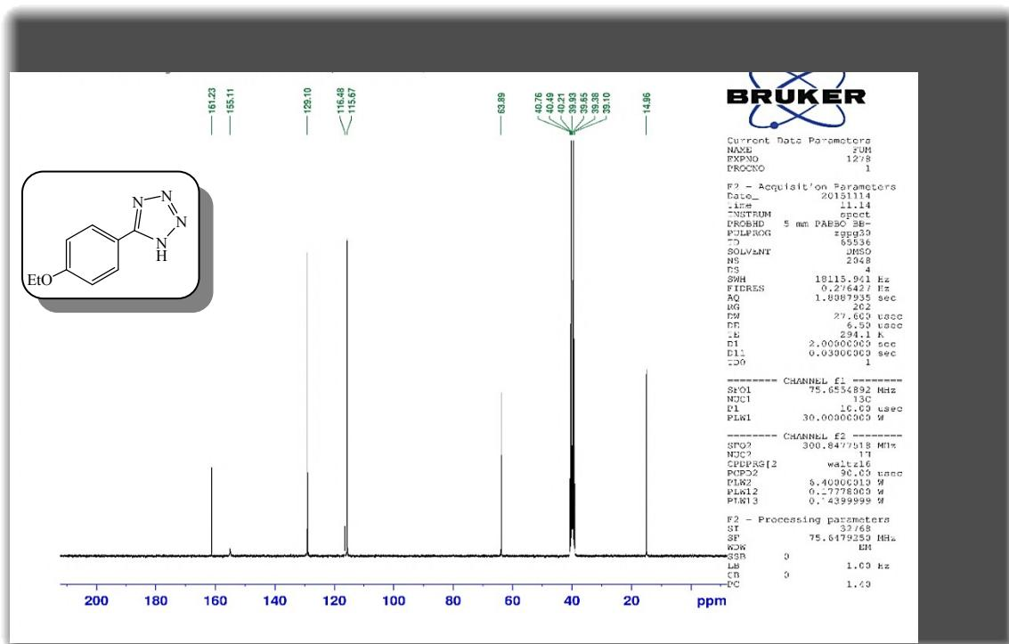
**Figure 41:**  $^{13}\text{C}$  NMR (75 MHz,  $\text{DMSO}-d_6$ ) of 5-(4-Ethoxyphenyl)-1*H*-tetrazole.
