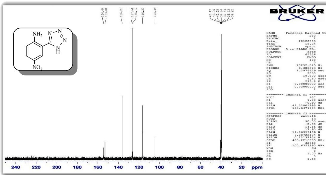
**Figure 21:**  $^{13}\text{C}$  NMR (100 MHz,  $\text{DMSO}-d_6$ ) of 4-Nitro-2-(1*H*-tetrazol-5-yl)benzenamine.
