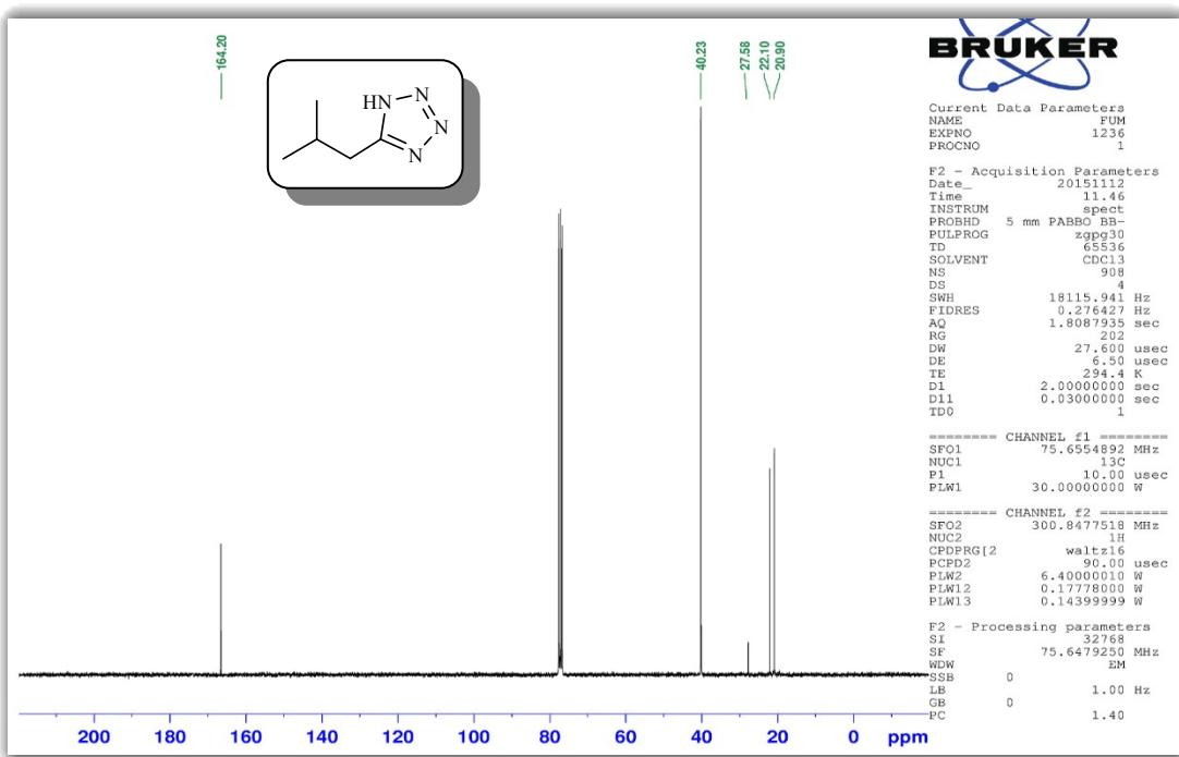
Figure 62:  $^{13}\text{C}$  NMR (75 MHz,  $\text{CDCl}_3$ ) of 5-Isobutyl-1*H*-tetrazole.
