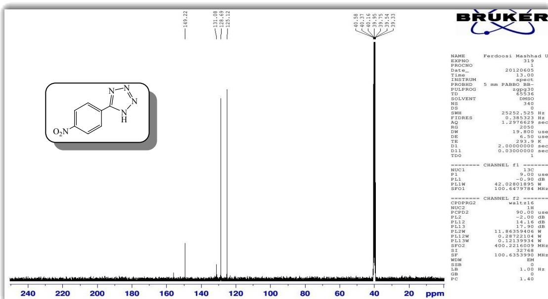
**Figure 13:**  $^{13}\text{C}$  NMR (100 MHz,  $\text{DMSO}-d_6$ ) of 5-(4-Nitrophenyl)-1*H*-tetrazole.
