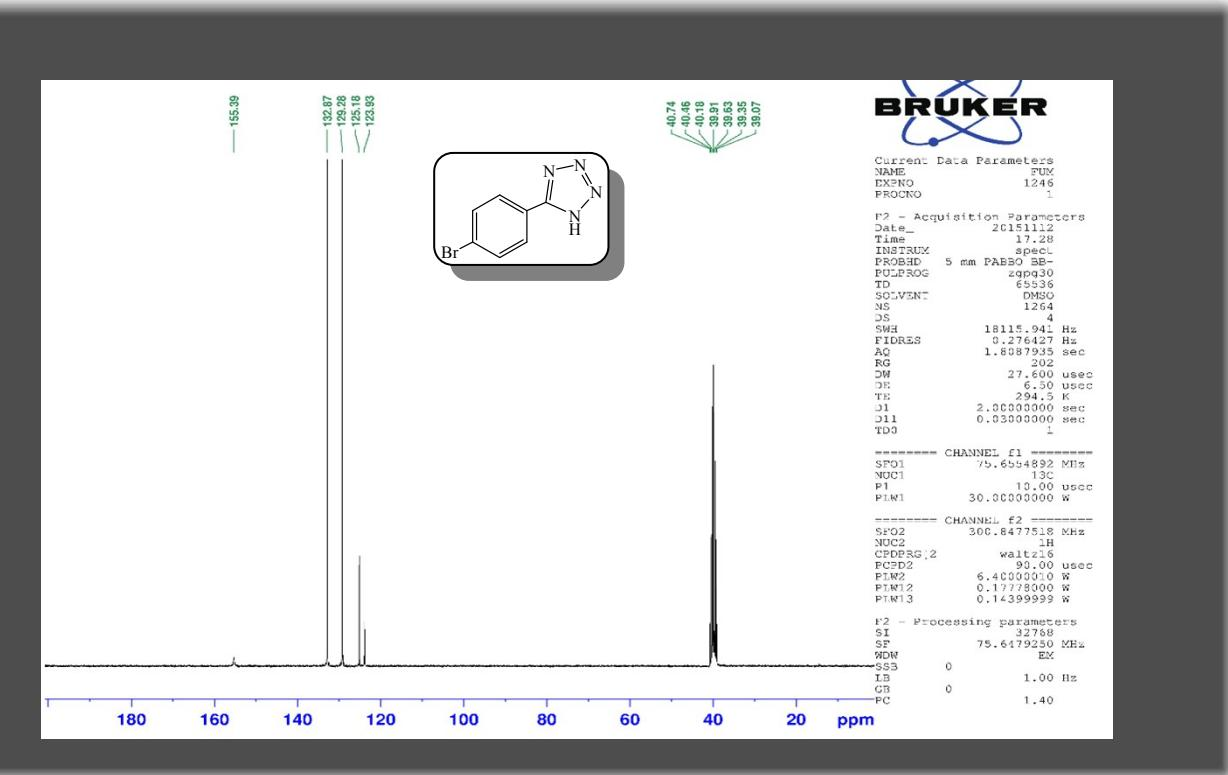
Figure 7:  $^{13}\text{C}$  NMR (75 MHz,  $\text{DMSO}-d_6$ ) of 5-(4-Bromophenyl)-1*H*-tetrazole
