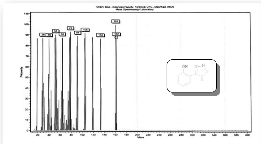
**Figure 38:** Mass spectrum of 2-(1*H*-tetrazol-5-yl)phenol.
