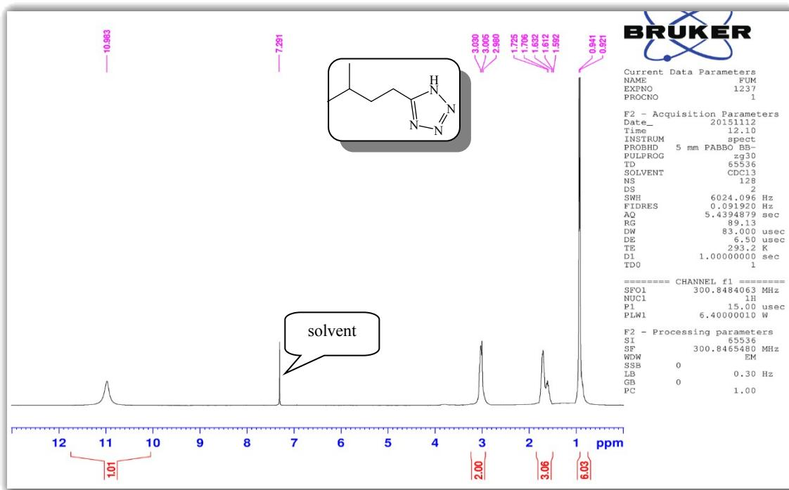
**Figure 64:** <sup>1</sup>H NMR (100 MHz, CDCl<sub>3</sub>) of 5-Isopentyl-1*H*-tetrazole.
