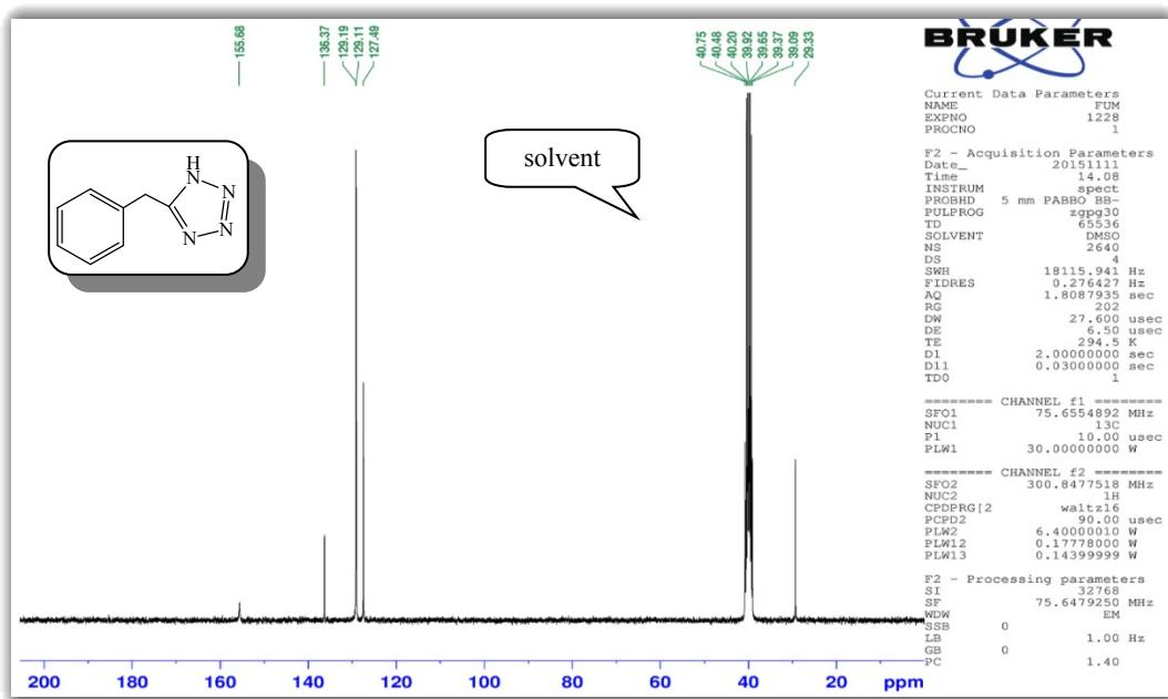
Figure 59:  $^{13}\text{C}$  NMR (75 MHz, DMSO- $d_6$ ) 5-Benzyl-1*H*-tetrazole.
