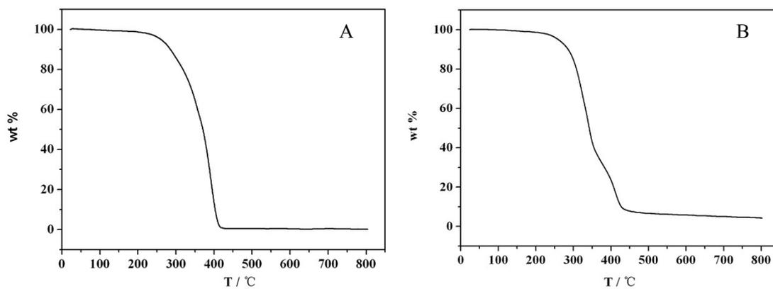
Fig .S3 TGA traces of P<sub>4,4,4,6</sub>Triz; (B) TGA traces of P<sub>4,4,4,6</sub>ATriz.
