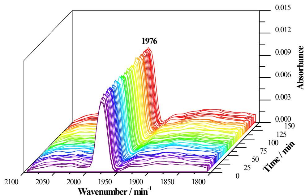
**Fig. S3** *In situ* IR spectra of the isolated **3e** in THF at room temperature.
