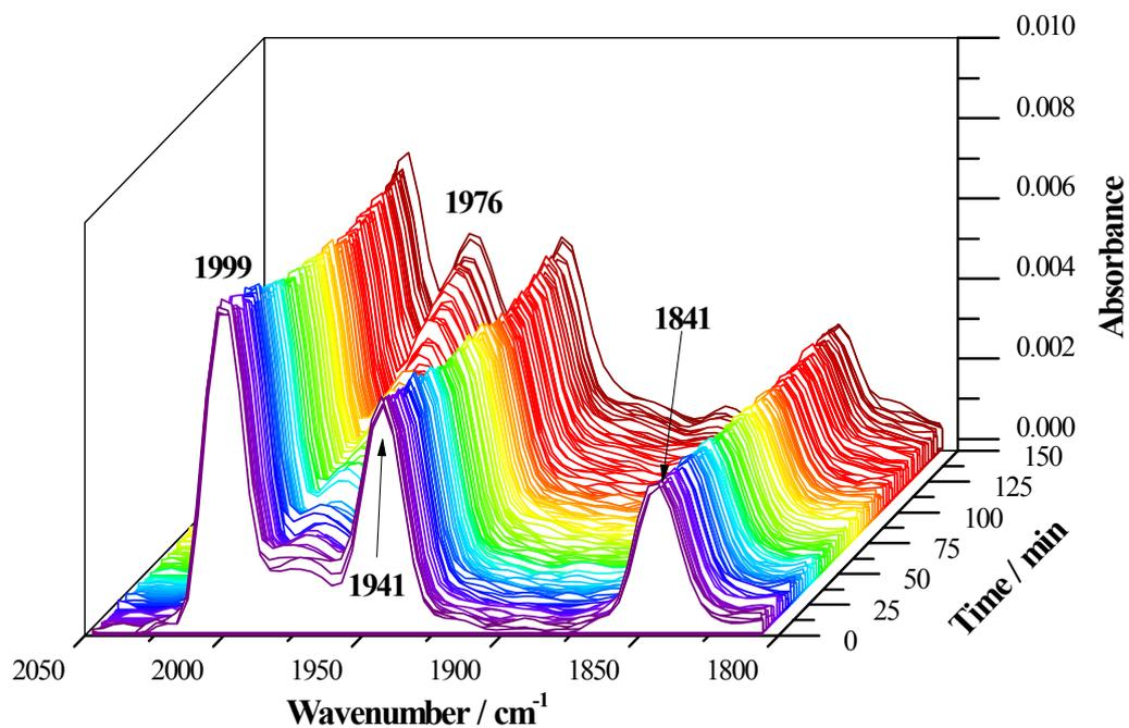
**Fig. S2** *In situ* IR spectra for conversion of the isolated **2e** into **3e** in THF at room temperature.
