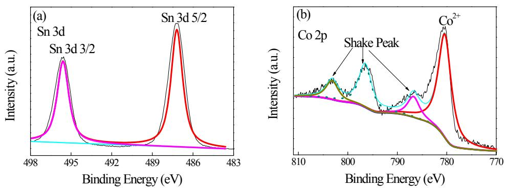
**Fig. S3** High resolution XPS spectra of (a) Sn 3d in SnO<sub>2</sub>/NG-500 and (b) Co 2p in CoO/NG-500.
