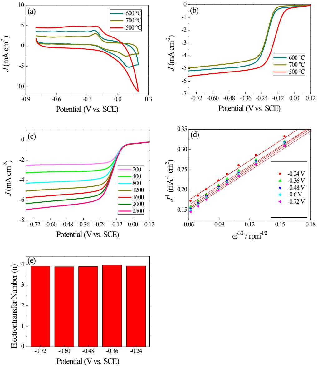
**Fig. S4** (a, b) Cycle voltammograms (a) and linear sweep voltammogram measurements (b) of CoO/SnO<sub>2</sub>/NG at different temperature; (c, d) LSV polarization curves (c) and K-L plots (d) at different potentials for CoO/SnO<sub>2</sub>/NG-500 in an O<sub>2</sub>-saturated 0.1 M KOH at 1600 rpm; (e) The  $n$  values at various potentials of CoO/SnO<sub>2</sub>/NG-500.
