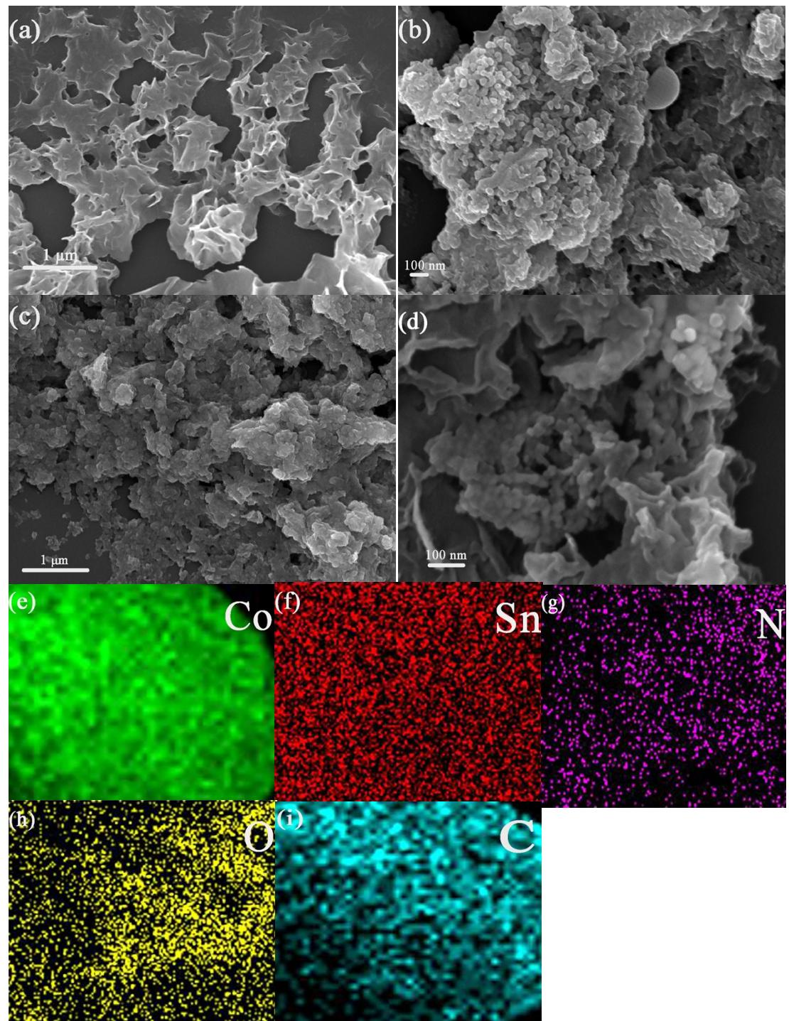
**Fig. S2** (a,b,c) SEM images of r-GO-500 (a), CoO/NG-500 (b), and SnO<sub>2</sub>/NG-500 (c); (d-i) EDX mapping of CoO/SnO<sub>2</sub>/NG-500.
