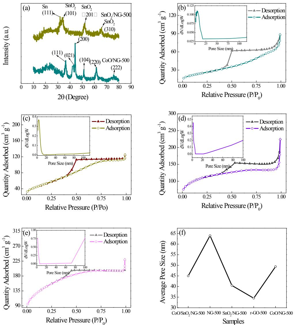
**Fig. S1** (a) XRD patterns of SnO<sub>2</sub>/NG-500 and CoO/SnO<sub>2</sub>/NG-500; (b-e) The nitrogen adsorption-desorption isotherm and the pore distribution curves inset for CoO/NG-500 (b), SnO<sub>2</sub>/NG-500 (c), NG-500 (d) and r-GO-500 (e); (f) The average pore width values of CoO/SnO<sub>2</sub>/NG-500, SnO<sub>2</sub>/NG-500, CoO/NG-500, NG-500 and r-GO-500.
