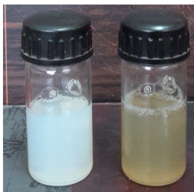
Fig. S3. Visual change in the colour of BLNP dispersion to yellowish, after the addition of \text{KMnO}_4 , indicating oxidation of \text{Ce}^{3+} to \text{Ce}^{4+} .
