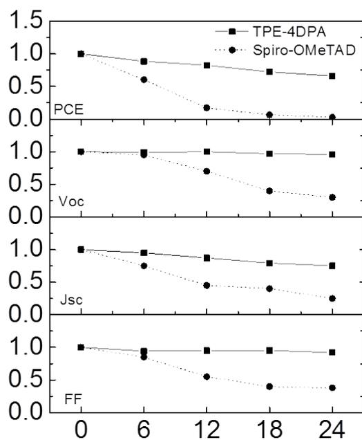
Figure S7 Normalized performance evolution of perovskite using TPE-4DPA and Spiro-OMeTAD as HTMs.
