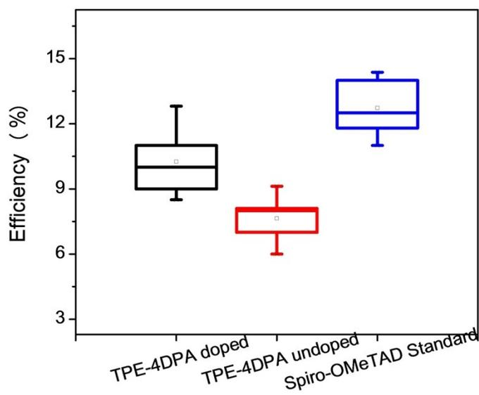
Figure S6. Statistics on the performance of perovskite solar cells using doped and undoped TPE-4DPA and standard spiro-OMeTAD as HTM
