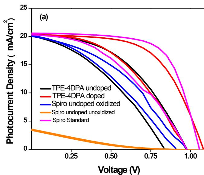
Figure S8. Current-voltage characteristics of the TPE-4DPA and Spiro-OMeTAD based perovskite solar cells in different conditions Current-voltage characteristics of the TPE-4DPA and Spiro-OMeTAD based perovskite solar cells under different conditions (in different scan directions).
