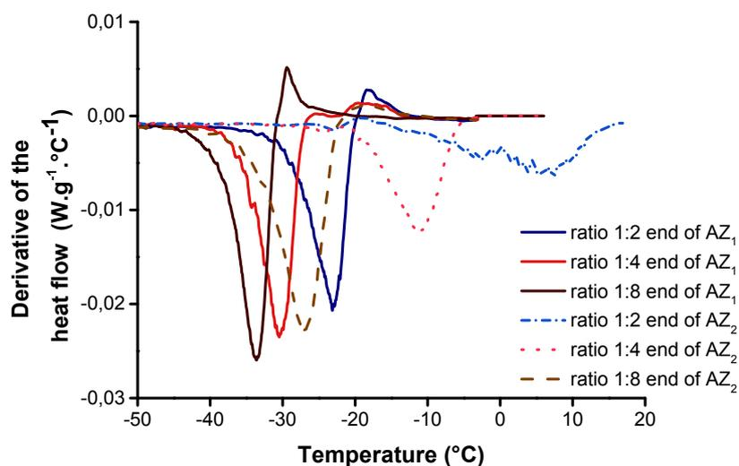
Figure ESI 2 – Derivative of the heat flow vs. temperature for different molar ratios 1:2, 1:4 and 1:8 (straight line: end of AZ<sub>1</sub>, dashed line: end of AZ<sub>2</sub>).
