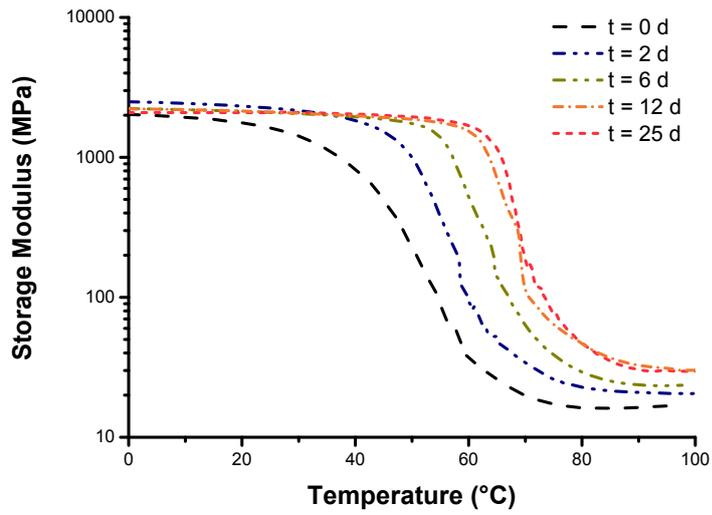
Figure ESI 3 - Storage modulus vs. temperature along AZ<sub>2</sub> progress (in days)
