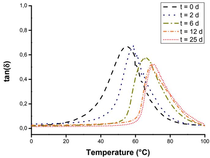
Figure ESI 4 – tan( $\delta$ ) vs. temperature along AZ<sub>2</sub> progress (in days)
