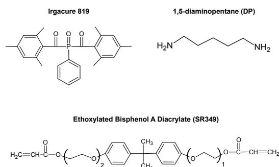
Figure ESI 1 - Chemical structures of the materials used in this study: SR349, 1,5-diaminopentane and Irgacure 819.
