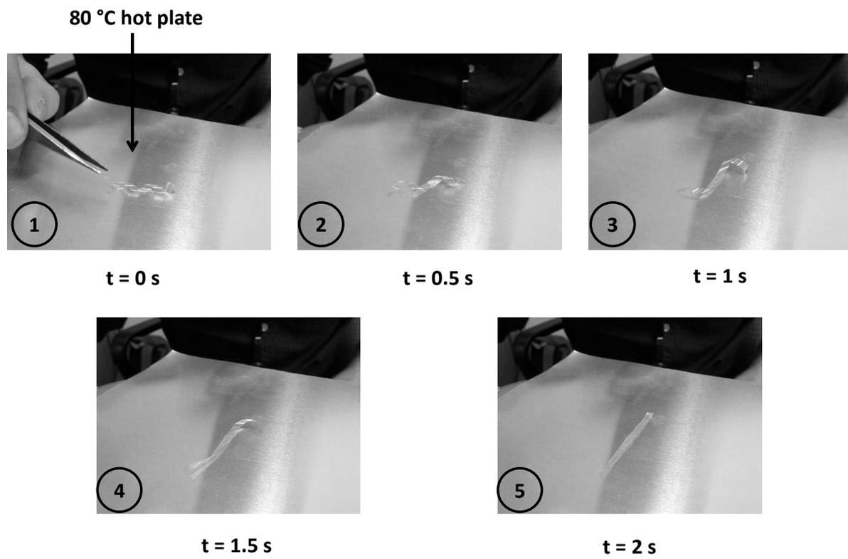
Figure 5 – Shape memory demonstration using double click aza-Michael addition and radical photopolymerization (ratio 1:4)
