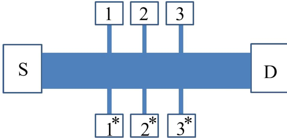
Figure S1 Schematic diagram showing a typical monolayer epitaxial graphene (EG) sample. S and D correspond to source and drain contacts. 1, 2, 3, 1\*, 2\* and 3\* are voltage probes. Channel dimensions, which are the same for all devices studied, are  $L = 0.6$  mm,  $W = 0.1$  mm, with voltage contacts spaced 0.1mm apart along both sides of the device.
