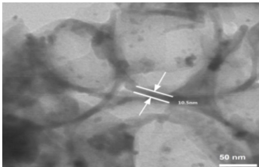
**Fig. S2** High-magnified TEM image of the hollow nanobeads SG.
