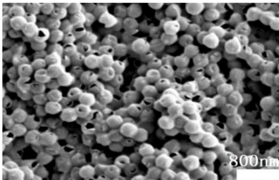
**Fig.S5** SEM image of the hollow nanobeads SG prepared by elevating the pH to 6.
