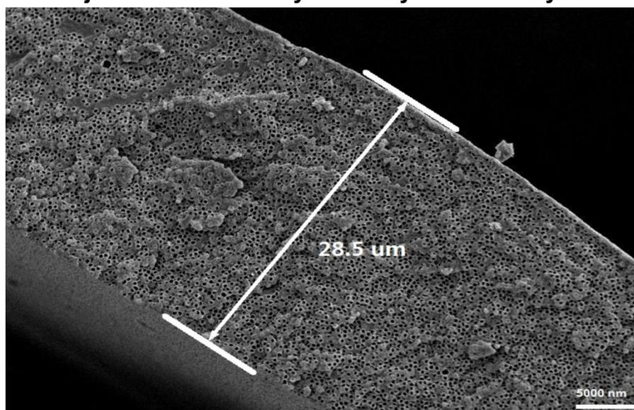
**Fig. S1 Low-magnified SEM image of the hollow nanobeads SG film.**
