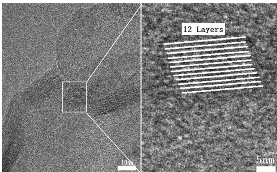
**Fig. S3** The High resolution transmission electron microscopy(HRTEM) images of the SG film of the hollow nanobeads.
