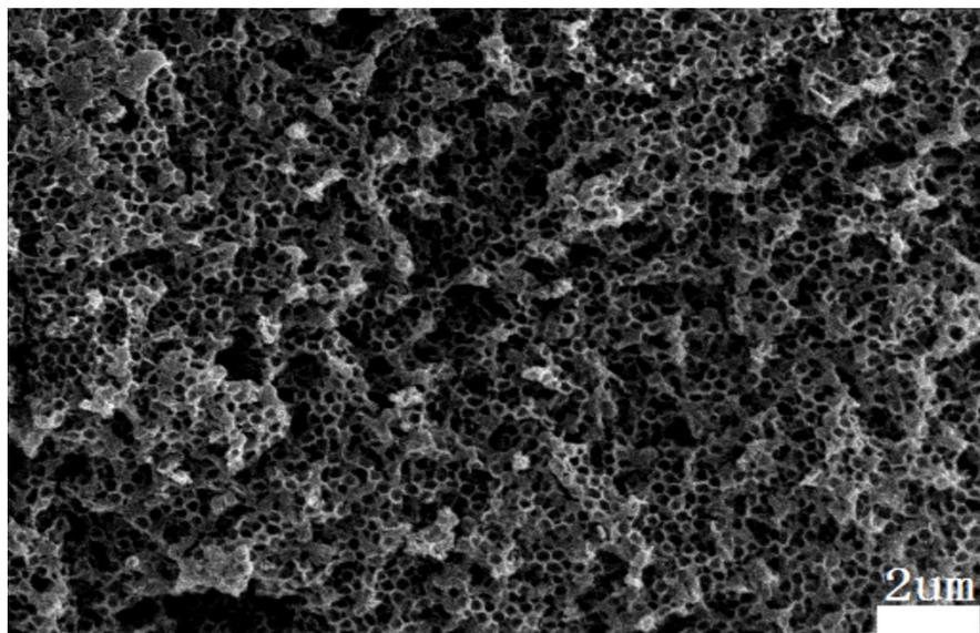
**Fig.S4** SEM image of the macro-porous SG prepared by controlling the
