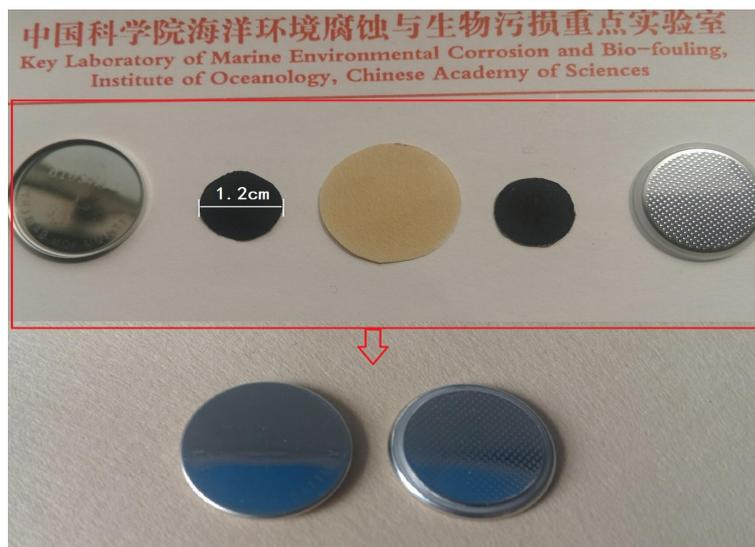
**Fig. S6** The photograph of the major parts of the supercapacitor.
