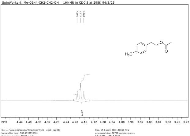
transmitter freq.: 500.133089 MHz time domain size: 32768 points width: 10000.00 Hz = 19.9947 ppm = 0.305176 Hz/pt number of scans: 16
