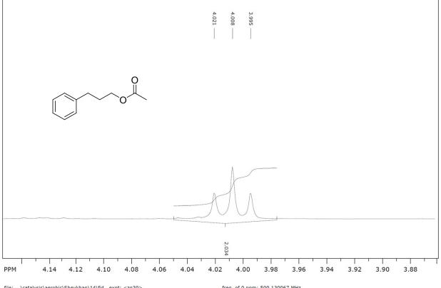
file: ...\catalysis\aerobic\Sheykhan\14\fid expt: <zg30> transmitter freq.: 500.133089 MHz time domain size: 32768 points width: 10000.00 Hz = 19.9947 ppm = 0.305176 Hz/pt number of scans: 16
