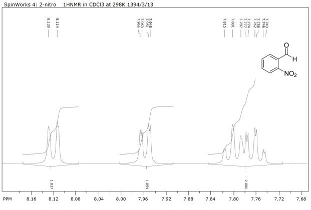
file: ...:\catalysis\aerobic\Sheykhan\2\fid expt: <zg30> transmitter freq.: 500.133089 MHz time domain size: 32768 points width: 1000.00 Hz = 19.9947 ppm = 0.305176 Hz/pt number of scans: 8 freq. of 0 ppm: 500.130023 MHz processed size: 32768 complex points LB: 0.300 GF: 0.0000 Hz/cm: 10.895 ppm/cm: 0.02178
