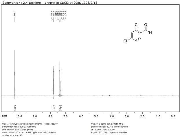
freq. of 0 ppm: 500.130055 MHz processed size: 32768 complex points LB: 0.300 GF: 0.0000 Hz/cm: 231.782 ppm/cm: 0.46344
