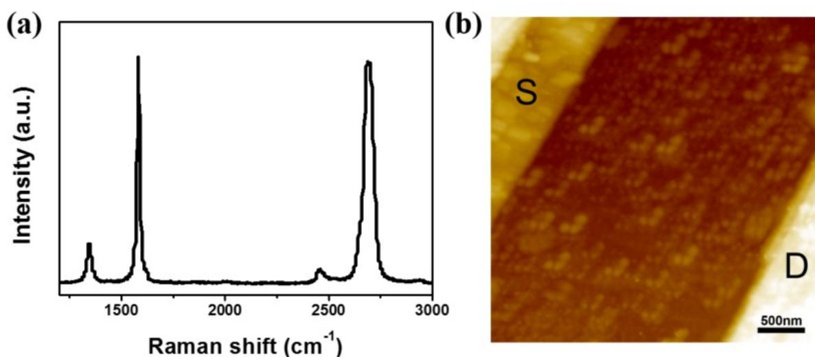
Fig. S1. (a) Raman spectra of graphene used in the study. The 2D peak and G peak of the graphene are similar intensity, which indicates bilayer graphene. (b) Top-view AFM image of graphene- $\text{CsPbBr}_{3-x}\text{I}_x$  NCs photodetector.
