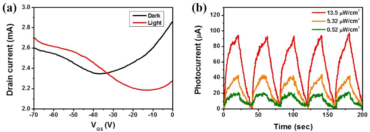
Fig. S3. (a) Transfer curve of graphene-CsPbBr<sub>3-x</sub>I<sub>x</sub> NCs photodetector as a function of gate-source voltage at 1 V<sub>DS</sub>. (b) Temporal response of graphene-CsPbBr<sub>3-x</sub>I<sub>x</sub> NCs photodetector for on/off illumination at bias 1 V<sub>DS</sub> and -60 V<sub>GS</sub>.
