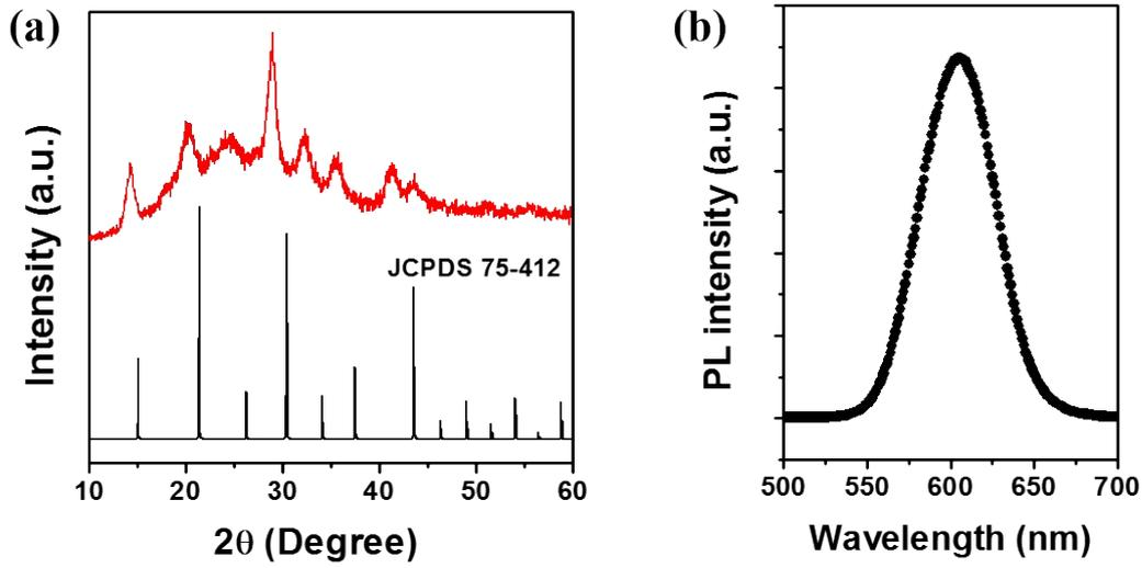
Fig. S2. (a) XRD pattern of CsPbBr<sub>3-x</sub>I<sub>x</sub> NCs (up) and CsPbBr<sub>3</sub> (down). The peaks of CsPbBr<sub>3-x</sub>I<sub>x</sub> NCs are shifted to low angle at comparing peaks of the CsPbBr<sub>3</sub> NCs. Doping large I atom to CsPbBr<sub>3</sub> NCs results in the extend lattice. (b) PL spectra of CsPbBr<sub>3-x</sub>I<sub>x</sub> NCs.
