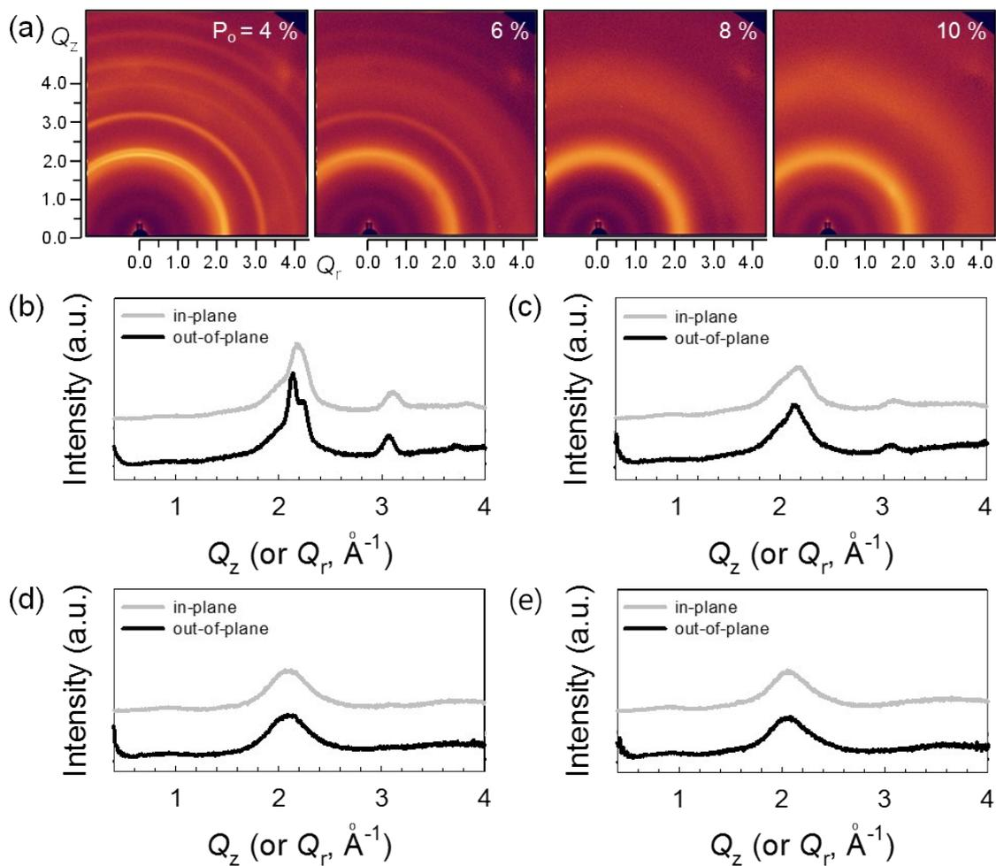
**Figure S1.** (a) 2D GIXD patterns of as-deposited SnO<sub>x</sub> films fabricated at P<sub>O</sub> = 4, 6, 8, and 10 %. (b–e) 1D in-plane and out-of-plane X-ray profiles extracted from the patterns shown in (a): (b) 4, (c) 6, (d) 8, and (e) 10 % P<sub>O</sub> samples.
