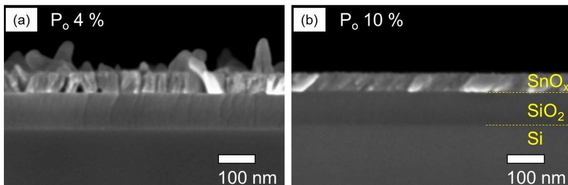
**Figure S5.** SEM micrographs of 45-nm-thick SnO<sub>x</sub> films fabricated under P<sub>o</sub> of (a) 4% and (b) 8%, and both subsequently annealed at 210 °C for 1 h.
