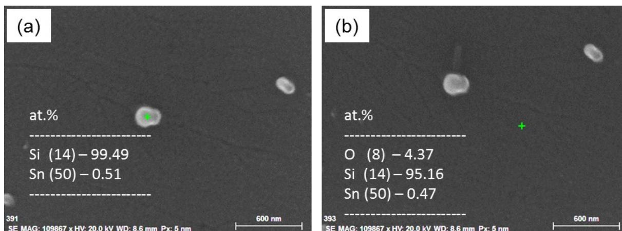
**Figure S3.** Energy dispersive X-ray spectroscopy (EDS) analysis of atomic composition in the  $\text{SnO}_x$  thin films (15-nm-thick) deposited on a Si substrate under  $P_{\text{O}}$  of 8 % and heat-treated at 210 °C for 1 h: (a) at the irregular protrusion and (b) outside of the irregular protrusion.
