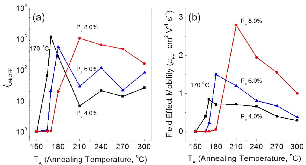
**Figure S4.** TFT performance metrics extracted from transfer characteristics of bottom gate TFTs prepared using  $\text{SnO}_x$  thin films (15-nm-thick) deposited under  $P_O$  of 4–8 % and heat-treated at  $T_A$  of 150–300 °C: (a)  $I_{ON/OFF}$  ratio and (b) field effect mobility ( $\mu_{FE}$ ).
