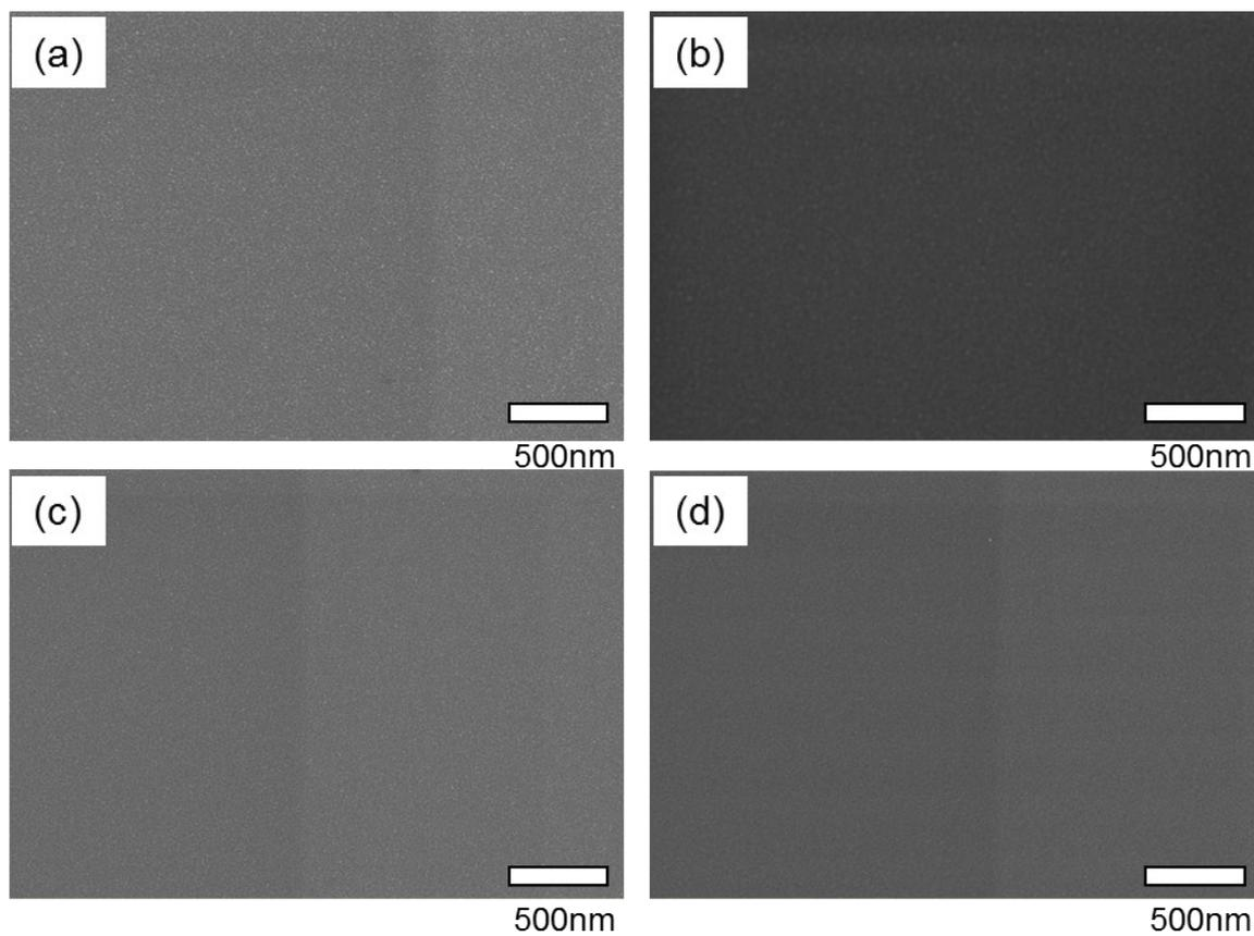
**Figure S2.** SEM images of as-deposited SnO<sub>x</sub> thin films (15-nm-thick) fabricated under various P<sub>O</sub>: (a) 4, (b) 6, (c) 8, and (d) 10 %.
