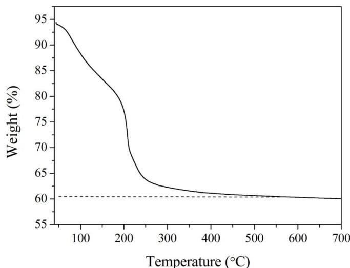
**Fig. S1** TG curve of the mixture of  $\text{Ce}(\text{NO}_3)_3 \cdot 6\text{H}_2\text{O}$  and  $\text{Co}(\text{NO}_3)_3 \cdot 6\text{H}_2\text{O}$  loaded on KIT-6 ( $\text{Co}/(\text{Ce}+\text{Co}) = 30 \text{ mol\%}$ ).
