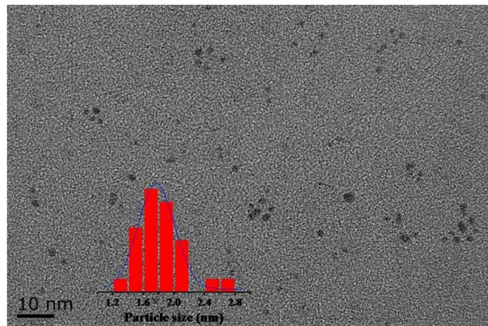
**Fig. S3** TEM image of PAMAM dendrimers-templated Pt NPs (inset is the particle size distribution histogram of Pt NPs).
