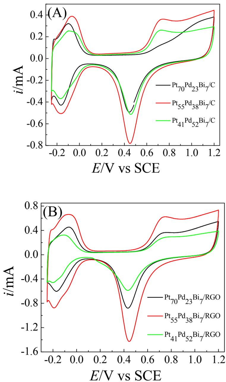
**Figure S1** Cycle voltammograms of  $\text{Pt}_{70}\text{Pd}_{23}\text{Bi}_7$ ,  $\text{Pt}_{55}\text{Pd}_{38}\text{Bi}_7$  and  $\text{Pt}_{41}\text{Pd}_{52}\text{Bi}_7$  catalysts supported on Vulcan XC72 carbon (A) and RGO (B) in 0.5 mol/L  $\text{H}_2\text{SO}_4$  at a scan rate of  $50 \text{ mV}\cdot\text{s}^{-1}$ .
