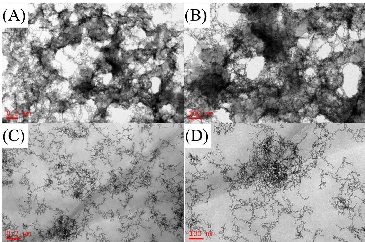
**Figure S2** TEM images of Pt<sub>55</sub>Pd<sub>38</sub>Bi<sub>7</sub>/C (A and B) and Pt<sub>55</sub>Pd<sub>38</sub>Bi<sub>7</sub>/RGO (C and D) with different magnifications.
