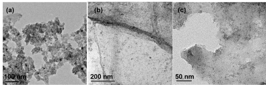
**Figure S5.** (a-c) Low resolution TEM images of  $\text{CuFe}_2\text{O}_4/\text{RGO}$  NCs with 15, 45 and 60 wt % graphene content respectively.
