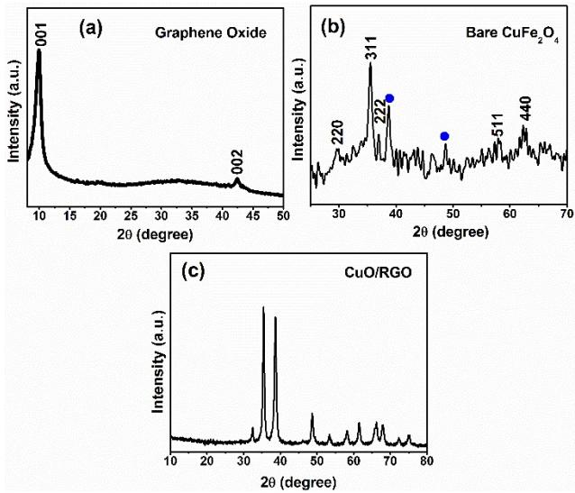
**Figure S1.** Powder XRD spectrum of (a) graphene oxide, (b) bare CuFe<sub>2</sub>O<sub>4</sub> NPs (impurity peaks of CuO marked with blue dot) and (c) CuO/RGO nanocomposites.
