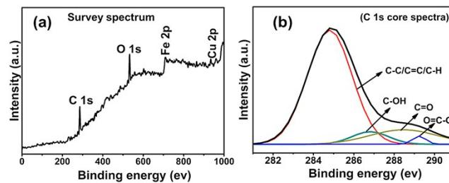
**Figure S4.** (a) Broad XPS spectrum and (b) C 1s core spectrum of CuFe<sub>2</sub>O<sub>4</sub>/RGO nanocomposites.
