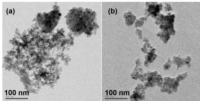
**Figure S6.** (a-b) Low resolution TEM images of bare  $\text{CuFe}_2\text{O}_4$  NPs.
