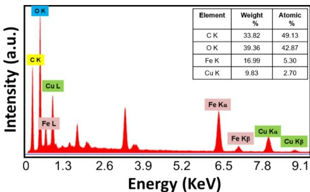
**Figure S2.** SEM-EDS analysis of CFRNCs.
