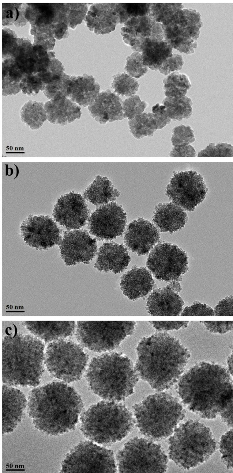
**Fig. S2.** TEM images of (a) 70 nm, (b) 100 nm and (c) 130 nm colloidal superparamagnetic nanocrystal clusters.
