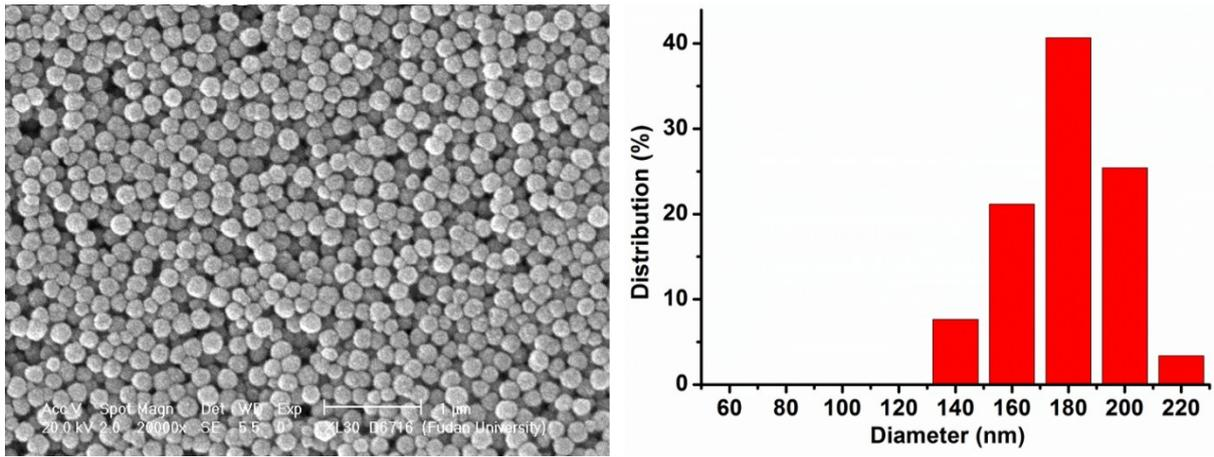
**Fig. S1.** SEM image and corresponding size distribution plot of 180 nm colloidal superparamagnetic nanocrystal clusters.
