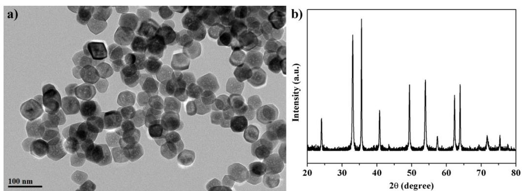
**Fig. S4.** TEM image (a) and XRD pattern (b) of  $\alpha$ -Fe<sub>2</sub>O<sub>3</sub> nanoparticles. Uniform  $\alpha$ -Fe<sub>2</sub>O<sub>3</sub> nanoparticles would be obtained when pure water was used as the solvent.
