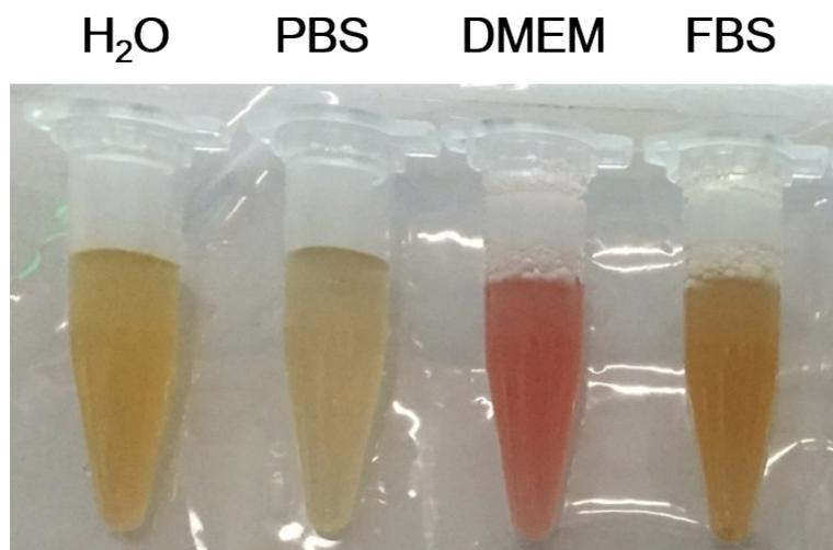
**Fig. S9.** The colloidal stability of 85 colloidal superparamagnetic nanocrystal clusters in H<sub>2</sub>O, PBS, DMEM and FBS at the concentration of 50  $\mu\text{g mL}^{-1}$  for 1 h.
