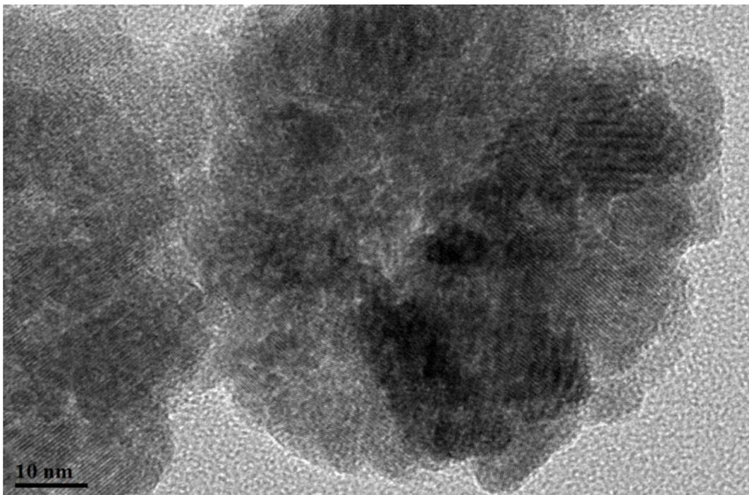
**Fig. S5.** The HRTEM image of 70 nm colloidal superparamagnetic nanocrystal clusters.
