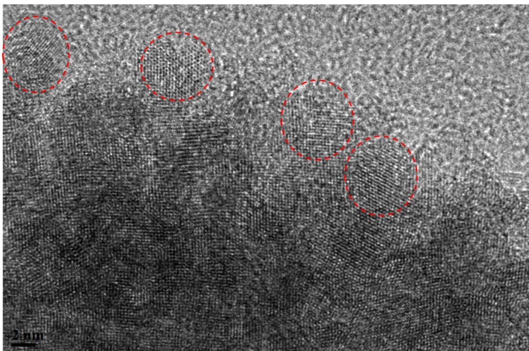
**Fig. S6.** The HRTEM image of 85 nm colloidal superparamagnetic nanocrystal clusters. The individual particles are marked by the red dash lines.
