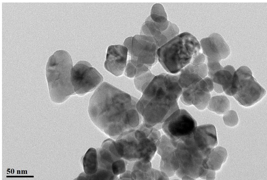
**Fig. S3.** TEM image of the sample with the content of water increased to 4.0 mL. Irregular nanoparticles are obtained.
