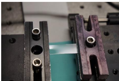
Figure S1. A homemade stretcher setup for pre-stretching PDMS substrate.
