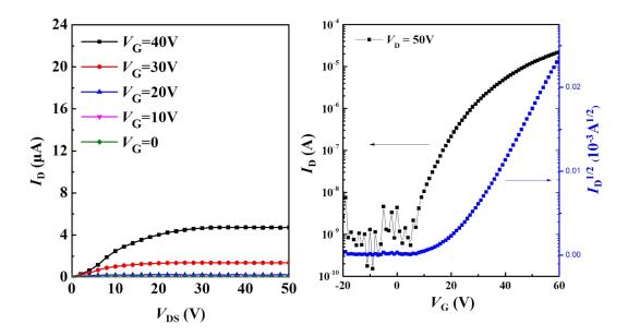
**Figure S2.** The output and transfer characteristics of *n*-type OFET-based memory devices with pure PCPI electret.
