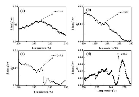
**Figure S1.** The derivative of the heat flux with respect to temperature obtained from the temperature-dependent DSC curves of native PI and PCPI/PI mixed polymers with different weight ratios of PCPIs: (a) 0, (b) 6%, (c) 10%, and (d) 20%.
