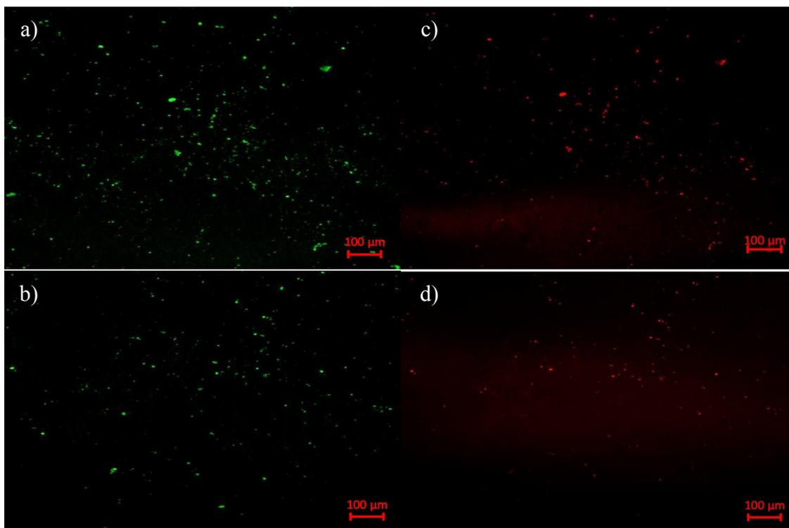
**Fig. S4** Confocal fluorescence microscopy images of the GOQD at the excitation wavelength of 473 nm collecting the fluorescence between (a-b) 490 and 590 nm; and (c-d) 570 and 670 nm.
