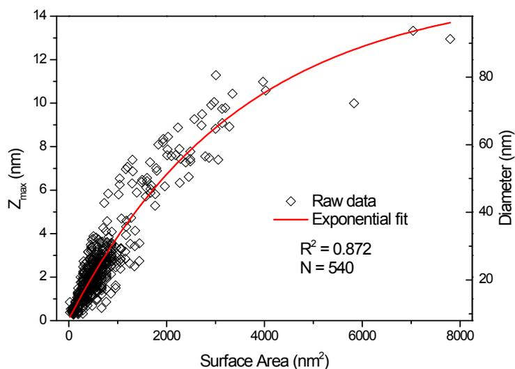
**Fig. S3** Exponential function fitting between surface area and height (or equivalent diameter) for GOQD measured by AFM.
