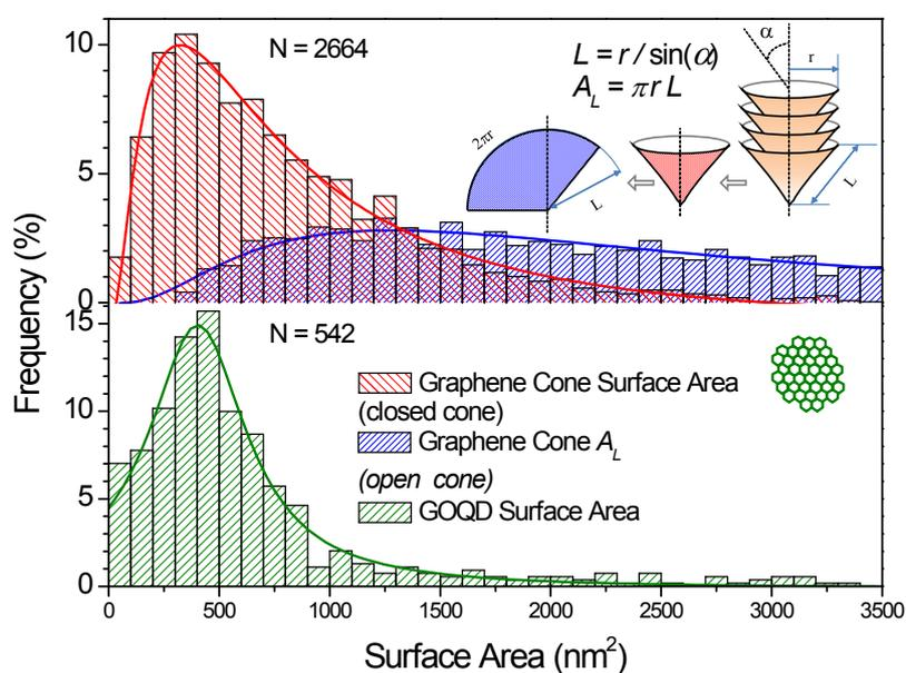
**Fig. S2** CNF cone lateral area (estimated using diameters and  $\alpha$  angles of CNF observed by TEM) and GOQD surface area log-normal distributions; e) representation and calculation of the lateral area of an open graphene cone in a CNF structure.
