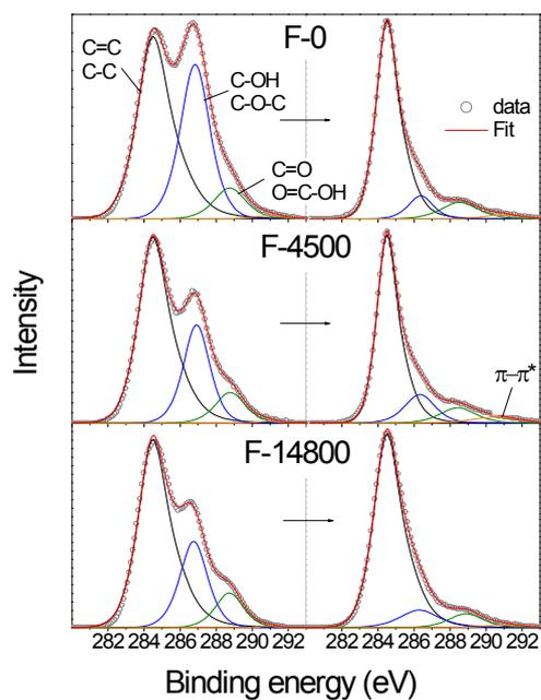
**Fig. S1** Deconvoluted C1s spectra of some fractions before (left) and after hydrothermal reduction (right).
