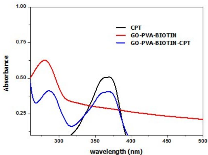
**Fig. S4** UV absorbance spectra of GO-biotinPVA (15.0 mg/L) after GO-biotinPVA- CPT (15.0 mg/L) and CPT (10.  $\mu$ M) in to the GO -biotinPVA in PBS buffer solution (pH 7.4) at 37  $^{\circ}$ C.
