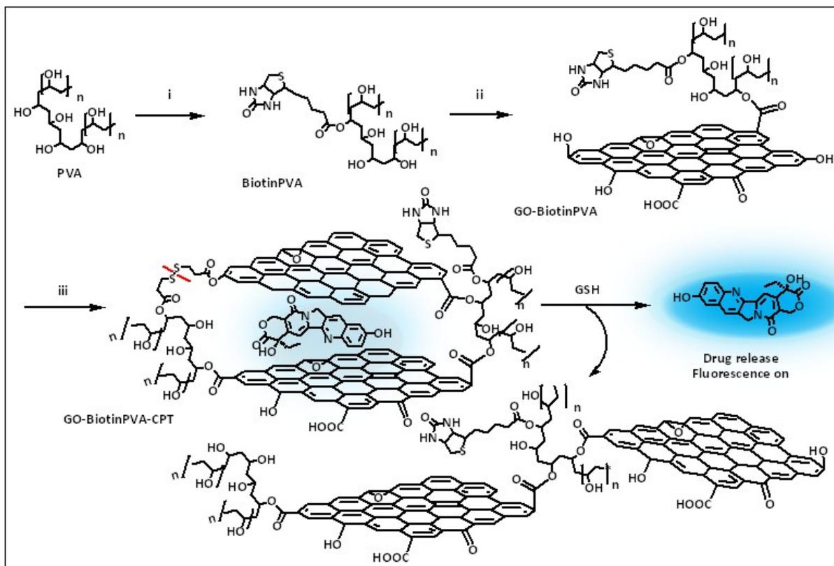
**Reagents and Reaction conditions:** i) D-biotin, EDC.HCl, DMAP, DMSO, RT, 24 h; ii) GO, EDC.HCl, DMAP, DMSO, RT, 24 h; iii) camptothecin (CPT), 3,3'-dithiodipropionic acid, EDC.HCl, DMAP, DMSO, RT, 24h.
