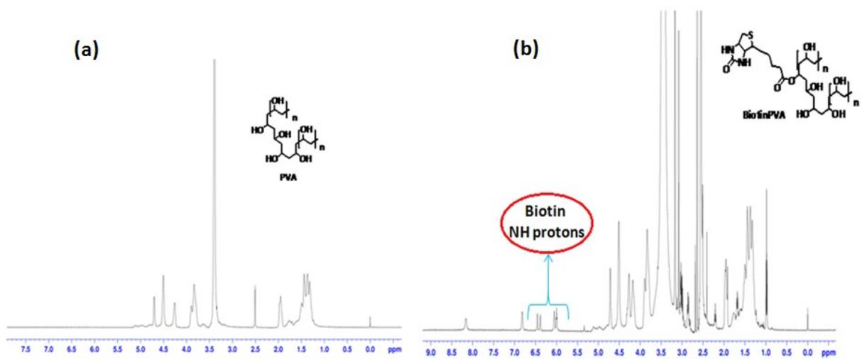
**Fig. S2** <sup>1</sup>H-NMR spectra of (a) PVA; (b) biotinPVA in DMSO-d<sub>6</sub>.
