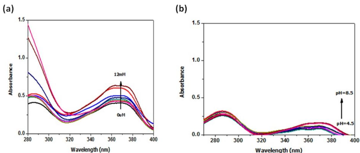
**Fig. S6** UV absorbance spectra of (a) GO-biotinPVA-CPT,(300 μg/mL) in the presence of different concentrations of GSH (0.0 μM – 12.0 mM) in PBS buffer solution (pH=7.4; 10% DMSO) at 37 °C; (b) GO-biotinPVA-CPT,(300.0μg/ mL) for different pH (4.5-8.5) in PBS buffer solution at 37 °C.
