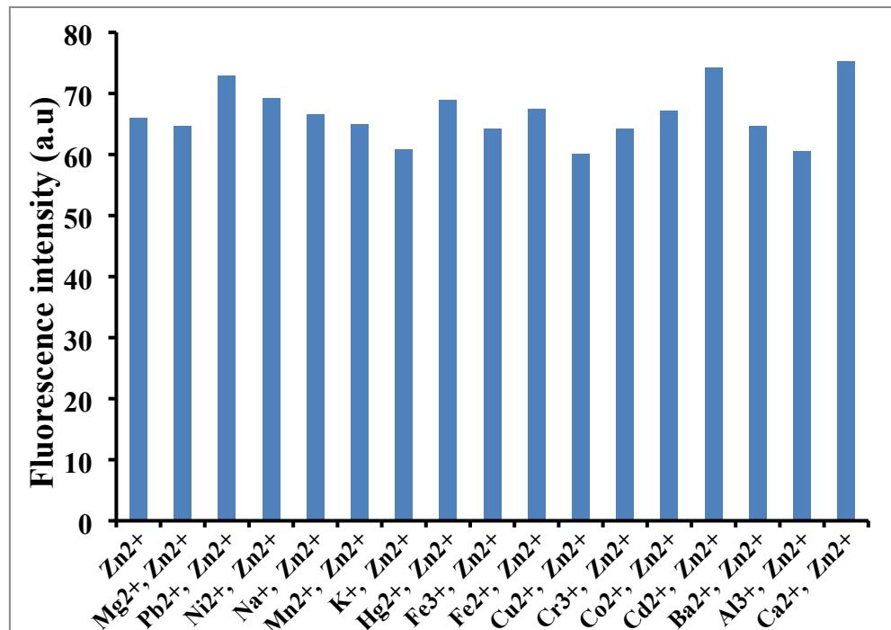
**Fig. S8** Change in fluorescence intensity of **1** (10 µM) in H<sub>2</sub>O:CH<sub>3</sub>CN (3:7, v/v) medium upon addition of 3 equiv. of Zn<sup>2+</sup> ions along with 5 equiv. of other metal ions
