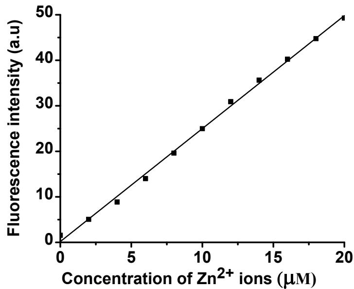
**Fig. S9** Linear response of **1** (10  $\mu\text{M}$ ) in the presence of  $\text{Zn}^{2+}$  ions (0–20  $\mu\text{M}$ ) in  $\text{H}_2\text{O}:\text{CH}_3\text{CN}$  (3:7, v/v) medium. The detection limits was calculated using the equation,  $\text{DL} = 3\sigma / \text{slope}$ .
