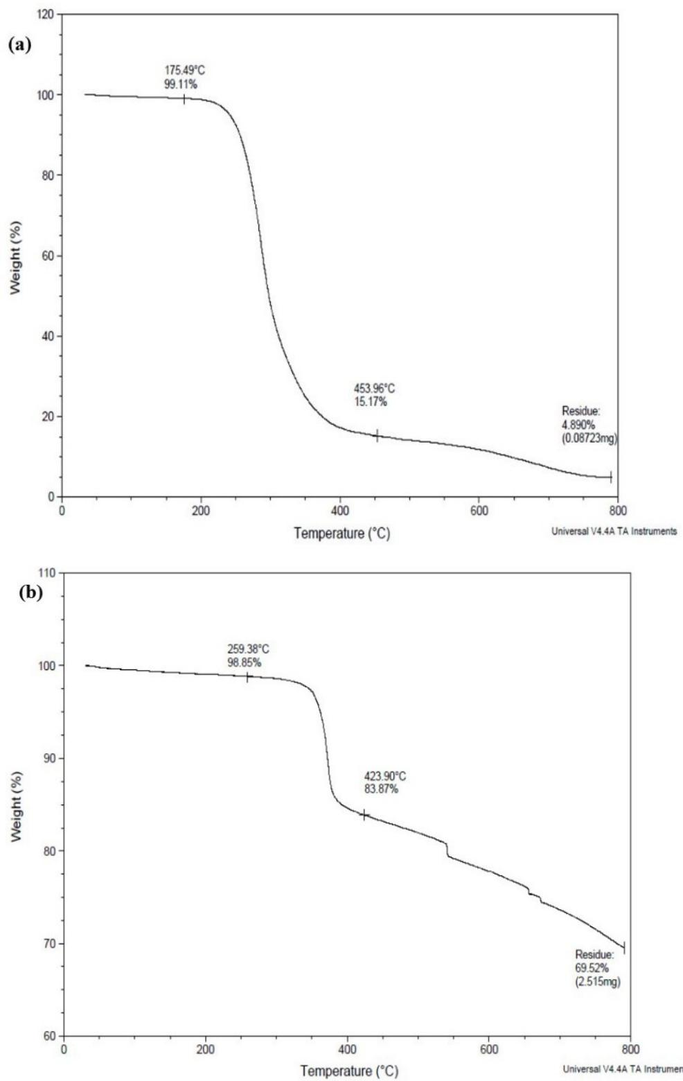
Fig. S13 TGA curve of **1** (a) and **1-Zn<sup>2+</sup>** complex (b)
