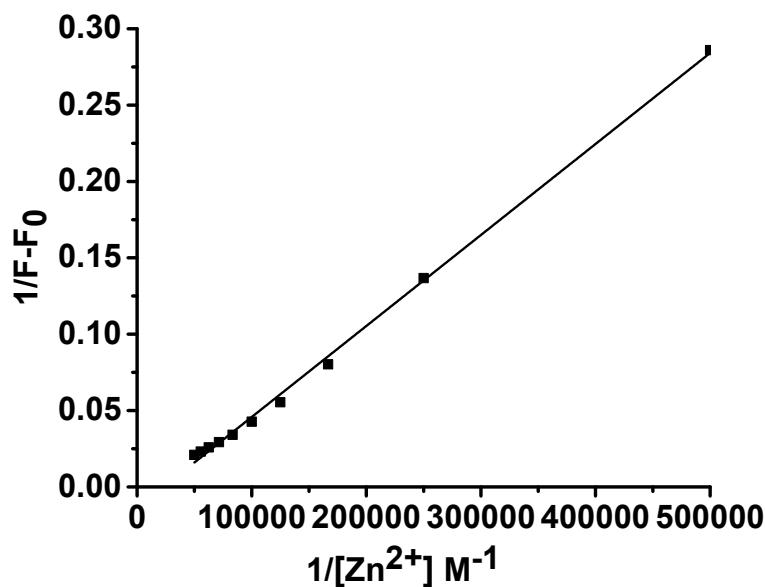
**Fig. S10** Benesi–Hildebrand plot obtained from the titration of **1** with  $\text{Zn}^{2+}$  ions in  $\text{H}_2\text{O}:\text{CH}_3\text{CN}$  (3:7, v/v) medium
