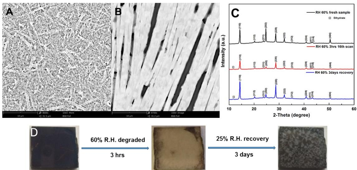
**Figure S4.** The SEM images of (A) fresh spin-coated perovskite film and (B) film recovered for 3 days from degradation (humidity of 60% for 3 hrs). (C) The XRD patterns of fresh spin-coated perovskite film, the degraded film (3 hrs under R.H. 60%) after 16 scans of X-ray irradiation (72min, 4.5min/scan), and film recovered 3 days under R.H. of 25%. Labeled peaks in the sample belong to the tetragonal perovskite phase. (D) Photographs of perovskite films from fresh to recovered stage.
