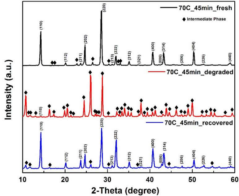
**Figure S1.** The XRD patterns of (A) fresh perovskite film, (B) degraded under humidity of 60%  $\pm$  5% for 14 days, (C) the film recovered from degraded phases. The intensity in all patterns is normalized for comparison.
