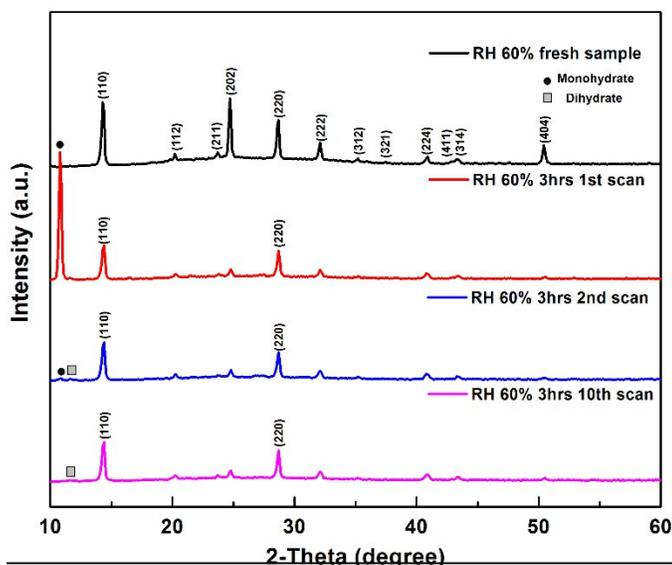
**Figure S3.** The XRD patterns of spin-coated perovskite films degraded under controlled humidity of 60% for 3 hrs. Major recovery occurred during the first scan of 5 min X-ray exposure. However, the observed recovery should be mainly due to the low humidity level 25% during XRD measurement. After 10 consecutive X-ray irradiation scans (4.5min/scan), no further recovery was observed. The labeled peaks belong to the tetragonal perovskite phase.
