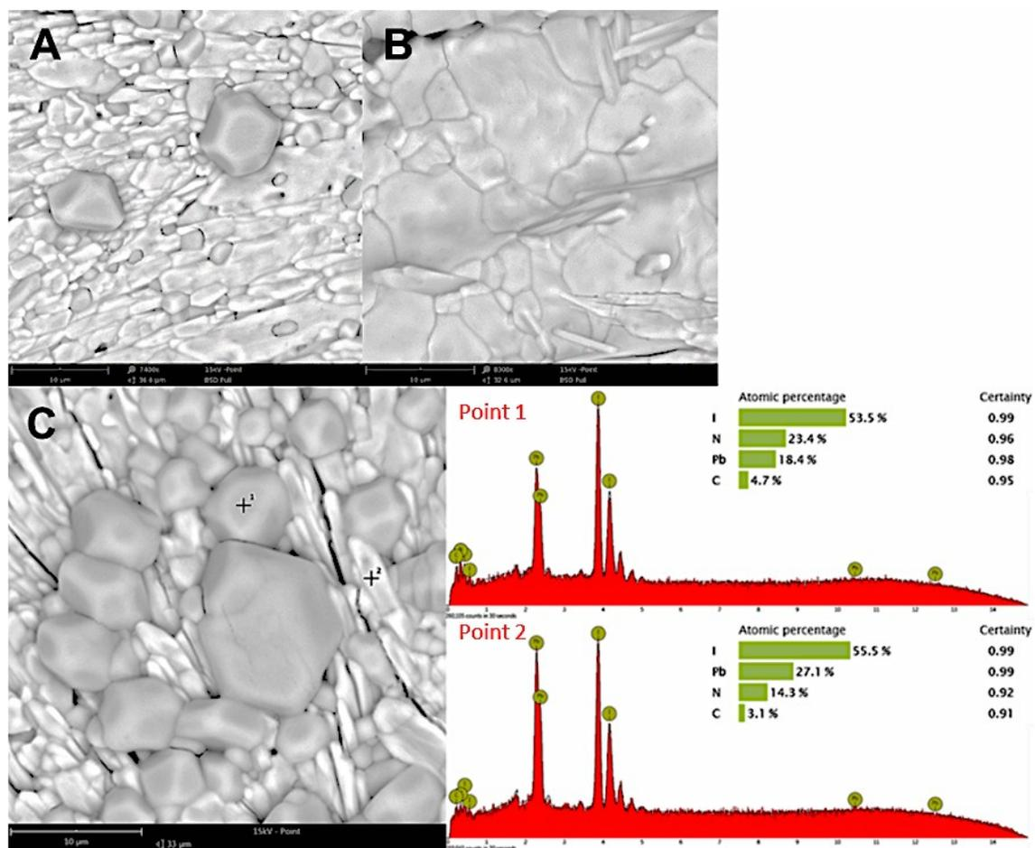
**Figure S10.** The SEM images and EDX spectrum of the low moisture recovered sample, A) at 7400x magnification, acquired from the center part; B) at 8300x magnification, acquired from the edge part; C) EDX spectrum acquired at point 1 and point 2 in image C with a scale bar 10 μm, indicating the formation of MAI rich perovskite grains nucleated from the PbI<sub>2</sub> rich bulk body.
