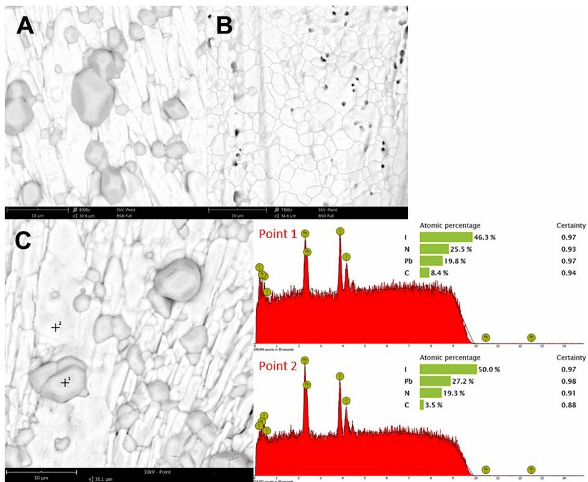
**Figure S11.** The SEM images and EDX spectrum of the heat recovered sample, A) at 8300x magnification, acquired from the center part; B) at 7800x magnification, acquired from the edge part; C) EDX spectrum acquired at point 1 and point 2 in image C with a scale bar 10 $\mu$ m, indicating the formation of MAI rich perovskite grains nucleated from the PbI<sub>2</sub> rich bulk body.
