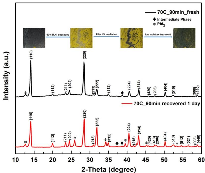
**Figure S6.** XRD patterns of a fresh perovskite film prepared at 70°C for 90 min and recovered after 15 minutes UV irradiation and low humidity exposure. The inset shows photographs of
