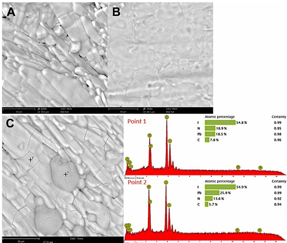
**Figure S8.** The SEM images and EDX spectrum of the X-ray recovered sample, A) at 8200x magnification, acquired from the center part; B) at 7500x magnification, acquired from the edge part; C) EDX spectrum acquired at point 1 and point 2 in image C with a scale bar 10 $\mu$ m, indicating the formation of stoichiometric perovskite grains nucleated from the PbI<sub>2</sub> rich bulk body.
