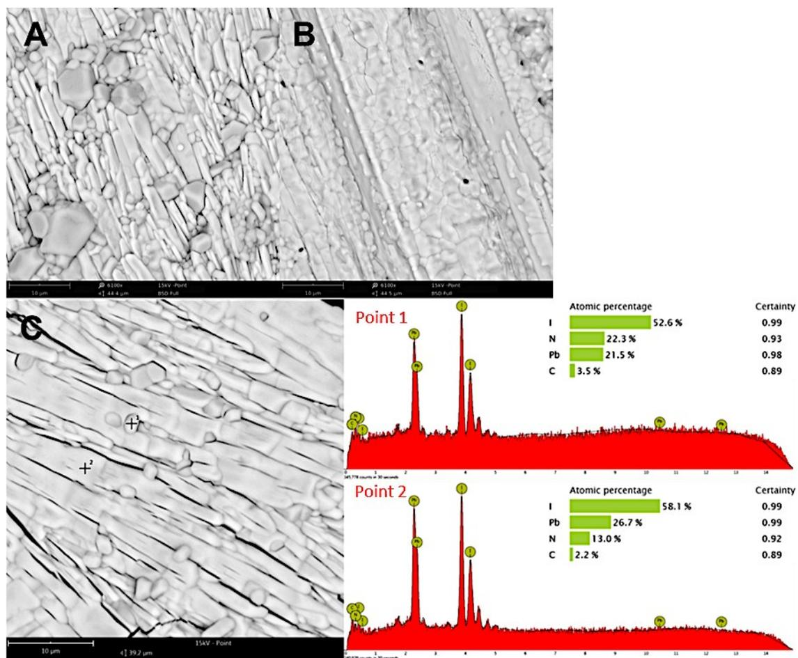
**Figure S9.** The SEM images and EDX spectrum of the E-beam recovered sample, A) at 6100x magnification, acquired from the center part; B) at 6100x magnification, acquired from the edge part; C) EDX spectrum acquired at point 1 and point 2 in image C with a scale bar 10μm, indicating the formation of stoichiometric perovskite grains nucleated from the MAI rich bulk body.
