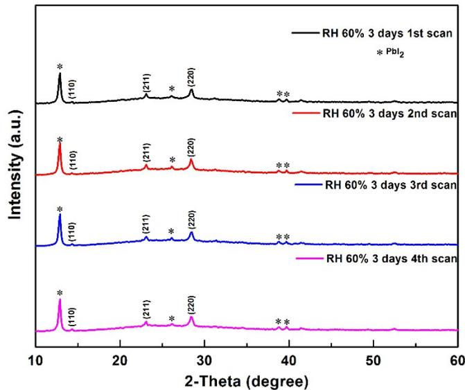
**Figure S2.** The XRD patterns of spin-coated perovskite films degraded under humidity of 60% for 3 days, after 4 scans of X-ray irradiation (50min, 12.5min/scan), no obvious recovery was observed through X-ray treatment. Labeled peaks in the sample belonging to the tetragonal perovskite.
