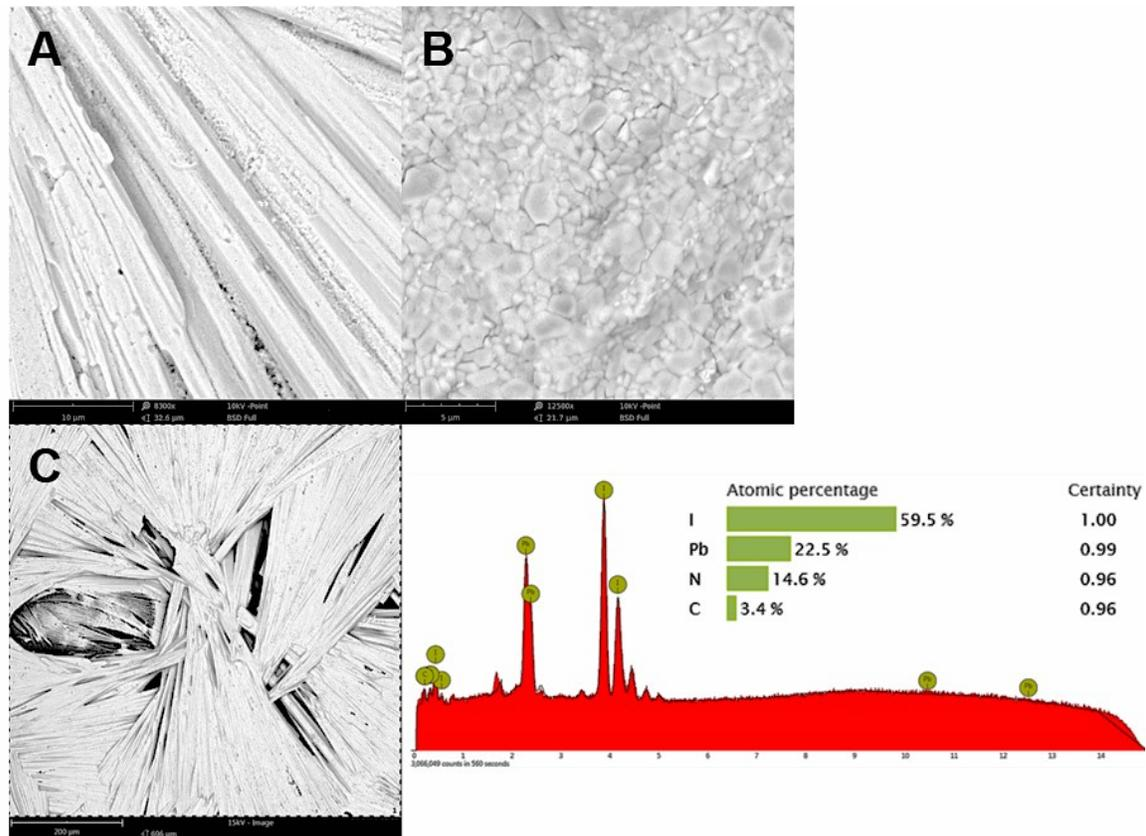
**Figure S7.** The SEM images and EDX spectrum of the fresh sample prepared at 70°C for 45min under vacuum, A) at 8300x magnification, acquired from the center part; B) at 12500x magnification, acquired from the edge part; C) EDX spectrum acquired by overview scanning of the region in image C with a scale bar 200μm. The fan-shaped morphology formed in the drop-casted sample prepared under vacuum.
