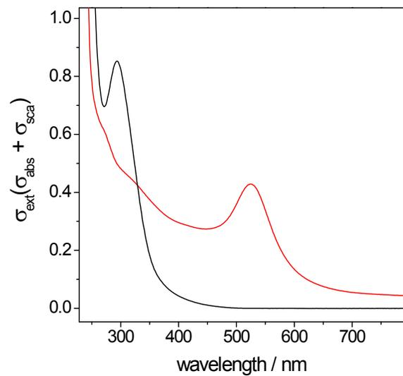
**Fig. S1.** UV-Vis spectra of the aqueous 1 mM HAuCl<sub>4</sub> solution (black line), and AuNP-PAH suspension (red line). Electronic spectra were recorded on Jasco V-670 spectrophotometer.
