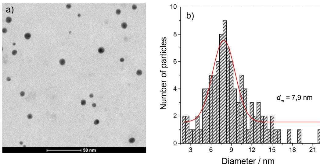
**Figure S2.** a) Transmission Electron Microscopy image of AuNPs-PAH; b) histogram of size distribution obtained by counting 100 particles. Images were recorded on FEI TECNAI G<sup>2</sup> F20 HRTEM.
