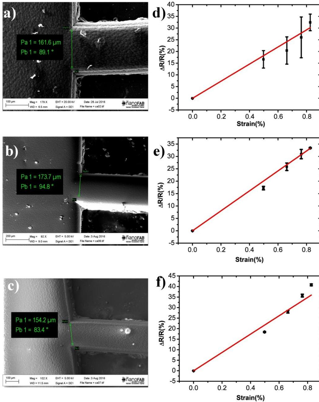
**Fig S1. a)-c)** SEM images of various PDMS stencils made by the same mold. The three PDMS stencils were selected when the silicon mold had been used for 15, 20 and 25 times, respectively. **d)-f)** Resistance change - strain characteristics of devices fabricated using the stencils shown in a)-c), respectively.
