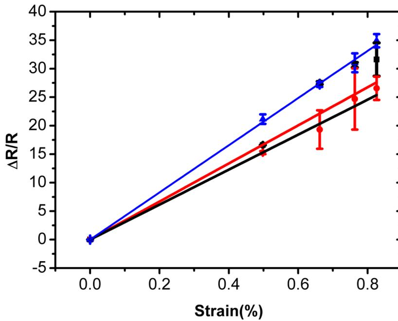
**Fig. S3.** Resistance change – strain characteristics of a device after repeated bending. The red, black, and blue curves show data of the device going through 0, 10 and 40 bending cycles, respectively.
