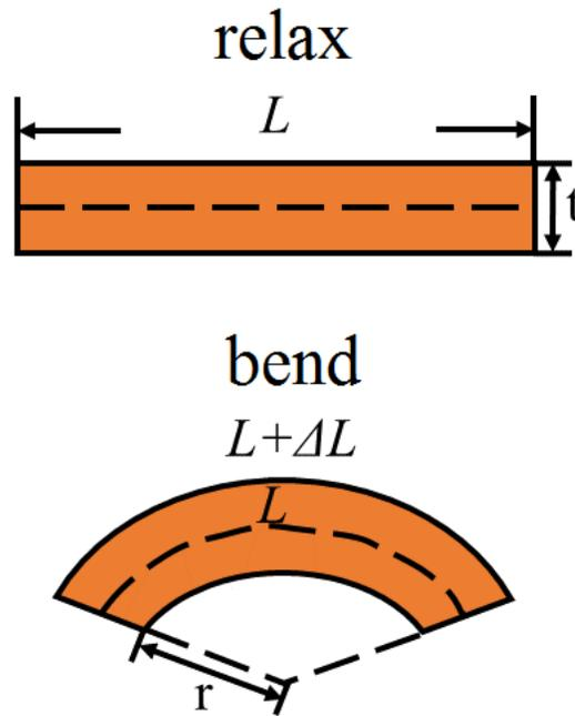
**Fig. S4.** Illustration of bending strain calculation
