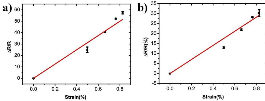
**Fig. S2.** The resistance change - strain characteristics of strain sensors made by the same PDMS stencil as the device shown in Fig. 5 in the manuscript.
