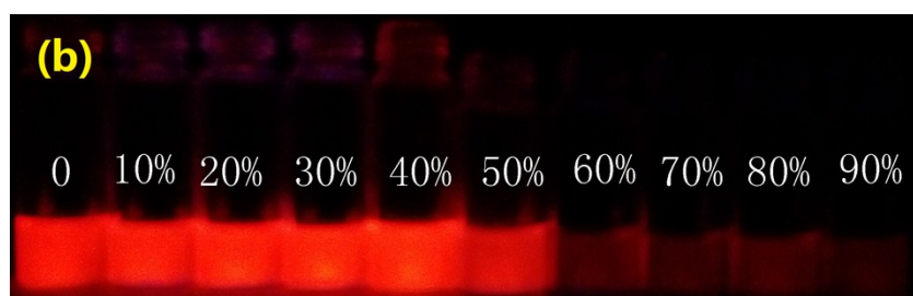
Fig.S16 (a) PL intensity vs f_w and (b) emission photographs of DPP2 in THF/water mixtures with different f_w values.
