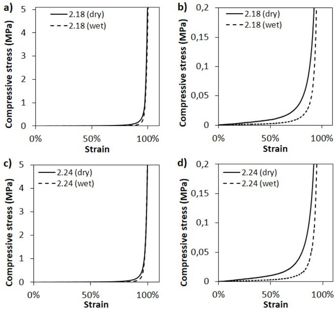
**Figure S4.** Compressive stress-strain curves of the GO-Col scaffolds at pH 2. **a-b)** 18% of collagen/GO w/w ratio; **c-d)** 24% of collagen / GO w/w ratio.
