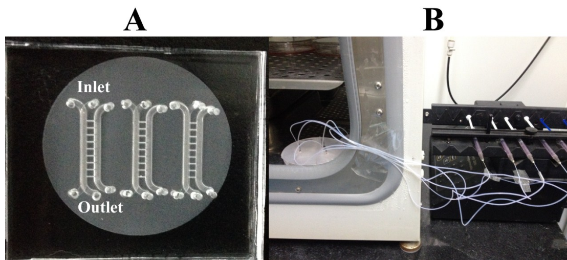
Fig. S1 Dynamic coculture Caco-2, HepG2, and U251 cells in microfluidic chip. (A) Photo of the fabricated microfluidic chip. (B) The integration of dynamic coculture microfluidic chip device.
