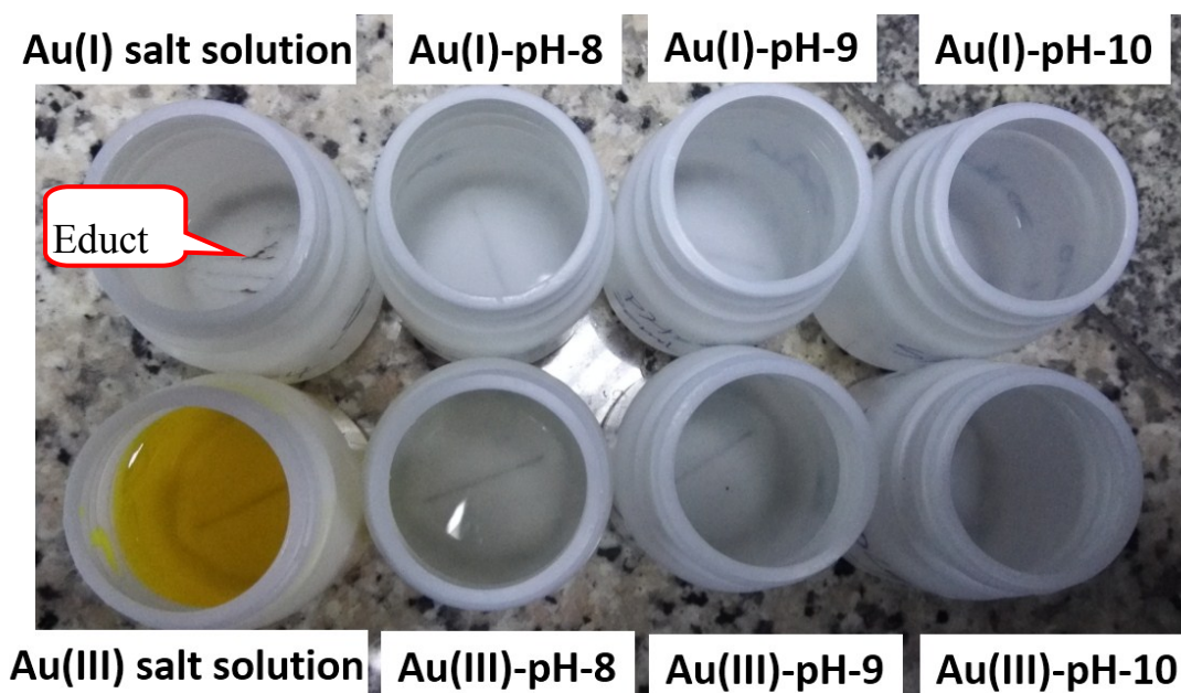
Fig. S2 Photographs of gold electrolytes and gold salt solution placed 2 weeks; all electrolytes had good stability except Au(I) salt solution.
