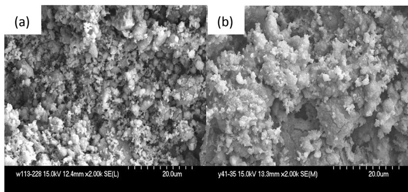
Fig. S1 SEM of as-prepared (a)  $\gamma$ -AlH<sub>3</sub>/MgCl<sub>2</sub> nano-composite doped with Zn and Zr and (b)  $\gamma$ -AlH<sub>3</sub>/MgCl<sub>2</sub> nano-composite.
