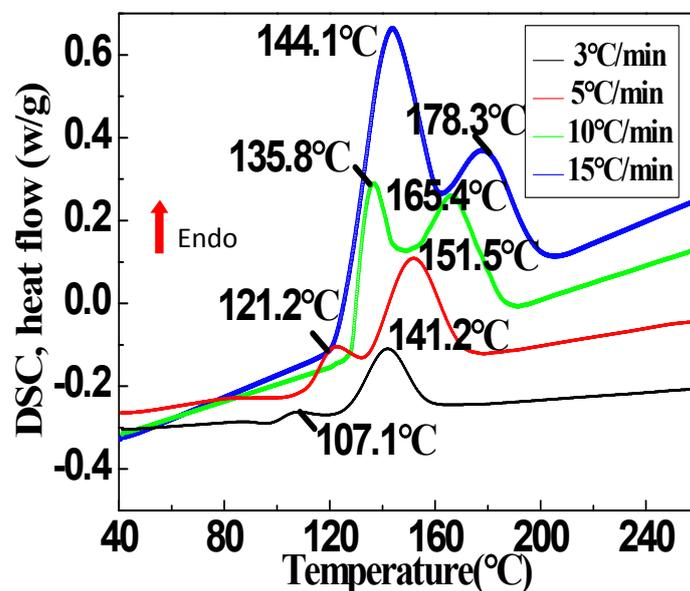
Fig. S3 DSC curves of the  $\gamma$ -AlH<sub>3</sub>/MgCl<sub>2</sub> nano-composite doped with Zn and Zr.
