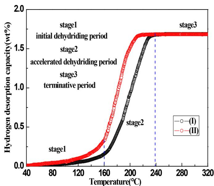
Fig. S2 TPD curves of as-prepared (I)  $\gamma\text{-AlH}_3/\text{MgCl}_2$  nano-composite and (II)  $\gamma\text{-AlH}_3/\text{MgCl}_2$  nano-composite doped with Zn and Zr. The hydrogen content is given as a percentage of the calculated salt.
