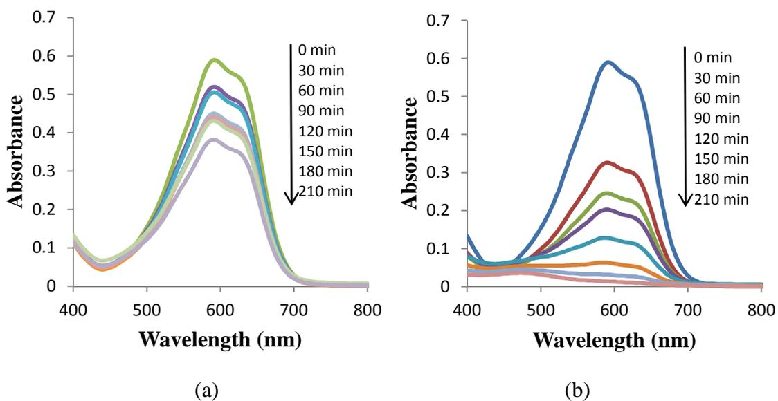
**Figure S4.** Absorbance spectra for the dye Remazol Brilliant Blue R in the presence of the Cotton-TiO<sub>2</sub> samples heated at (a) 80 °C; (b) 110 °C. “0 min” means the time of the irradiation starting. The contact between the samples and the dye solution started 60 min before.
