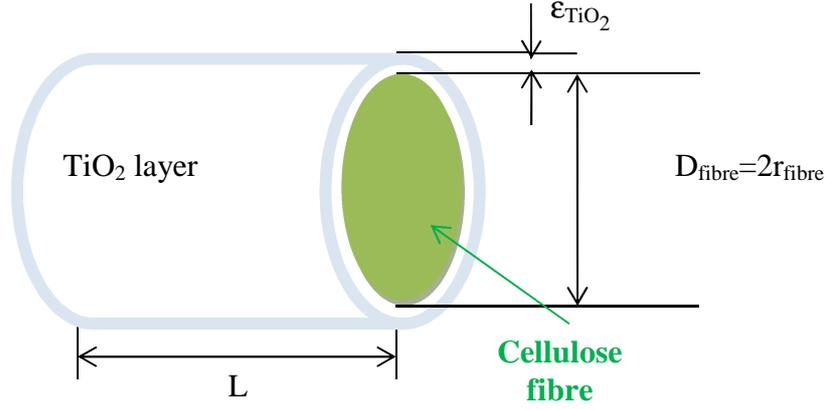
**Scheme S1.** Cellulose fibre covered with a thin layer formed by a compact packing of TiO<sub>2</sub> nanoparticles.
