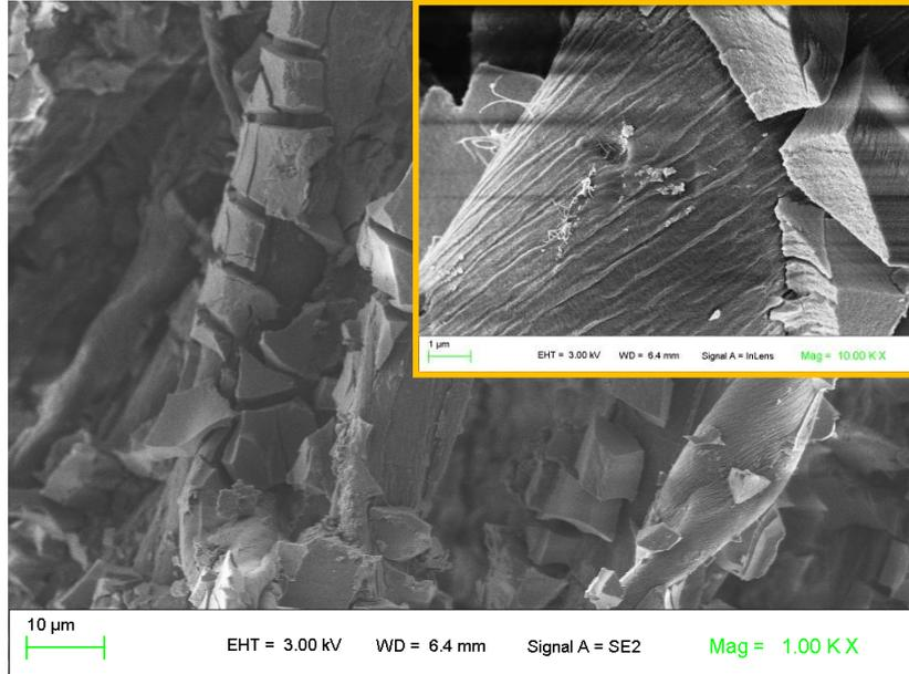
**Figure S3.** SEM observation of cotton fibres treated with  $\text{Ti}(\text{OBu})_4$  in tert-butanol at 1 wt.% for 12 h without acetic acid, followed by a hydrothermal treatment at 120 °C during 3 h.
