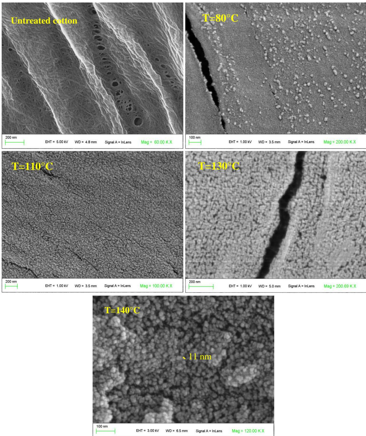
**Figure S2.** FE-SEM images samples of untreated cotton and functionalized with TiO<sub>2</sub> NPs prepared with hydrothermal treatments held at different temperatures: 80 °C, 110 °C, 130 °C and 140 °C.
