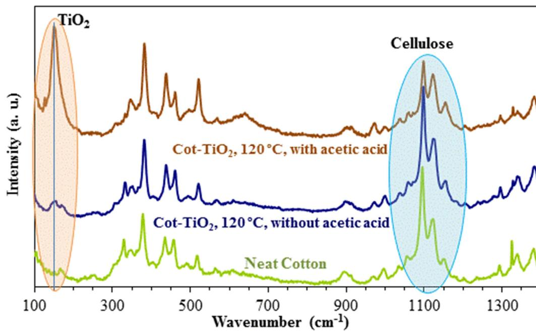
**Figure S1.** Raman spectra of neat cotton and cotton-TiO<sub>2</sub> after hydrothermal treatment at 120 °C in presence of acetic acid and in the absence of acetic acid. (Acetic acid was added during the first phase of the treatment).
