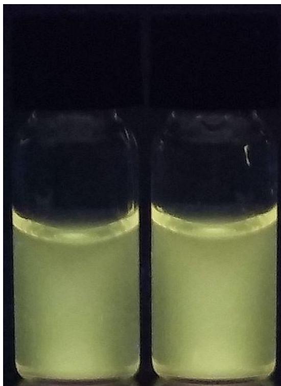
Figure S4 The photographs of S-free GQDs aqueous solution at the absence (left) and presence (right) of 140.0 \mu\text{M} Pb 2+ at 365 nm UV irradiation.
