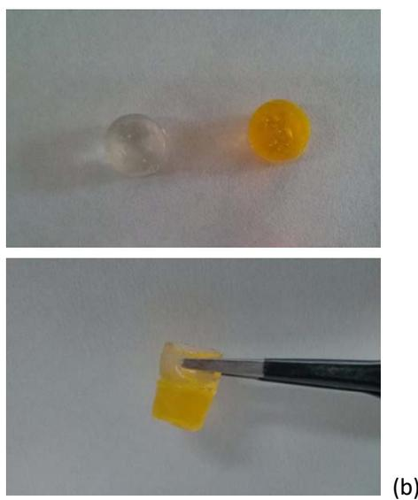
**Scheme S1.** (a) Mechanism of in situ gelation of GC and OHC-PEO-CHO. (b) A demonstration of the self-healing behavior of the GC/OHC-PEO-CHO hydrogel.
