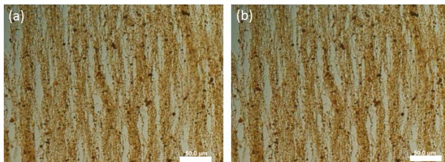
**Figure S4.** Firmness of the adhered silica rods on the GC/OHC-PEO-CHO hydrogel surface monitored by optical microscope before (a) and after (b) the surface was washed by PBS for three times. Scale bar: 50  $\mu\text{m}$ .
