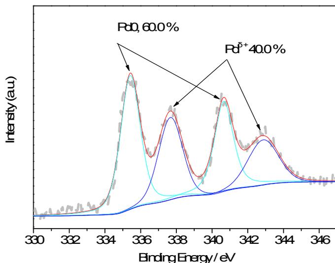
Fig. S7. Pd3d spectra of Pd/CN-CF.
