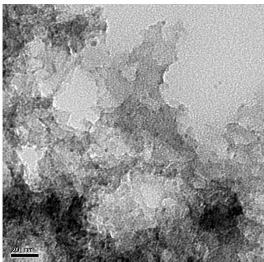
**Fig. S14.** TEM image of Pd/CN-CF after the 6th run.
