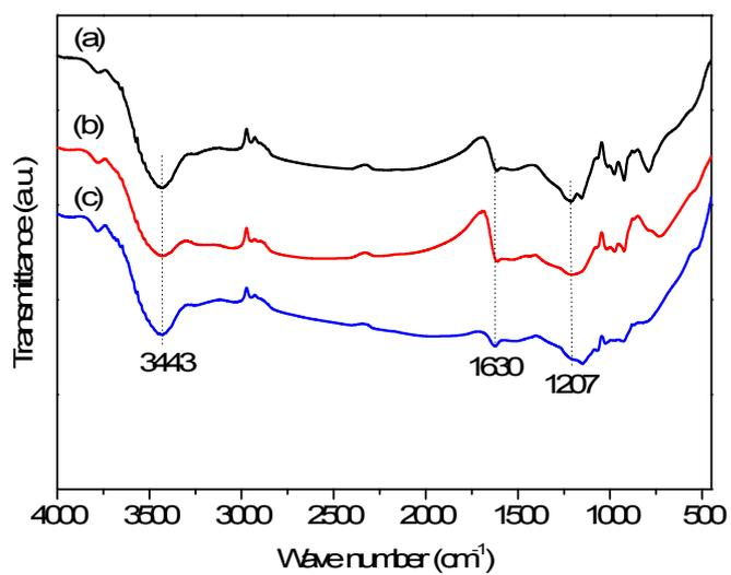
Fig. S3. FTIR patterns of (a) CN-CT, (b) CN-CF and (c) CN-TE.
