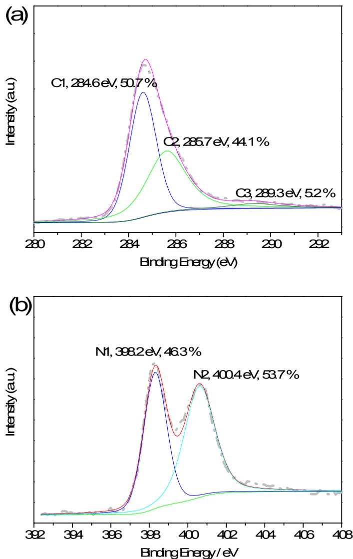
**Fig. S4.** (a) C1s and (b) N1s spectra of CN-CF.
