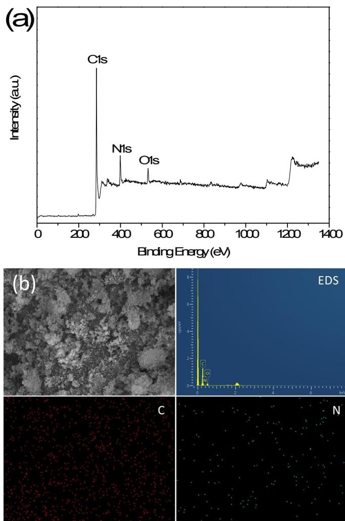
**Fig. S5.** (a) XPS survey spectra and (b) surface EDS analysis of CN-CF.
