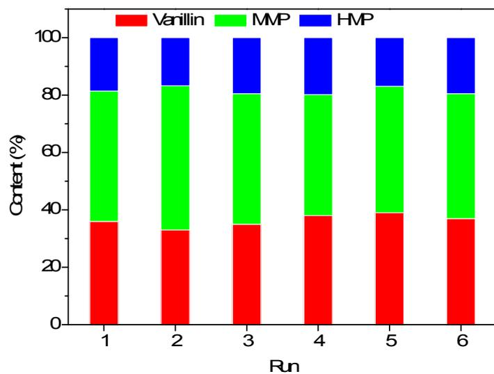
**Fig. S12.** Re-uses of Pd/CN-CF catalyst for the vanillin hydrogenation. Reaction conditions: vanillin (200 mg), catalyst (20 mg), H<sub>2</sub>O (16 mL), 1 MPa H<sub>2</sub>, 70 °C, 0.5 h.
