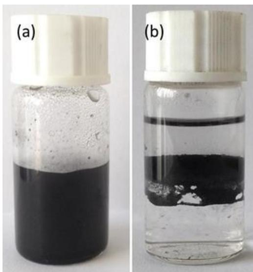
**Fig. S11.** Digital photos of catalyst and product separation. (a) The reaction mixture, (b) extracted by ethyl acetate. The Pd/CN-CF catalyst disperses in biphasic interface between ethyl acetate and water and can be easily recycled.
