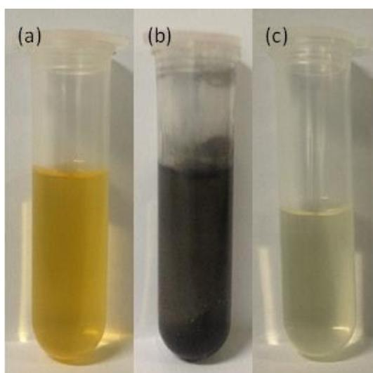
**Fig. S6.** The reaction solution for preparing Pd/CN-CF. (a) The PdCl<sub>2</sub> aqueous solution without CN-CF, (b) the PdCl<sub>2</sub> aqueous solution is added with CN-CF and stir at 40 °C for 1h, (c) the solution of (b) after removal of CN-CF by centrifugation.
