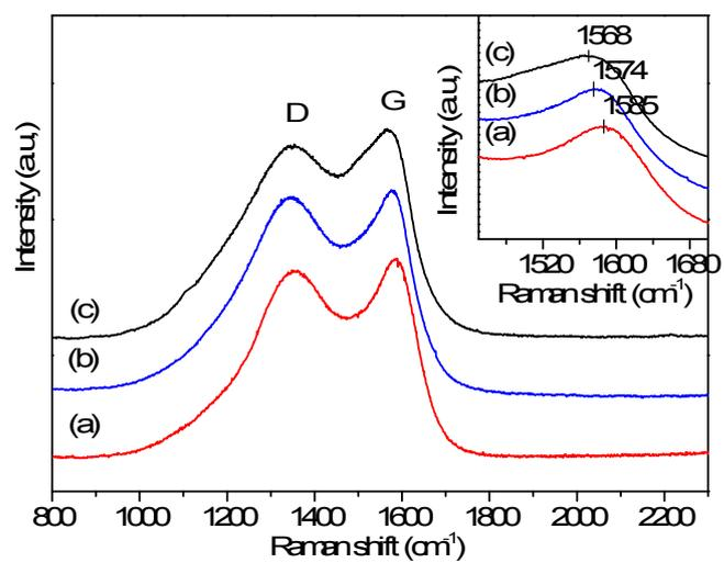
Fig. S2. Raman spectra of (a) CN-CT, (b) CN-TE and (c) CN-CF.
