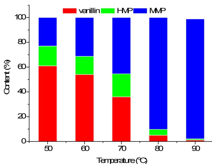
Fig. S8. Temperature-activity profile for the selective hydrogenation of vanillin.
