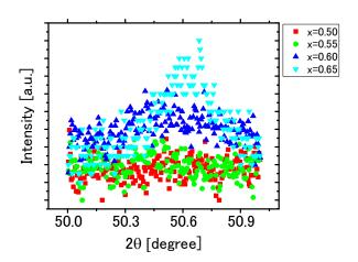
**Supplementary 1.** (A) XRD data for each x value; (B) extended XRD peaks around the phase change from Pm-3m to I4/mcm; (C) extended XRD peaks around the phase change from I4/mcm to Pnma
