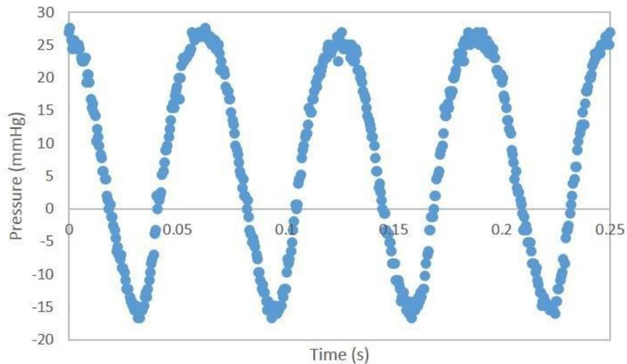
**Figure S2: Plot of pressure vs. time for flow through a regular PVC pipe at flow setting VI. The value of pressure shown here is relative to atmospheric pressure.**
