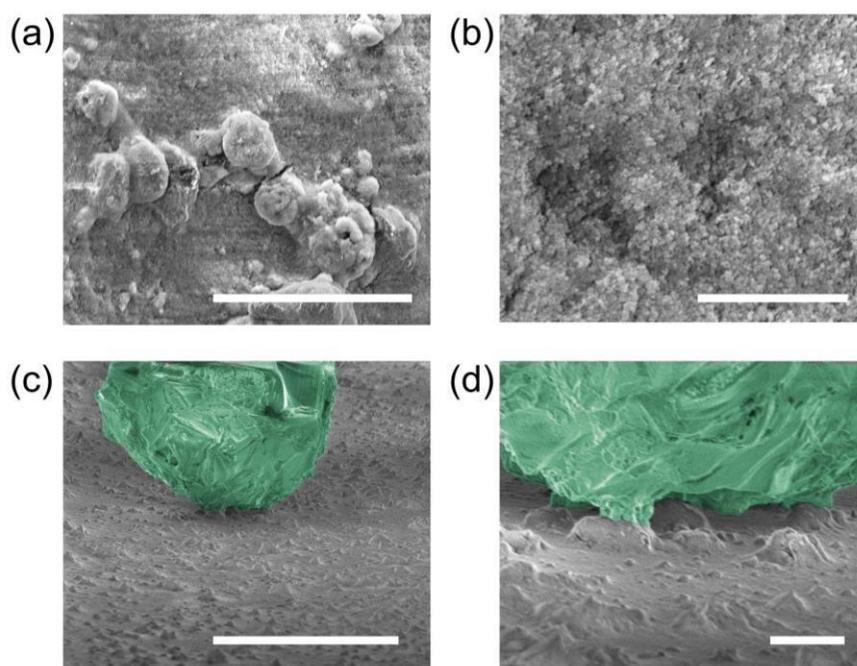
**Figure S1: SEM images of the top view of (a) micro-particles and (b) nano-particles of the liquid repellent coating. (c) Side view of a precipitate of NaCl (green) on the liquid repellent coating. (d) Magnified view of the base of the NaCl precipitate (green) that was suspended above the near-superhydrophobic surface by the micro-particles in the**
