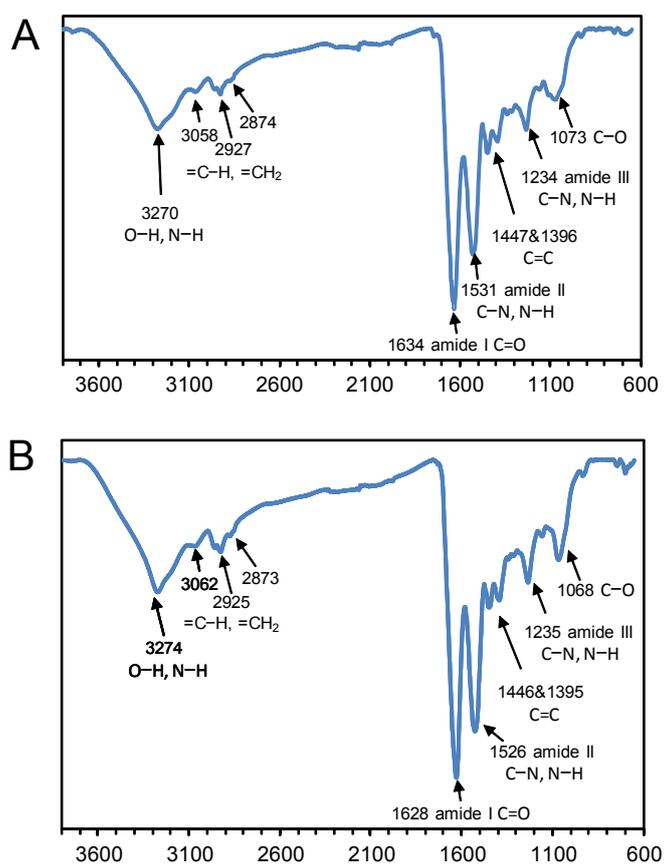
**Fig. S2.** The FT-IR spectra of ESM before and after operation.
