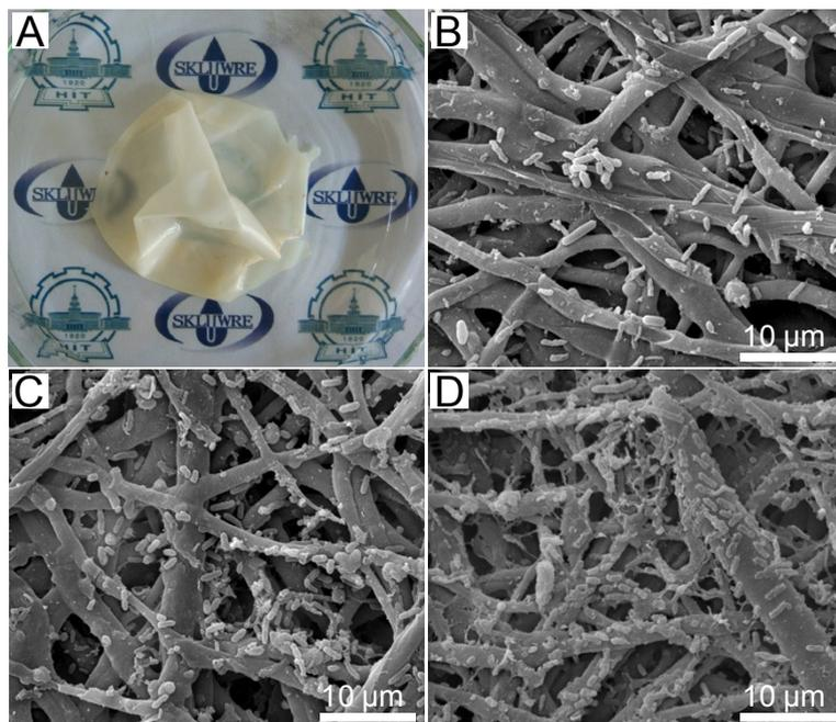
**Fig. S3.** (A)The optical image of EMS after 11 cycles' operation, and corresponding SEM images after the 4<sup>th</sup> cycle (B), 9<sup>th</sup> cycle (C), and 11<sup>th</sup> cycle (D).
