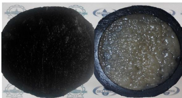
**Fig. S4.** Optical images of the air-cathode of MFC after long-term operation in the presence (left) and absence (right) of ESM.
