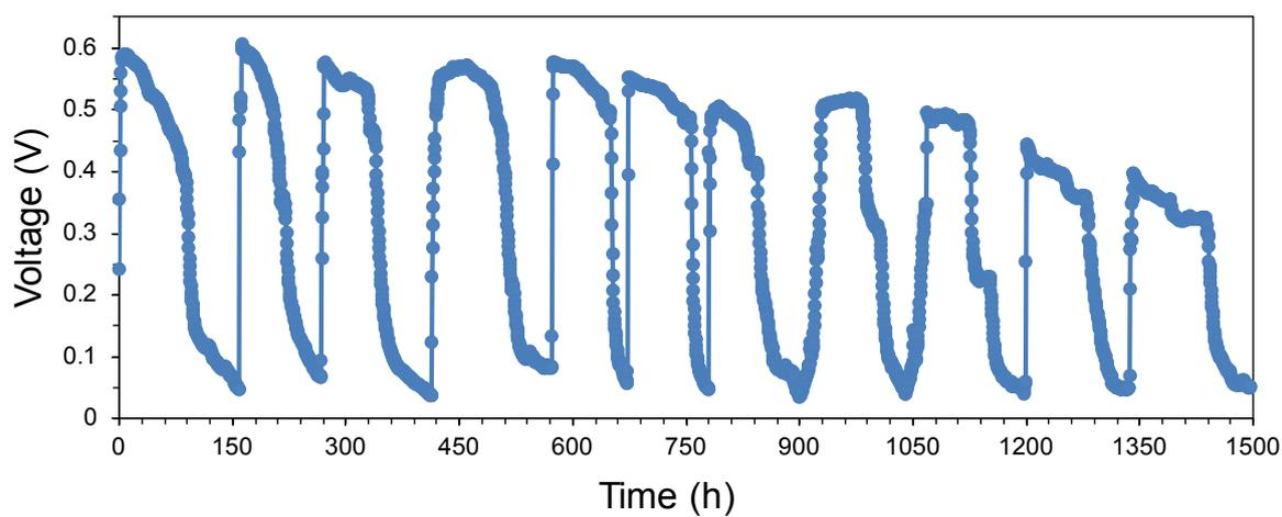
**Fig. S1.** Voltage output as operation continues for the cathode with ESM.
