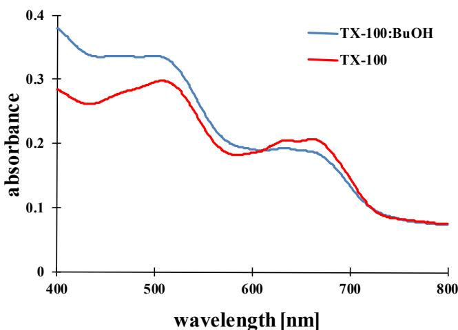
*Figure S5.* Comparison of the absorption spectra of systems with  $[BMIM][Tf_2N]$  with or without surfactant. In both cases, the ionic liquid mass fraction equals to 0.45.
