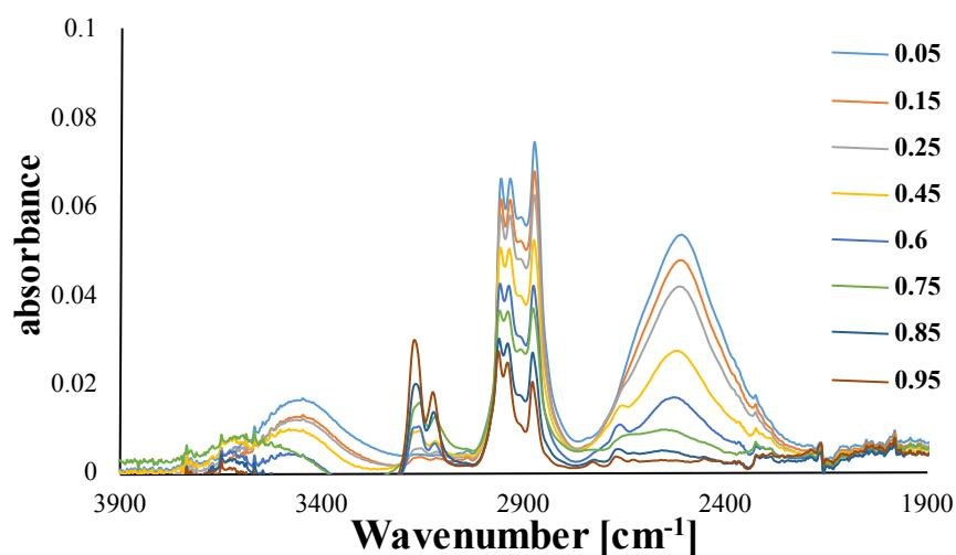
Figure S9. FTIR spectra of  $H_2O/(TX-100:BuOH)/[BMIM][PF_6]$  microemulsion at ionic liquid content 0.05; 0.15; 0.25; 0.45; 0.85; 0.95
