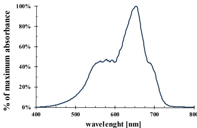
*Figure S6.* Normalized absorption spectrum of  $\text{CoCl}_2$  in butanol.
