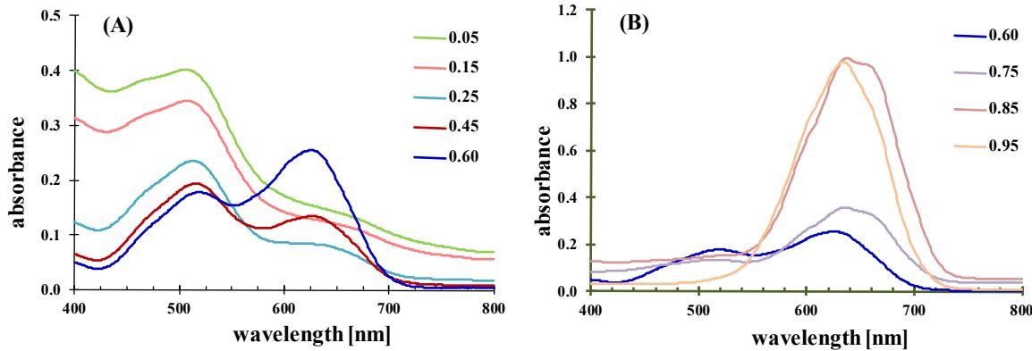
Figure S4. Dependences of absorbance of  $\text{CoCl}_2$  in the  $\text{H}_2\text{O}/\text{TX-100}:\text{BuOH}/[\text{BMIM}][\text{Tf}_2\text{N}]$  microemulsion on the IL mass fraction at the lower (A) and higher (B) IL contents determined for L85 line ( $\text{TX-100}/\text{H}_2\text{O} = 0.85/0.15$ ).
