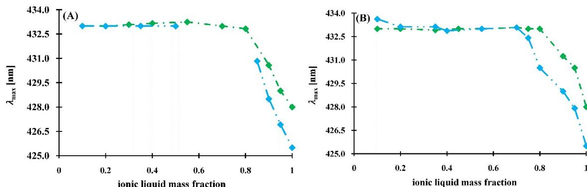
*Figure S7.* The dependences of maximum absorption wavelength of methyl orange dissolved in the microemulsions on ionic liquid content determined for L85 dilution lines, (A) represents  $[BMIM][PF_6]$
