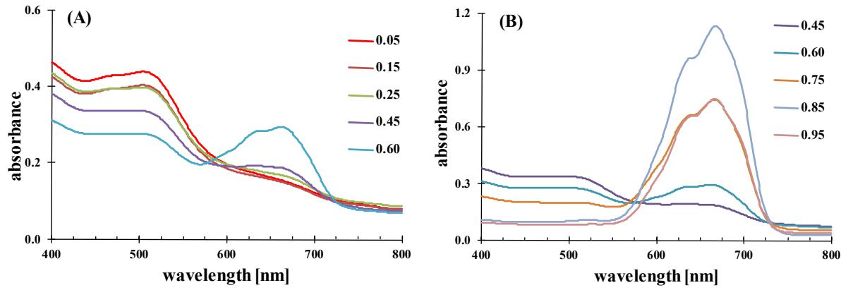
Figure S3. Dependences of absorbance of  $\text{CoCl}_2$  in the  $\text{H}_2\text{O}/(\text{TX-100}:\text{BuOH})/[\text{BMIM}][\text{PF}_6]$  microemulsion on the IL mass fraction at the lower (A) and higher (B) IL contents determined for L85 line ( $\text{TX-100}/\text{H}_2\text{O} = 0.85/0.15$ ).
