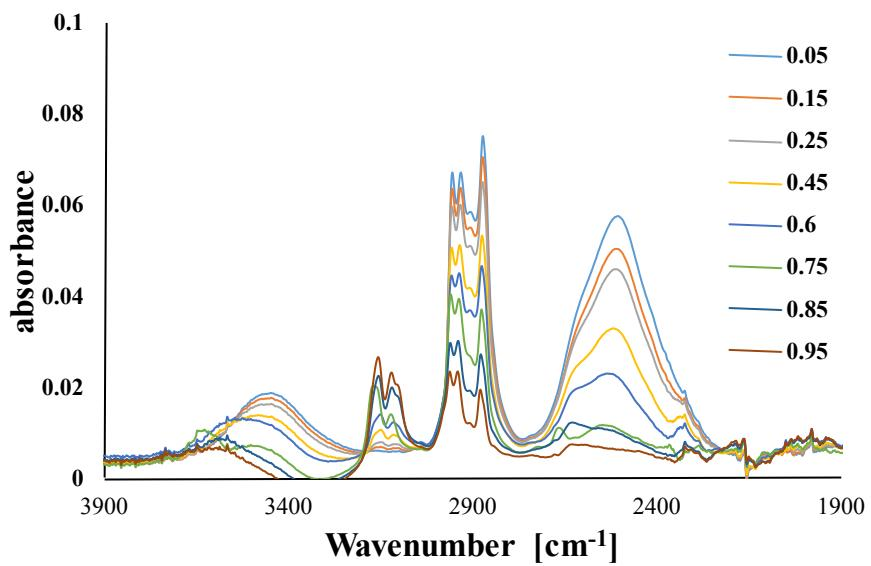
Figure S10. FTIR spectra of  $H_2O/(TX-100:BuOH)/[BMIM][Tf_2N]$  microemulsion at ionic liquid content 0.05; 0.15; 0.25; 0.45; 0.6; 0.75; 0.85; 0.95
