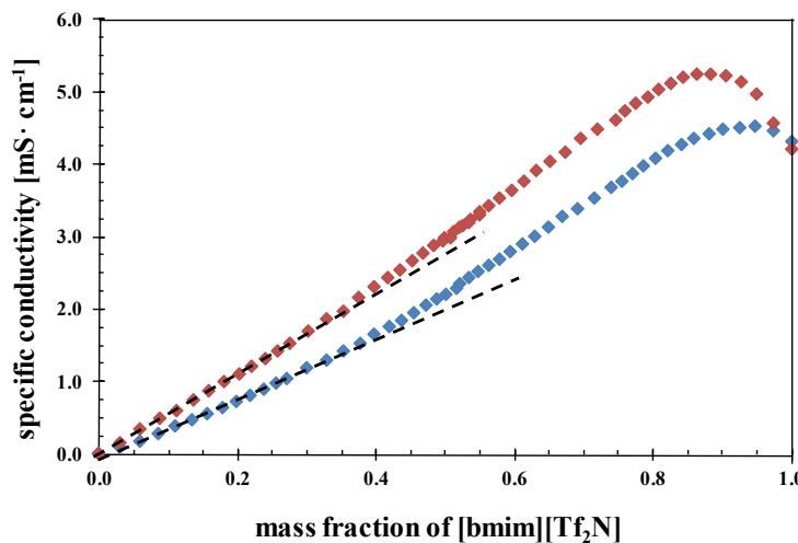
Figure S1. Specific conductivity of [BMIM][Tf<sub>2</sub>N]/(TX-100:BuOH)/H<sub>2</sub>O system in a function of IL content for (◆) 0.15:0.85 and (◆) 0.05:0.95 water-to-mixed surfactant mass ratio.
