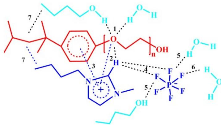
Figure S2. Selected interactions between components of [BMIM][PF<sub>6</sub>]/(TX-100:BuOH)/H<sub>2</sub>O microemulsion
