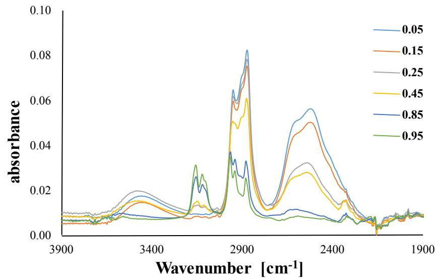
Figure S8. FTIR spectra of  $H_2O/TX-100/[BMIM][Tf_2N]$  microemulsion at ionic liquid content 0.05; 0.15; 0.25; 0.45; 0.85; 0.95
