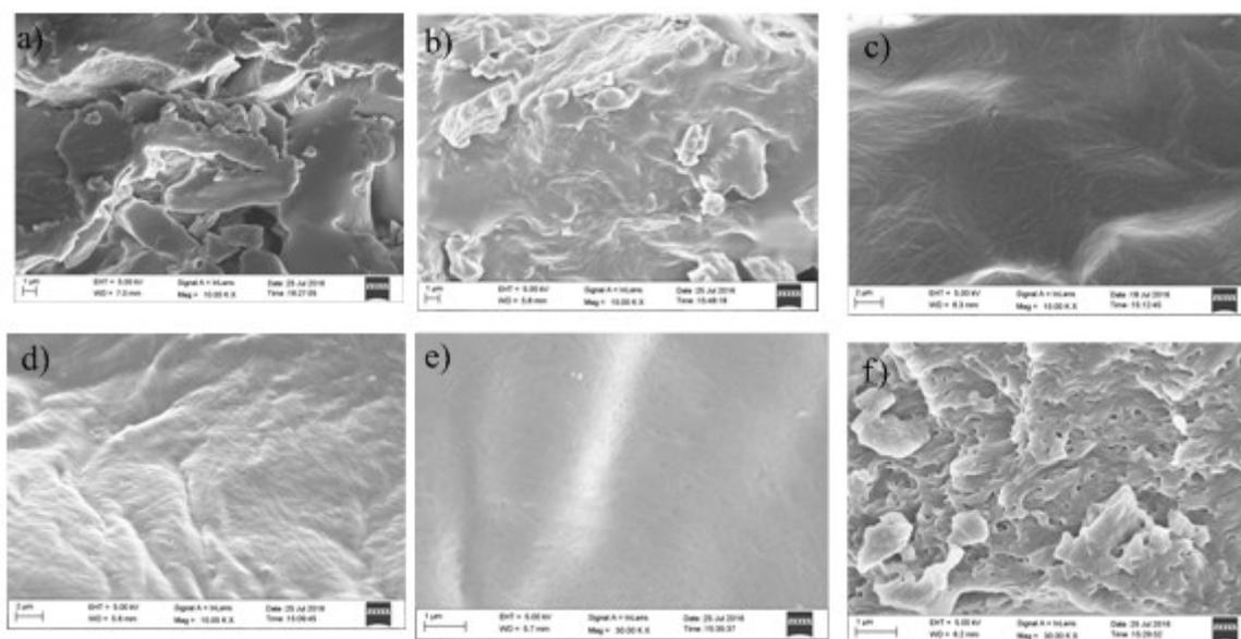
**Figure S1** SEM images of the xerogels of **9a** a) Cyclohexane b) Hexane c) Benzene d) *tert*-butyl benzene e) Mesitylene. f) SEM image of gel of **9e** Dodecane
