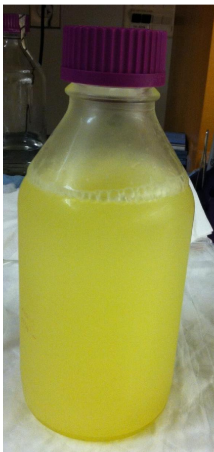
Fig. S12 Digital image of a 1 litre culture of CdS precipitating bacteria, showing the typical yellow color associated with CdS in the culture.
