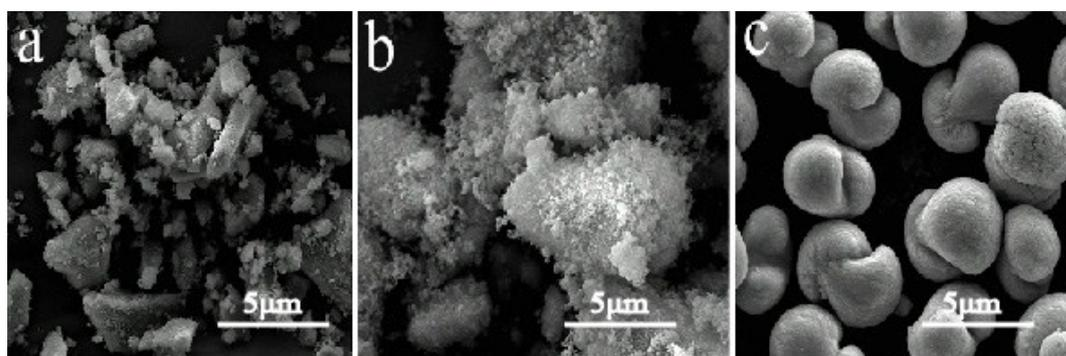
Fig. S8 SEM images of samples with diethylene glycol (a), 1,2-propylene glycol (b), isopropanol (c) as solvent
