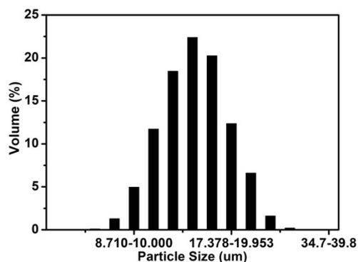
Fig. S3 Particle size distribution of LiFePO<sub>4</sub> microsphere.
