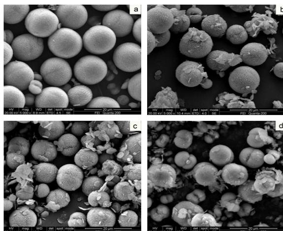
Fig. S6 SEM images of samples prepared with glycol solvent containing different content of deionized water (a) 0%; (b) 3%; (c) 5%; (d), 10%
