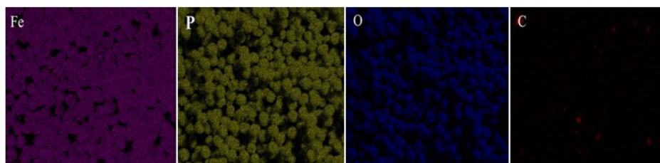
Fig. S2 EDS analysis of the  $\text{LiFePO}_4$  microsphere
