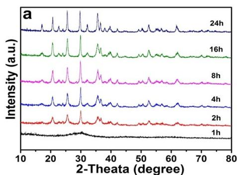
Fig. S4 XRD patterns of the LiFePO<sub>4</sub> microsphere prepared at different solvothermal time
