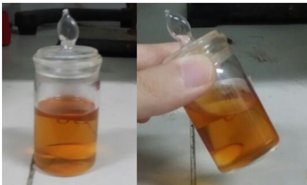
Figure S4. Images of the de-forming products of C5 after heating and cooling down process dissolving in Toluene.
