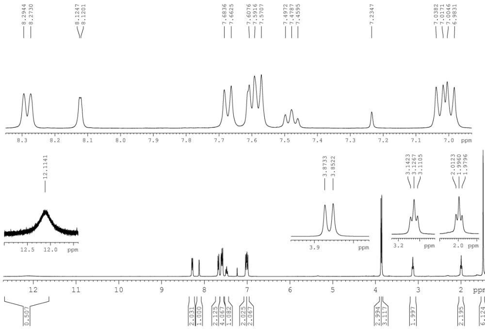
**Figure S36.** <sup>1</sup>H NMR spectrum of P4 at 400 MHz in CDCl<sub>3</sub> (303 K). Lorentz-Gauss transformation (lb = -0.4, gb = 40 %).
