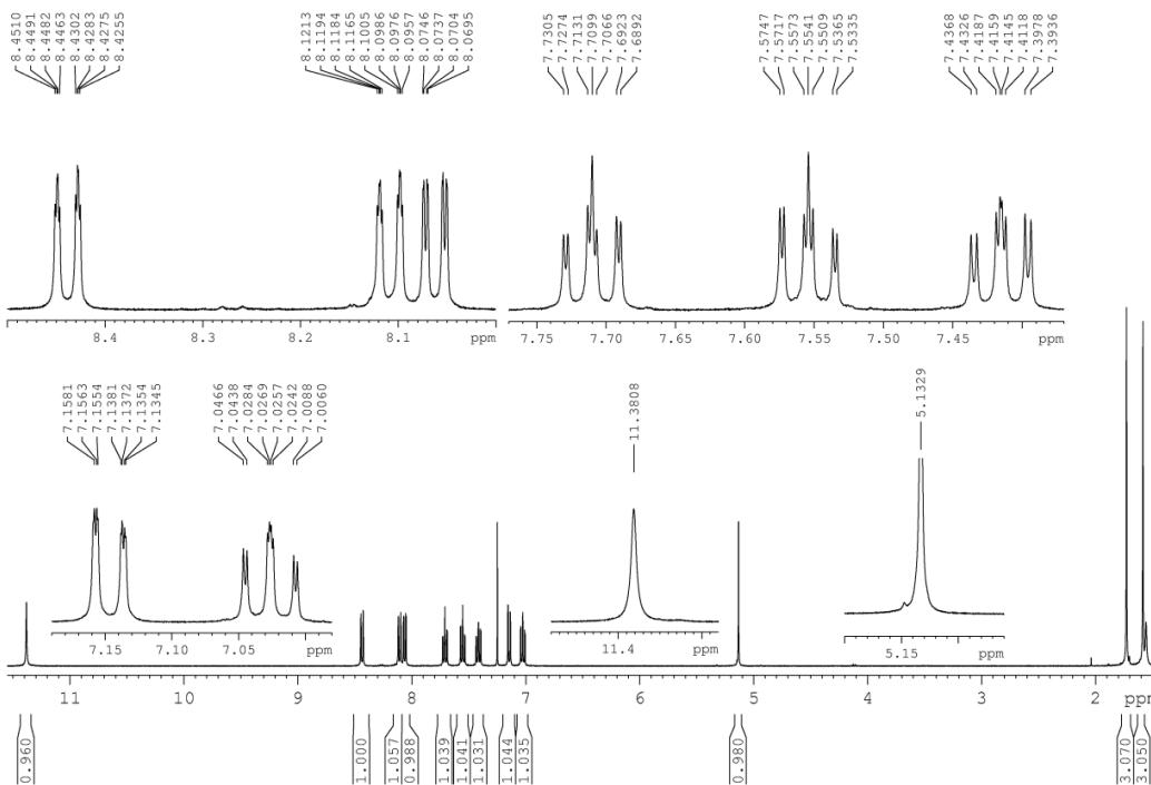
**Figure S10.**  $^1\text{H}$  NMR spectrum of **P1** at 400 MHz in  $\text{CDCl}_3$  (303 K). Lorentz-Gauss transformation ( $\text{lb} = -0.3$ ,  $\text{gb} = 40\%$ ).
