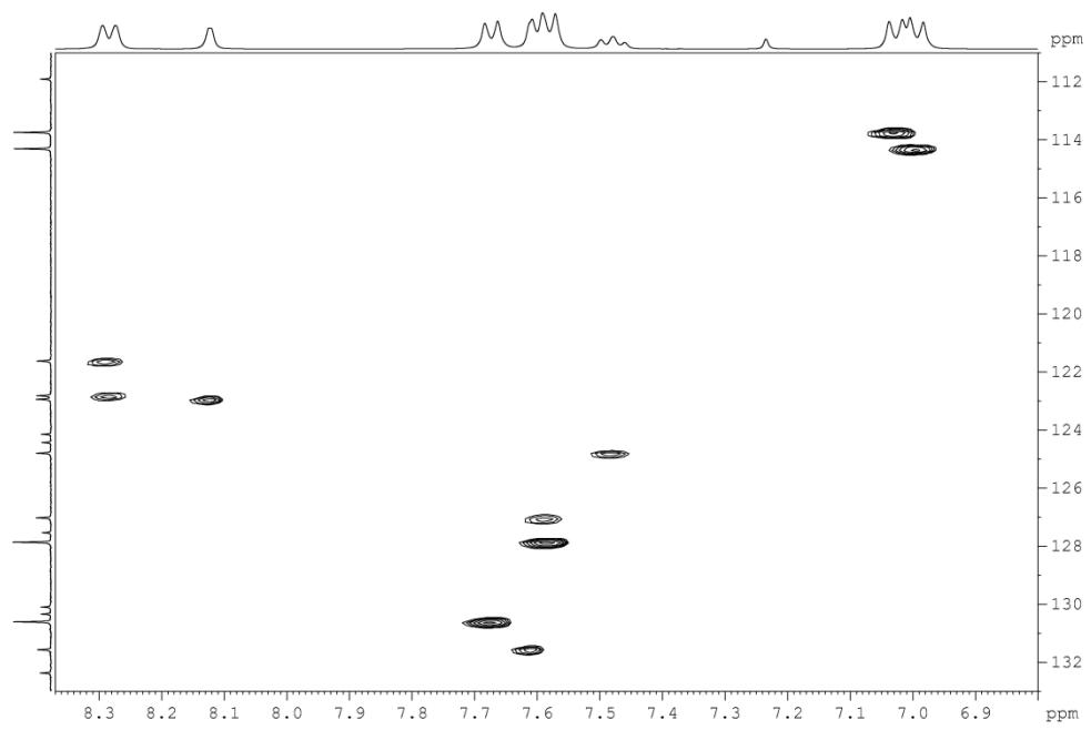
**Figure S43.** Expanded  $^1\text{H}$ - $^{13}\text{C}$  HSQC spectrum of **P4** at 400 MHz in  $\text{CDCl}_3$  (303 K). Correlations in black represent peaks with positive phase ( $\text{CH}_3$  and  $\text{CH}$  correlations) whereas the correlation in red indicates negative intensities ( $\text{CH}_2$  correlations).
