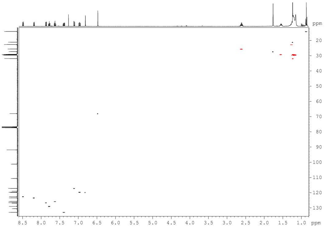
**Figure S24.**  $^1\text{H}$ - $^{13}\text{C}$  HSQC spectrum of **P2** at 400 MHz in  $\text{CDCl}_3$  (303 K). Correlations in black represent peaks with positive phase ( $\text{CH}_3$  and  $\text{CH}$  correlations) whereas the correlation in red indicates negative intensities ( $\text{CH}_2$  correlations).
