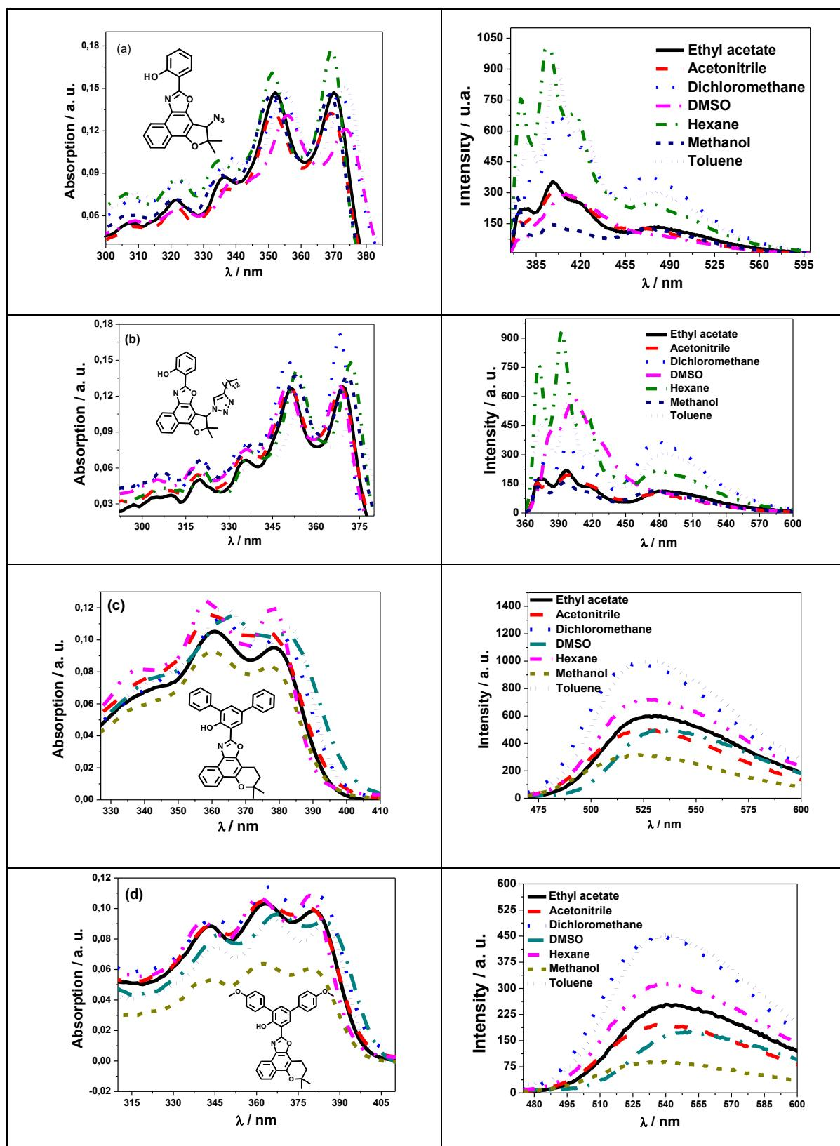
**Figure S53.** UV-Vis spectra (left) and emission spectra (right) of (a) **P1**, (b) **P2**, (c) **P3** and (d) **P4** in different solvents.
