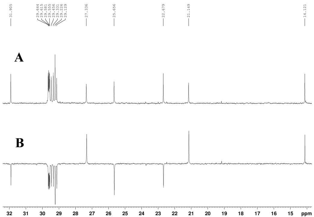
**Figure S21.** Expanded (A)  $^{13}\text{C}$  NMR and (B) DEPT-135 spectra of **P2** at 100 MHz in  $\text{CDCl}_3$  (303 K).
