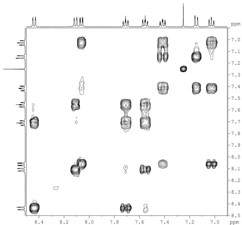
**Figure S14.** Expanded COSY spectrum of **P1** at 400 MHz in  $\text{CDCl}_3$  (303 K) showing the correlations between aromatic <sup>1</sup>H resonances.
