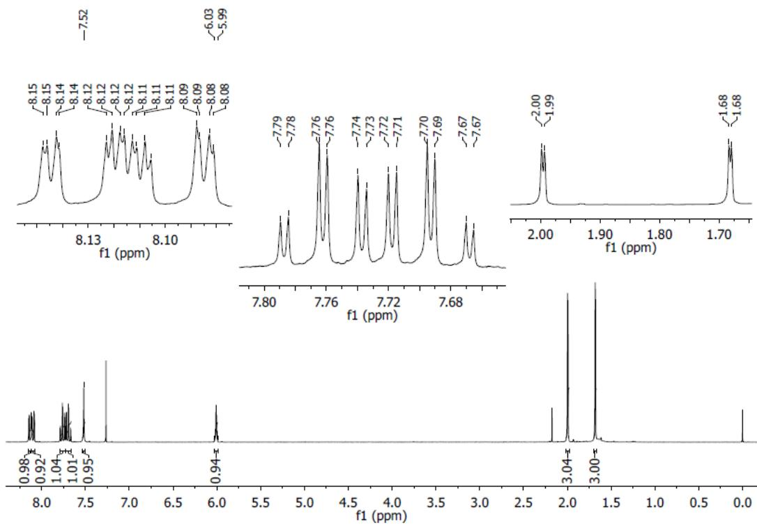
**Figure S1.** <sup>1</sup>H NMR spectrum of compound 2 at 400 MHz in CDCl<sub>3</sub> (303 K).
