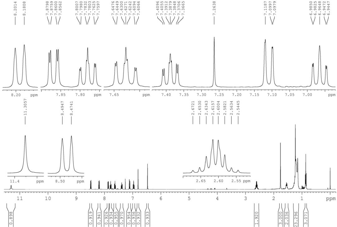
**Figure S17.**  $^1\text{H}$ NMR spectrum of **P2** at 400 MHz in  $\text{CDCl}_3$  (303 K).
