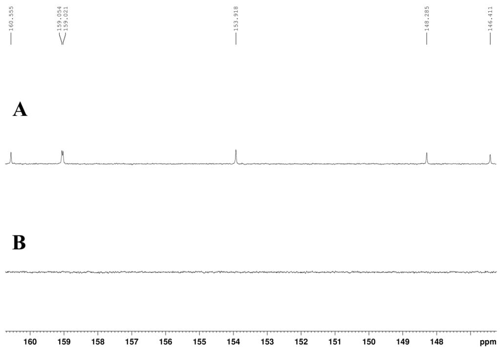
**Figure S39.** Expanded (A)  $^{13}\text{C}$  NMR and (B) DEPT-135 spectra of **P4** at 100 MHz in  $\text{CDCl}_3$  (303 K).
