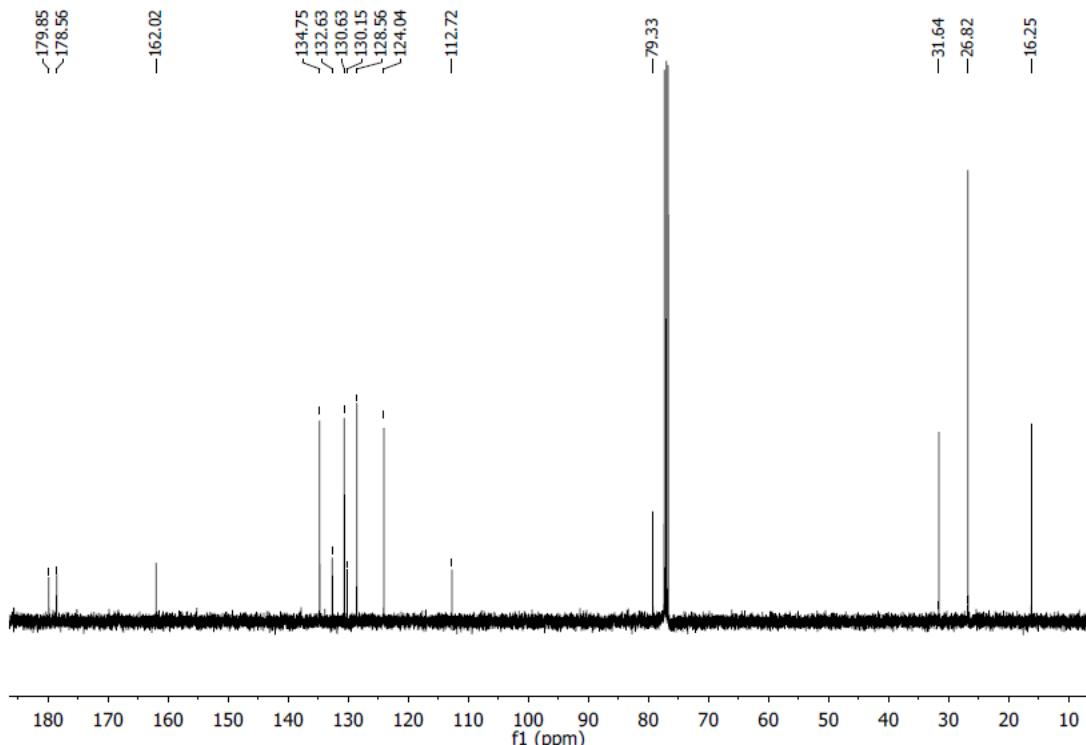
**Figure S6.**  $^{13}\text{C}$  NMR spectrum of compound 4 at 100 MHz in  $\text{CDCl}_3$  (303 K).
