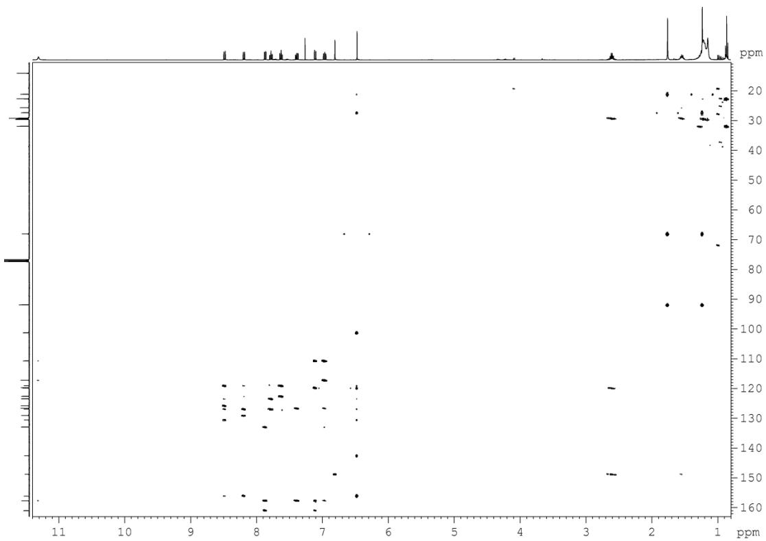
**Figure S25.** <sup>1</sup>H-<sup>13</sup>C HMBC spectrum of **P2** at 400 MHz in CDCl<sub>3</sub> (303 K).
