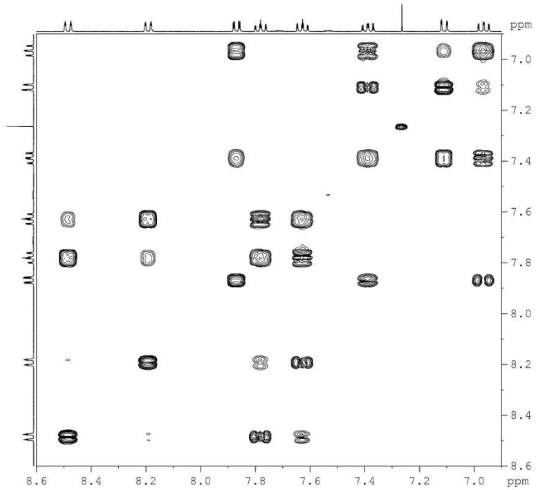
**Figure S23.** Expanded COSY spectrum of **P2** at 400 MHz in  $\text{CDCl}_3$  (303 K) showing the correlations between aromatic  $^1\text{H}$  resonances.
