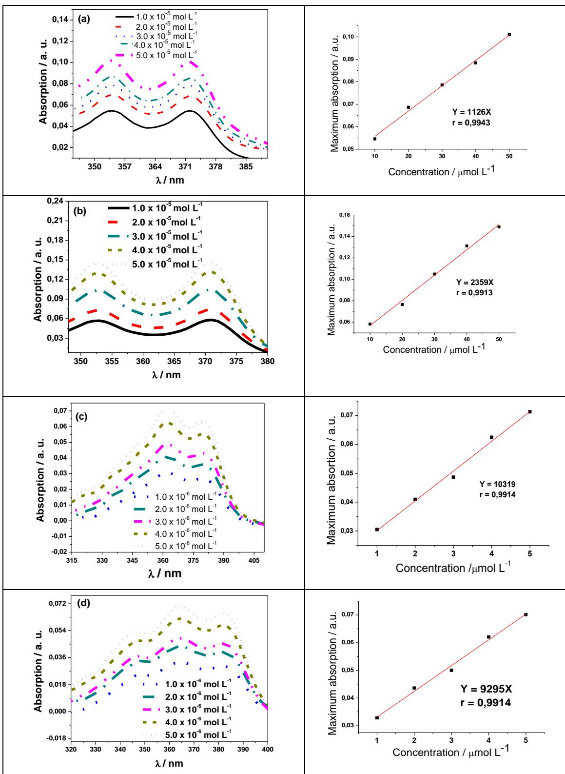
**Figure S54.** UV-Vis spectra (left) and calibration curve (right) for (a) **P1**, (b) **P2**, (c) **P3** and (d) **P4**.
