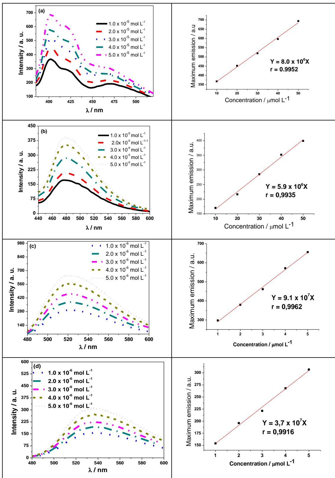
**Figure S55.** Emission spectra (left) and calibration curve (right) obtained for (a) **P1**, (b) **P2**, (c) **P3** and (d) **P4**.
