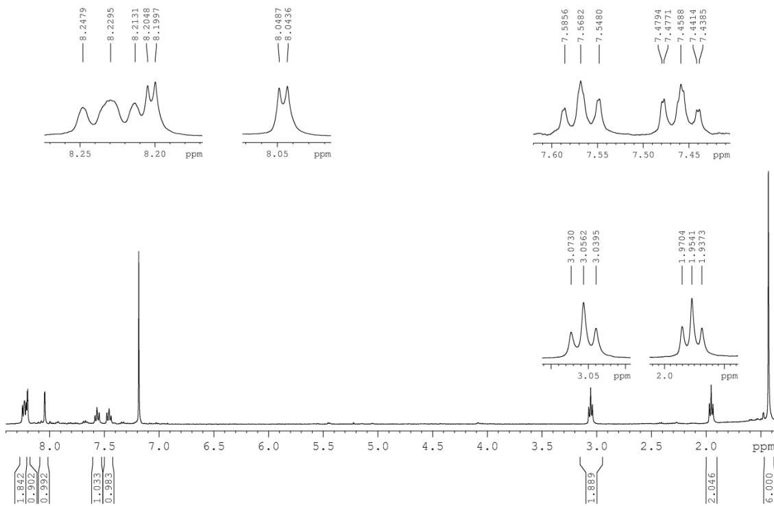
**Figure S7.**  $^1\text{H}$  NMR spectrum of compound **5** at 400 MHz in  $\text{CDCl}_3$  (303 K).
