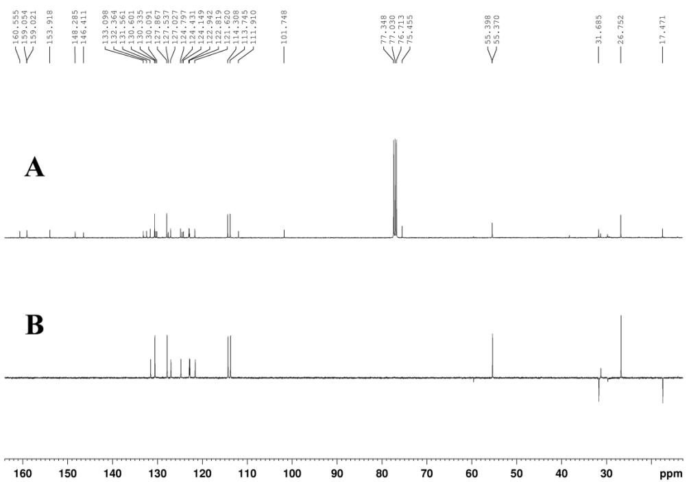
**Figure S37.** (A) <sup>13</sup>C NMR and (B) DEPT-135 spectra of **P4** at 100 MHz in CDCl<sub>3</sub> (303 K).
