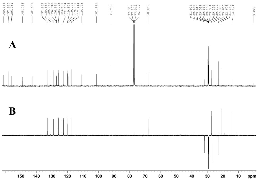
**Figure S19.** (A) <sup>13</sup>C NMR and (B) DEPT-135 spectra of **P2** at 100 MHz in CDCl<sub>3</sub> (303 K).
