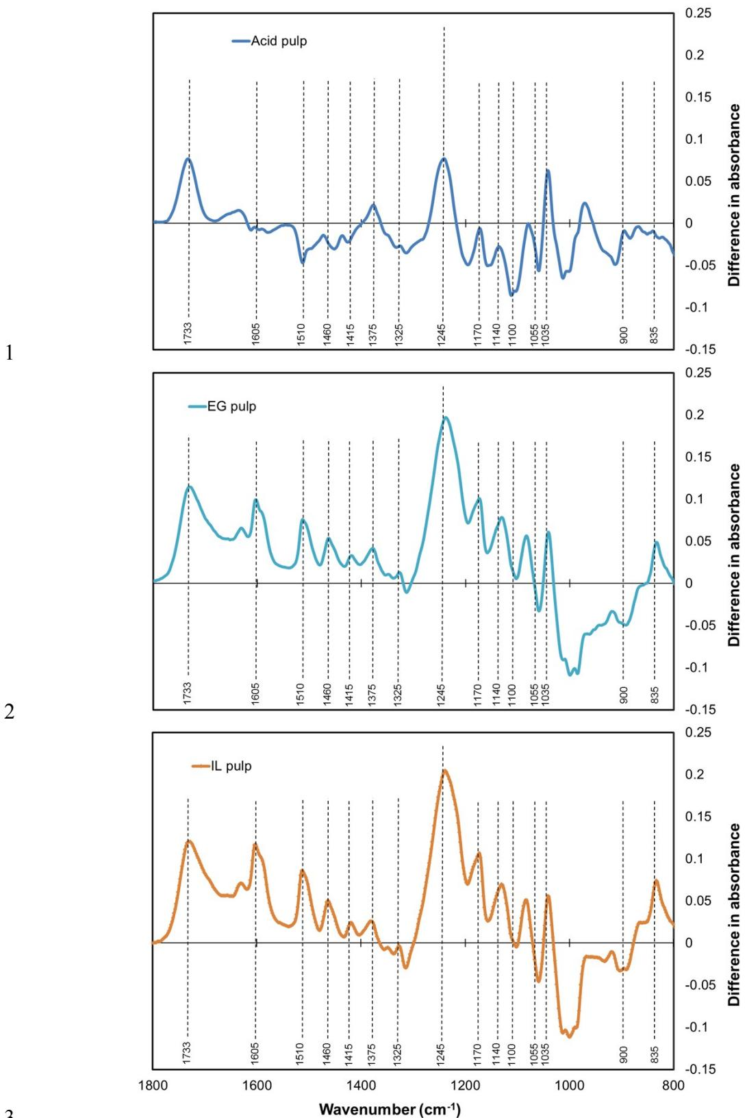
4 Fig. S2. FTIR difference spectra (compared to bagasse) of the pulp (fiber) after acid
