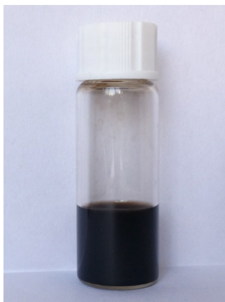
Fig. S3 The photograph of SCX6-MnO 2 @RGO aqueous dispersion (1.0 mg mL -1 ) after being stored for 6 months.
