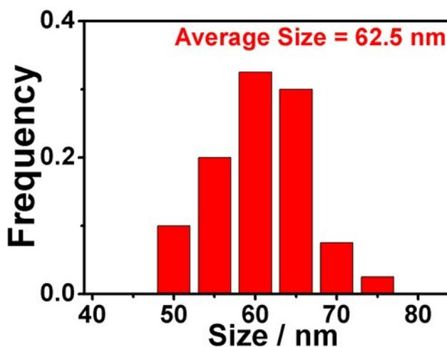
Figure S1. The size distribution histogram of Au nanoparticles measured on 250 particles from the SEM image of CoS<sub>2</sub>/Au sample.
