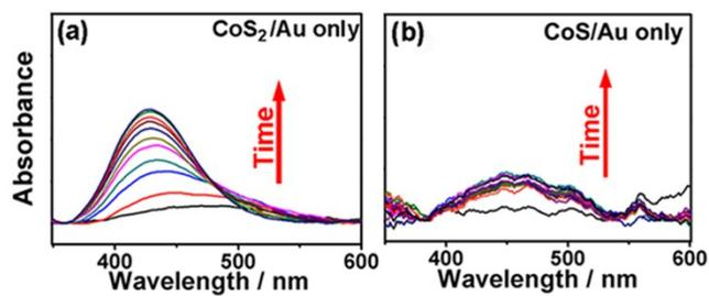
Figure S4. The UV-vis spectra of the catalytic oxidation process of OPD molecules without the addition of  $\text{H}_2\text{O}_2$ : (a) only  $\text{CoS}_2/\text{Au}$  and (b) only  $\text{CoS}/\text{Au}$  composite was added.
