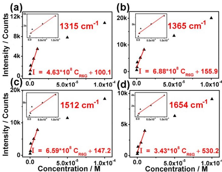
Figure S7. The work curves of Raman peak intensity and concentration of R6G at (a)  $1315 \text{ cm}^{-1}$ , (b)  $1365 \text{ cm}^{-1}$ , (c)  $1512 \text{ cm}^{-1}$ , and (d)  $1654 \text{ cm}^{-1}$  by employing  $\text{CoS}_2/\text{Au}$  as the substrate.
