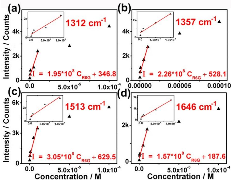
Figure S8. The work curves of Raman peak intensity and concentration of R6G at (a) 1312  $\text{cm}^{-1}$ , (b) 1357  $\text{cm}^{-1}$ , (c) 1513  $\text{cm}^{-1}$ , and (d) 1646  $\text{cm}^{-1}$  employing CoS/Au as the substrate.
