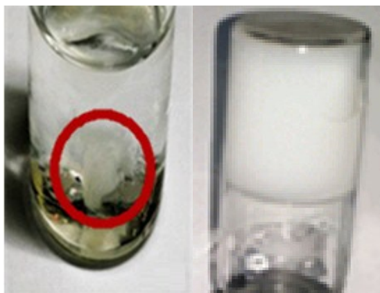
Fig. S6. The photograph of 75% and 100% [EMIM]BF 4 / PVA/H 3 PO 4 gel polymer electrolyte, highlighting the formation of curdy white precipitate. The dried composition of these electrolytes show completely opaque thin films.
