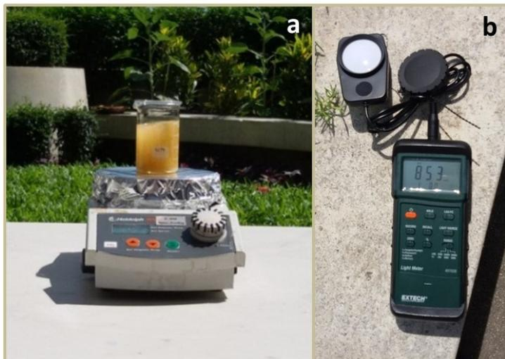
**Figure S11** (a) Photodeposition activity under natural sunlight and (b) sunlight intensity measurement by Lux meter.
